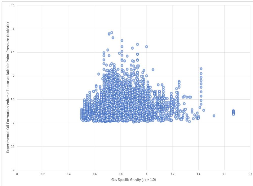
Figure A-7—Cross plot of the gas specific gravity against the experimental oil formation volume factor at bubble point pressure for the worldwide dataset.
