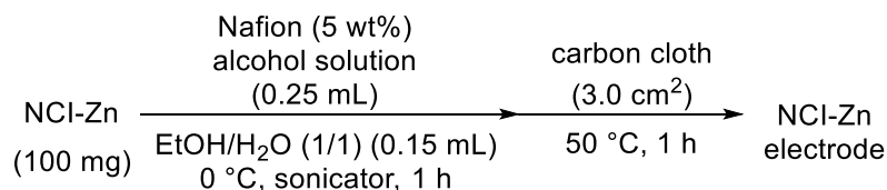
Scheme 30. Preparation of NCI-Zn electrode
