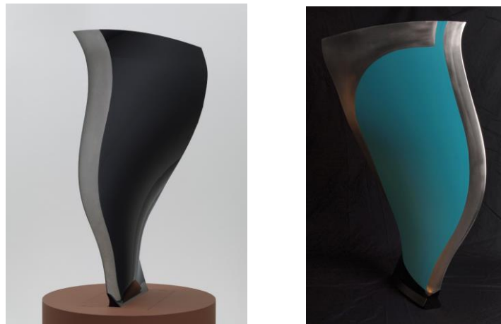
Fig. 1.1 GE composite fan blade [1] (left) and Rolls Royce composite fan blade [2] (right)
