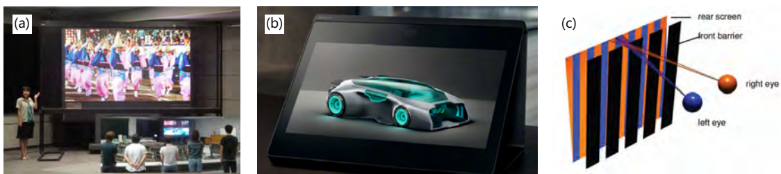
Fig. 2.8. Several examples for aerial displays; (a) Distant aerial image presentation using parallax barrier [147]. (b) Stereoscopic display using fly-eye lens [11]. (c) Dynamic parallax barrier named "Dynallax" [148].
