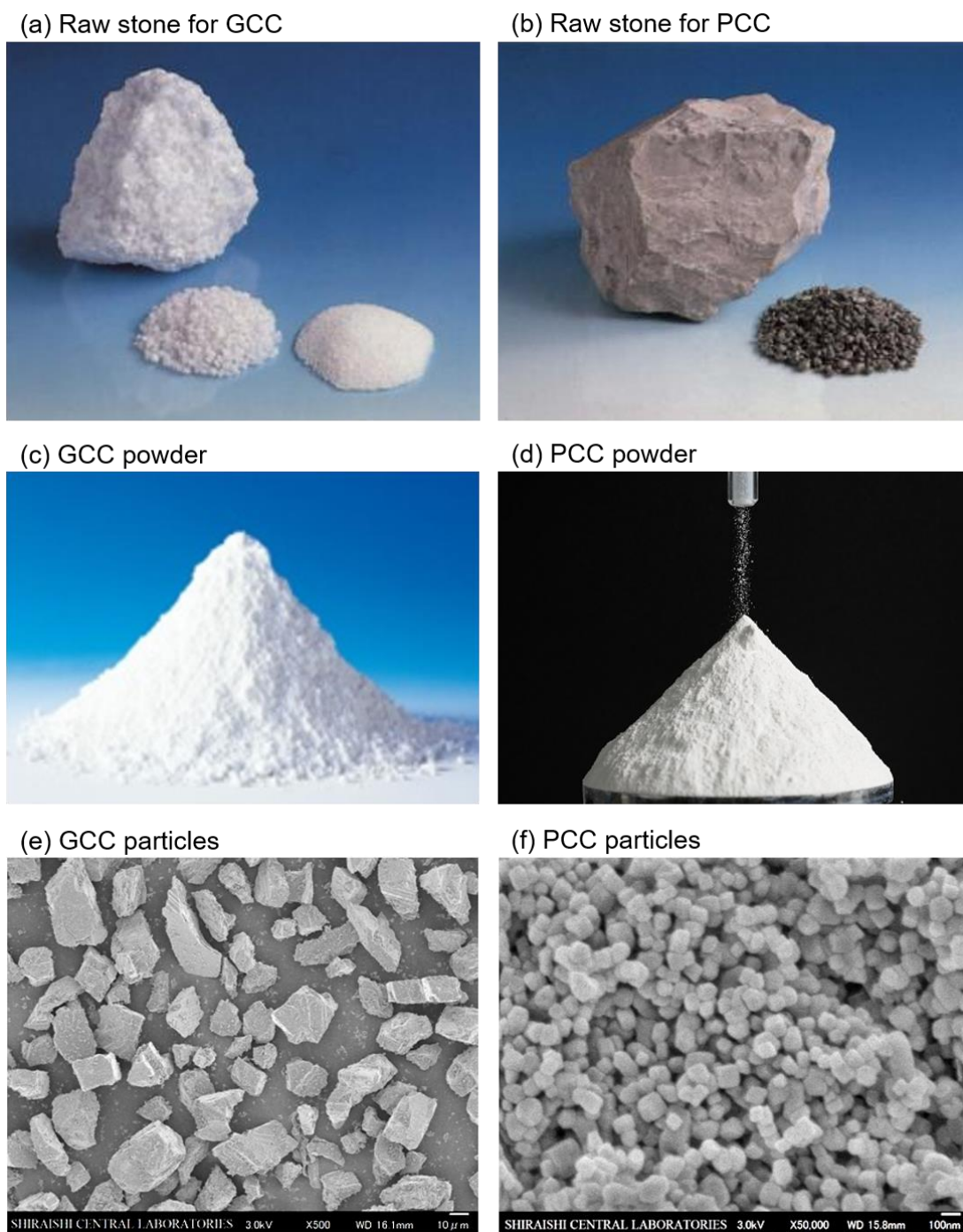
Fig. 1-4. Pictures of raw stones for (a) ground calcium carbonate (GCC) and (b) precipitated calcium carbonate (PCC). Pictures of (c) GCC and (d) PCC in the forms of powders. SEM images of (e) GCC irregular-shaped particles (magnification: \times 500 , scale bar: 10\ \mu\text{m} ) and (f) PCC rhombohedral nanoparticles (magnification: \times 50,000 , scale bar: 100\ \text{nm} ).
