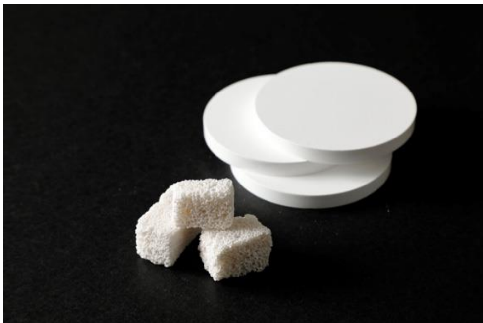
Fig. 1-6. Picture of dense and porous calcite ceramics.
