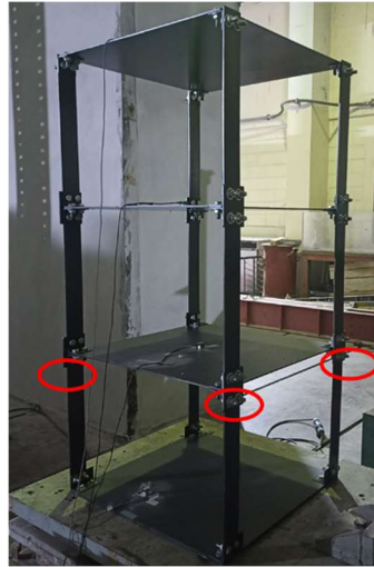
Case 2: Damaged first floor
