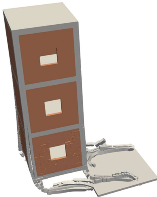
Figure 5-25 : Damage JMA 6.5
