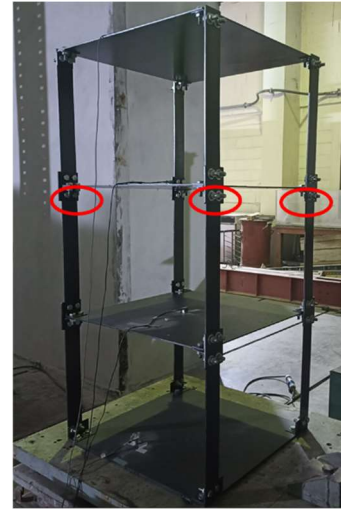
Case 3: Damaged second floor
