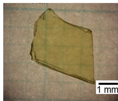
Fig. 3.15 \text{RbFe}(\text{MoO}_4)_2 single crystal obtained by the flux method.
