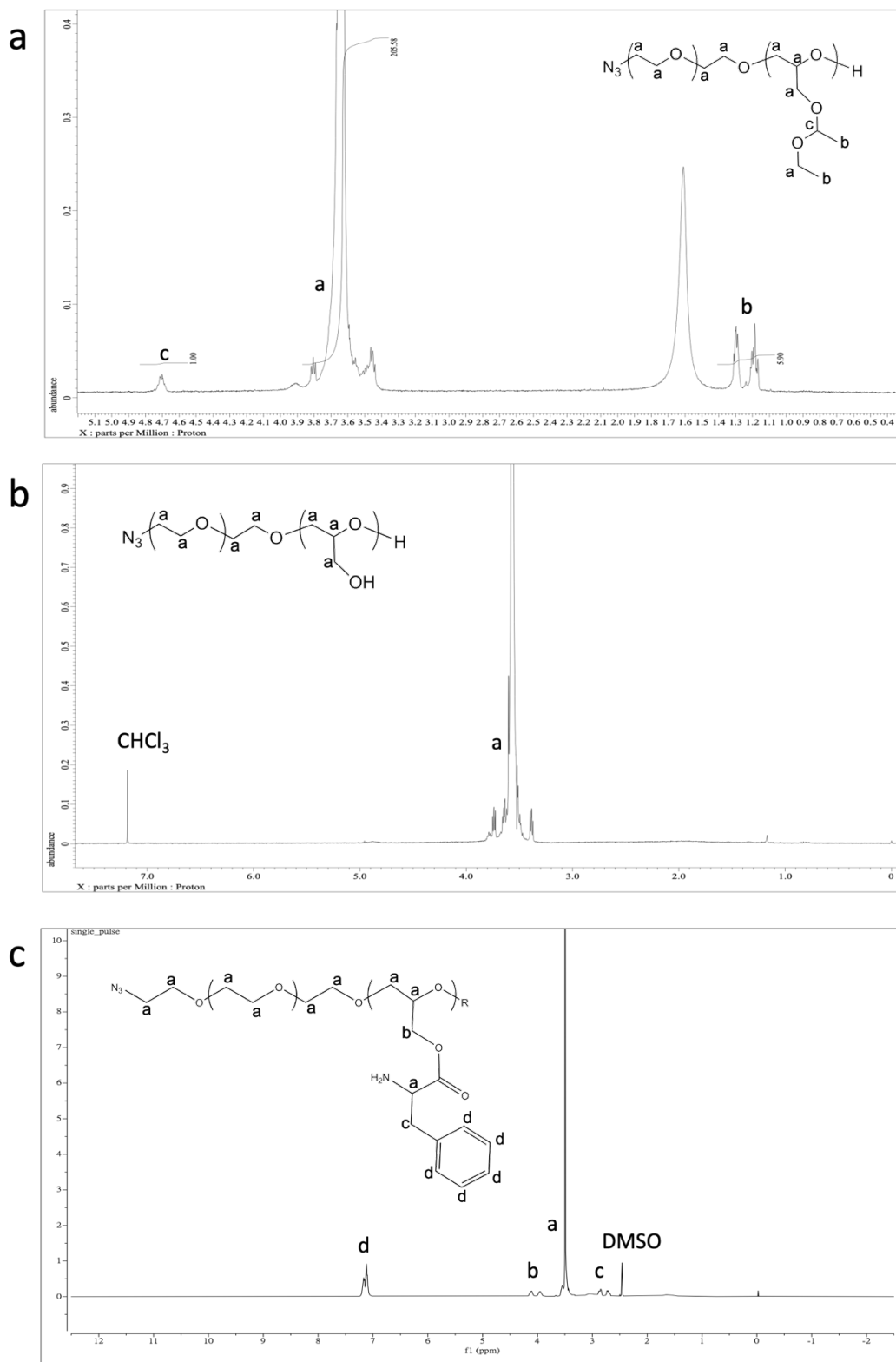
Figure 3.2 ^1\text{H-NMR} spectra of polymers. a) ^1\text{H-NMR} spectrum of PEG-PEEGE. 89 units of EEGE were added. b) ^1\text{H-NMR} spectrum of PEG-PG. Deprotection was confirmed c) ^1\text{H-NMR} spectrum of PEG-PG(Phe). The conjugation rate of Phe was calculated to be around 89%.
