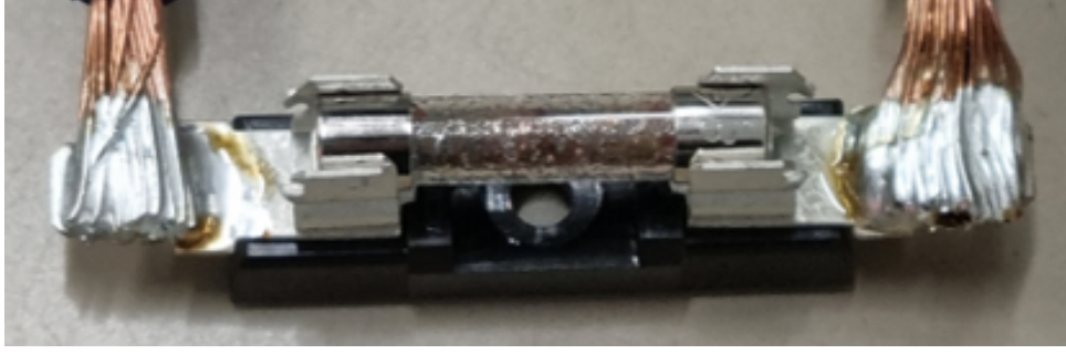
Figure 2.19: Post-commutation condition of the glass fuse
