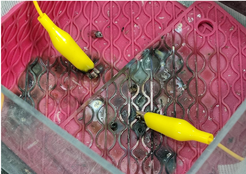
Figure 2.11: Post-test condition of the glass fuse
