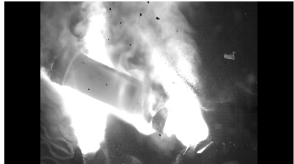
(b) Fuse explosion under late commutation
