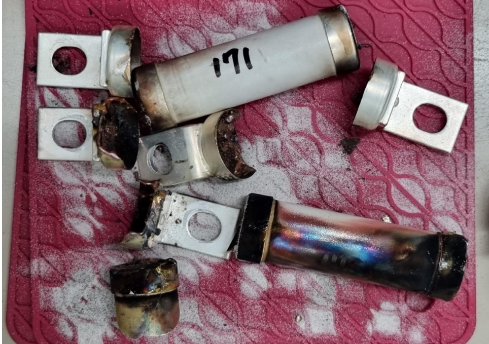
Figure 2.8: Post-test condition of the ceramic fuse
