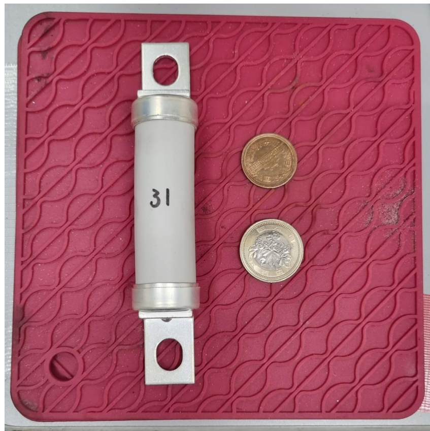
Figure 3.9: Ceramic fuse tested in the experiment
