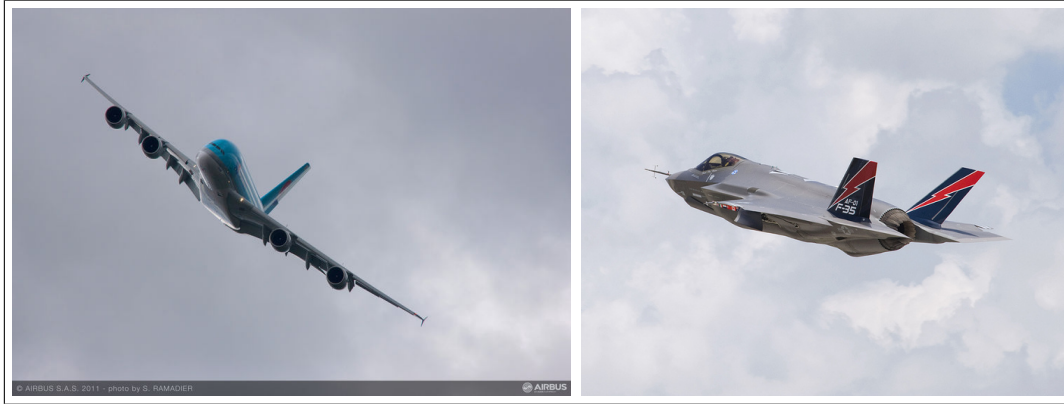
Figure 4.10: Modern engineering designs: an open-loop stable passenger airliner A380 on the left, and an unstable jet fighter F35 on the right [34][35].
