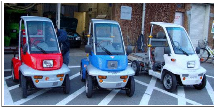
Figure 3.6: IWM-driven EV COMS of Hori Laboratory: COMS3, COMS1, and COMS2 from the left.
