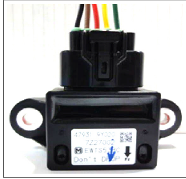
Figure 4.7: Acceleration sensor unit used in the system. Yaw rate, x-directional, and y-directional accelerations can be measured.
