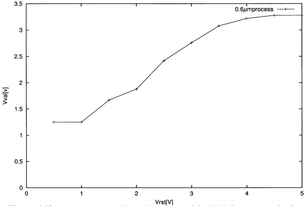
**Figure 4.12** Relation between  $V_{rst}$  and  $V_{val}$  (case of CMOS  $0.6\mu$  process technology)
