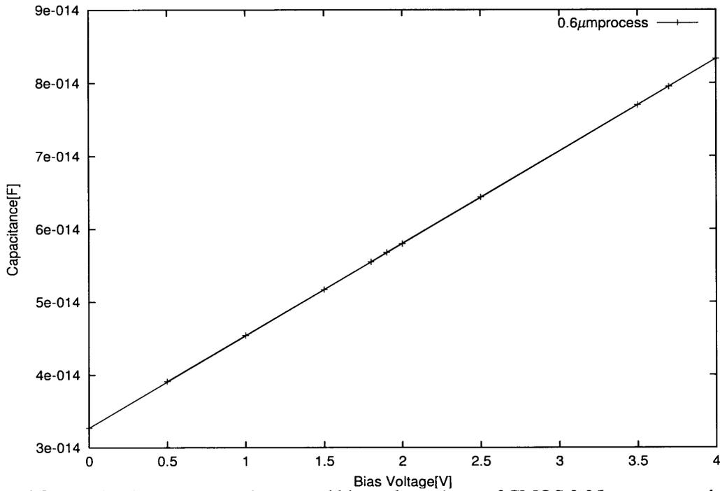
**Figure 4.8** Relation between capacitance and bias voltage (case of CMOS 0.35 μm process technology)
