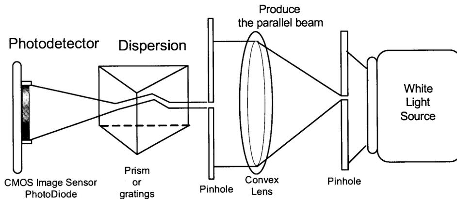
**Figure 4.2** Optical system(in the case of a prism)
