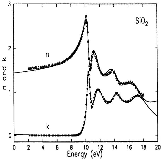
**Figure 6.1** Infractive index and Extinction coefficient( $\text{SiO}_2$ )
