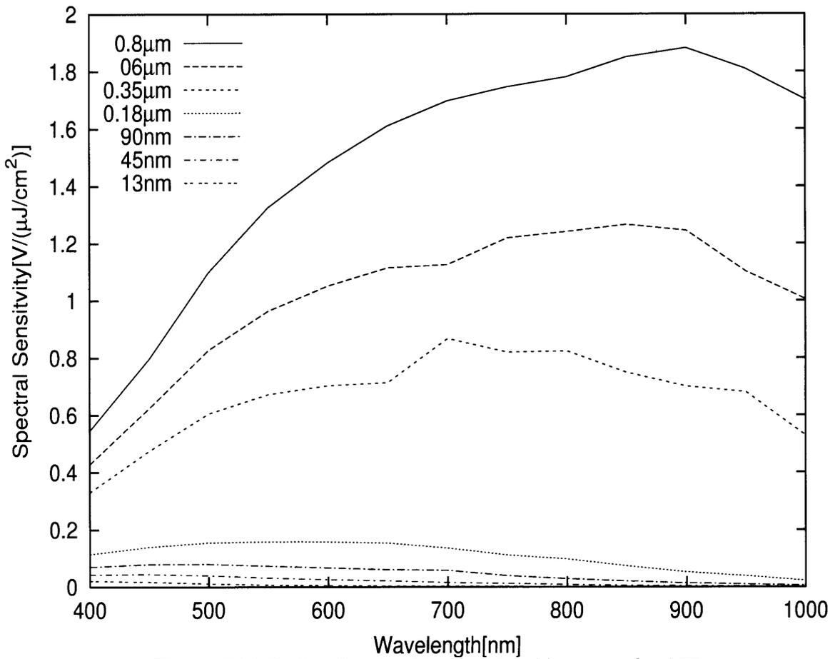
**Figure 5.16** Scaling Trends of Spectral Sensitivity with fixed FF
