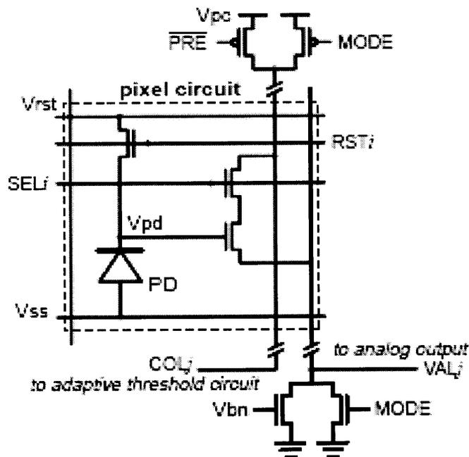
Figure 4.1 Readout Circuit Configuration
