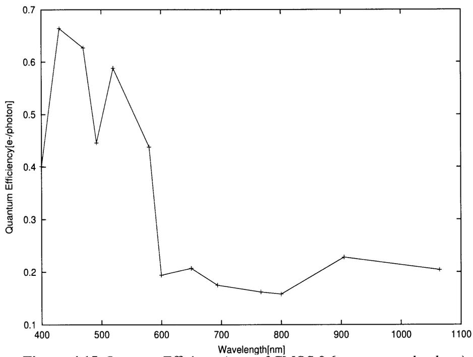
**Figure 4.15** Quantum Efficiency(case of CMOS 0.6 $\mu$  process technology)
