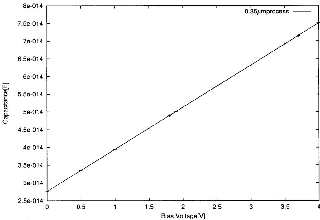
**Figure 4.9** Relation between capacitance and bias voltage (case of CMOS 0.6 μm process technology)
