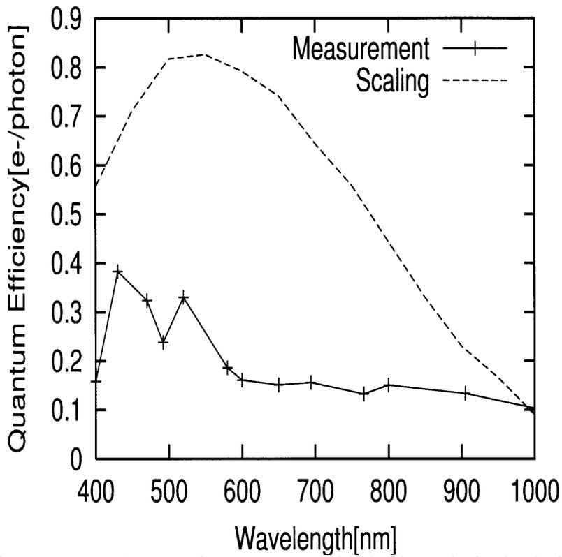
**Figure 5.13** Comparison Results of measurement with the theoretical value in  $0.35\mu\text{m}$  process
