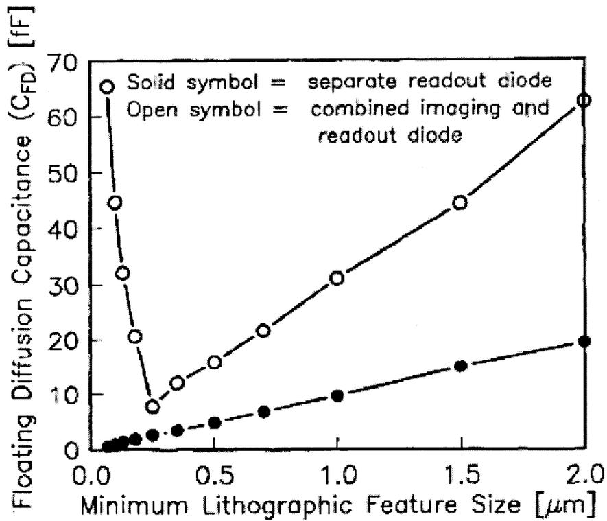
Figure 5.14 Floating Diffusion node capacitance as a function of the minimum feature size[16].
