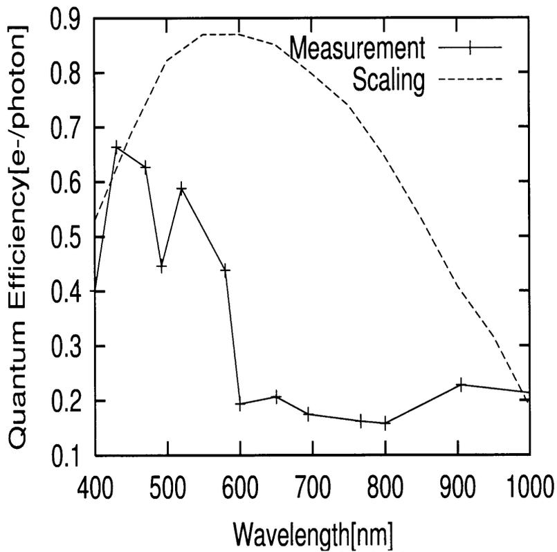
Figure 5.12 Comparison Results of measurement with the theoretical value in 0.6  $\mu\text{m}$  process
