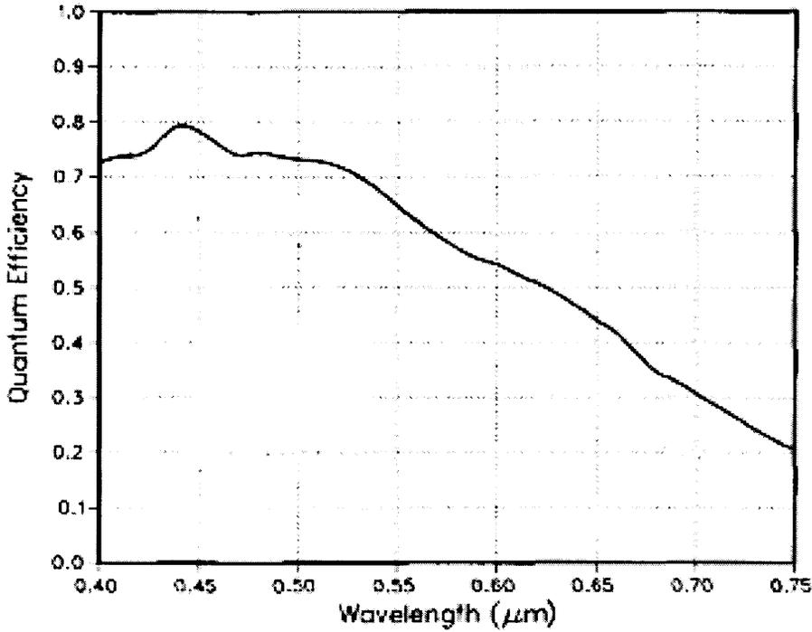
Figure 3.6 Quantum Efficiency of CCD[18]
