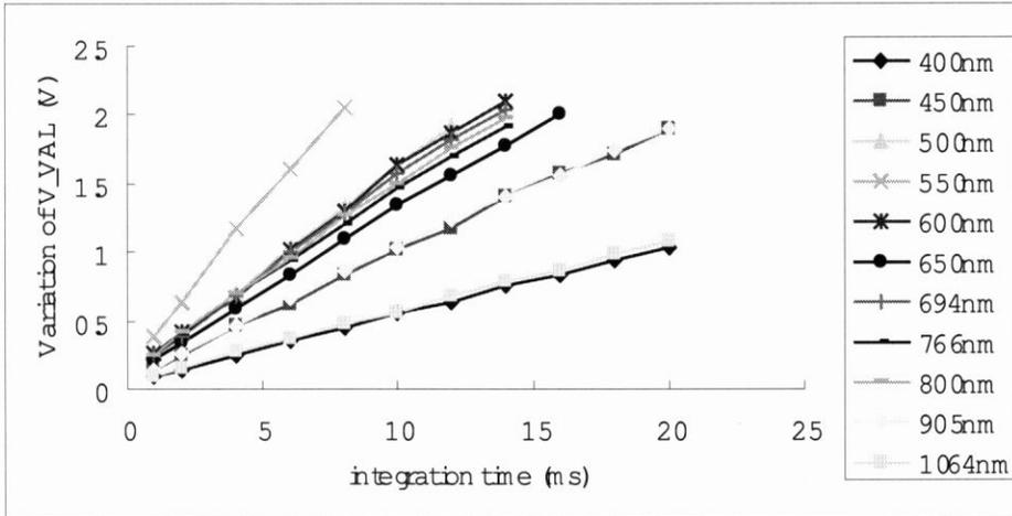
**Figure 4.13** Variation of  $V_{val}$  per integration time[ms](case of CMOS  $0.35\mu$  process technology)
