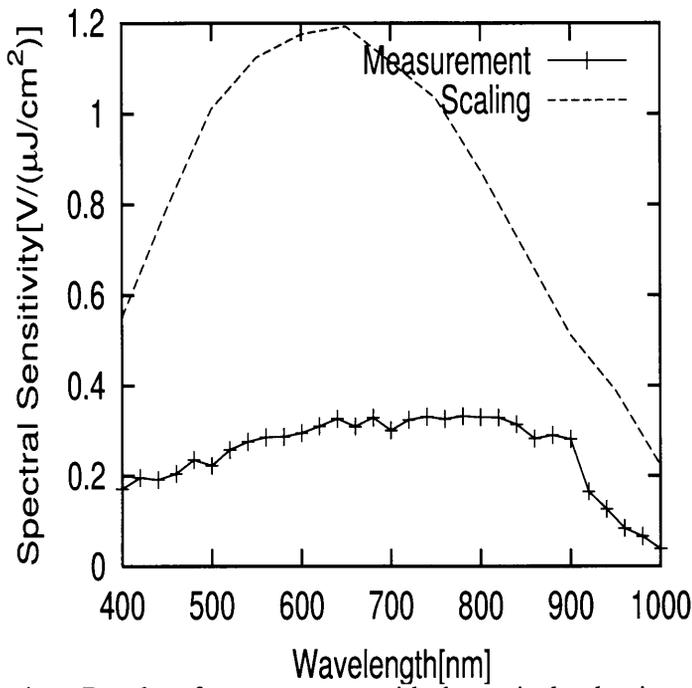
**Figure 5.19** Comparison Results of measurement with theoretical value in a 0.35μm process technology
