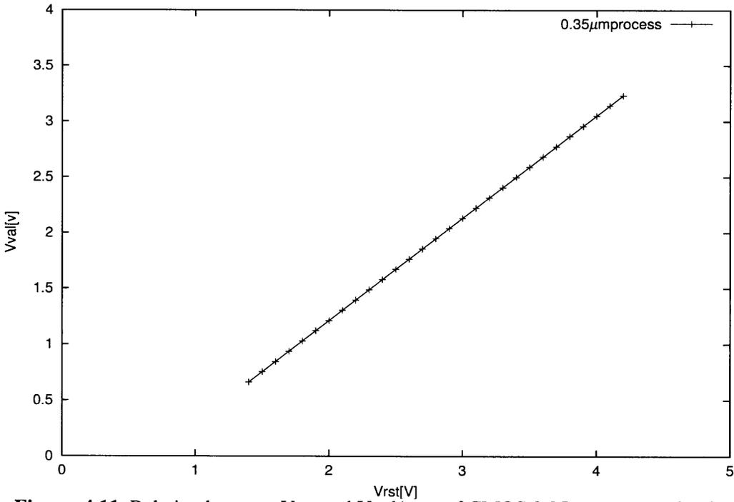
Figure 4.11 Relation between  $V_{rst}$  and  $V_{val}$ (case of CMOS 0.35 $\mu$  process technology)
