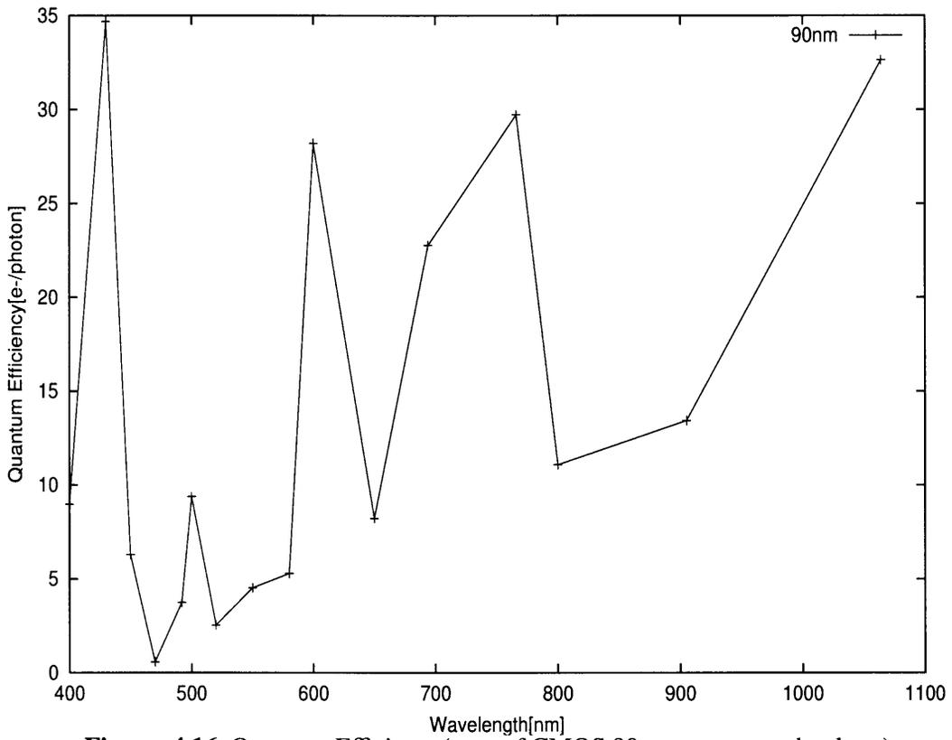
Figure 4.16 Quantum Efficiency(case of CMOS 90nm process technology)
