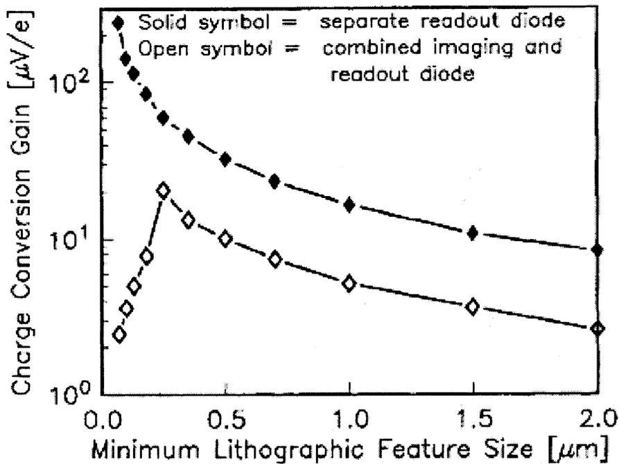
Figure 5.15 Charge to voltage conversion gain as a function of the minimum feature size[16].
