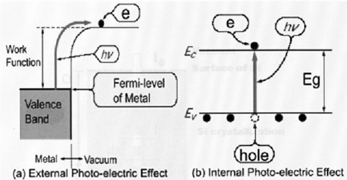
Figure 3.3 Photoelectric Effect
