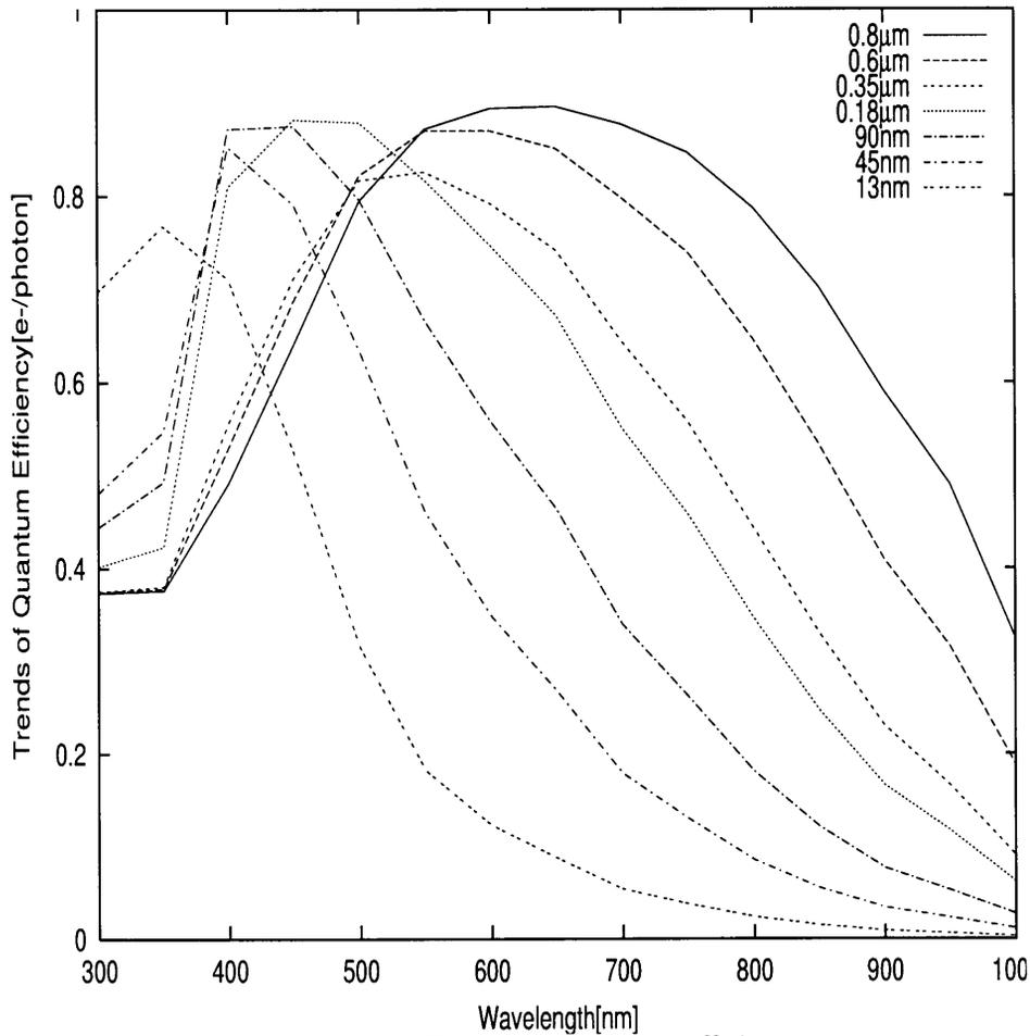
**Figure 5.10** Trends of Quantum Efficiency
