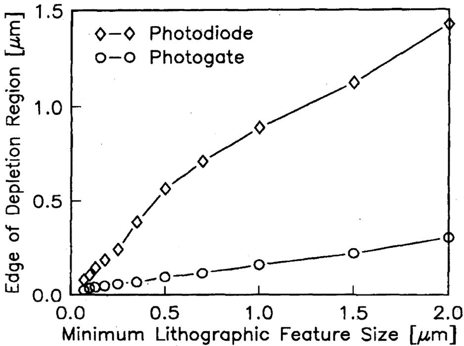
**Figure 5.7** The location of the edge of the depletion region as a function of  $L_g$
