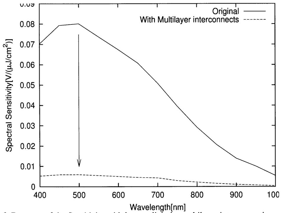
**Figure 6.6** Decrease of the Sensitivity with loss of light by multilayer interconnections and low-k layers
