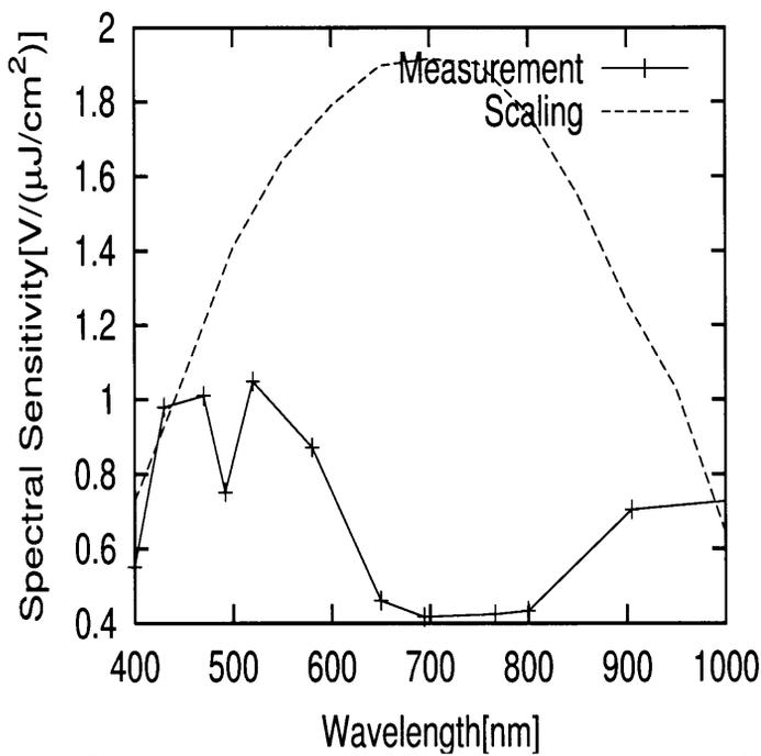
**Figure 5.20** Comparison Results of measurement with theoretical value in a 0.6μm process technology
