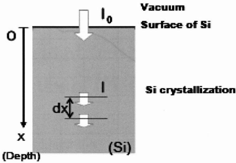
Figure 3.4 State of light absorption
