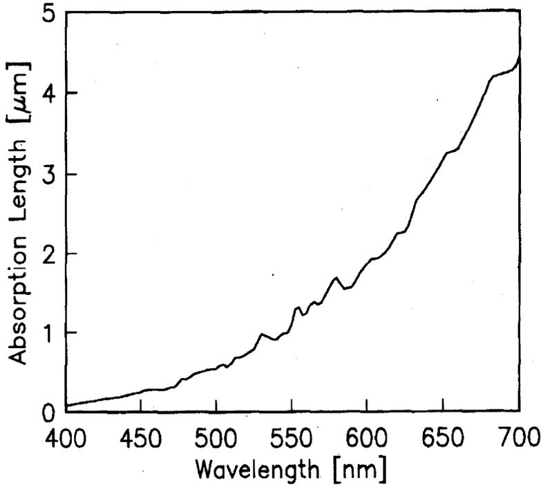
**Figure 5.8** Light absorption length in silicon. Data from E.Palik [22]
