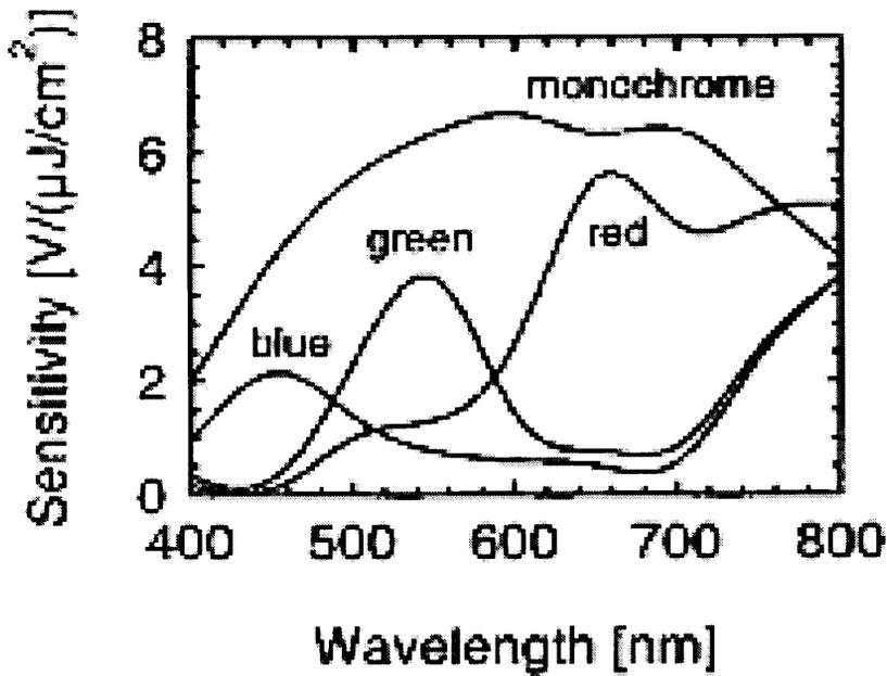
Figure 3.2 Monochrome and color sensitivity of a PPD imager[7]
