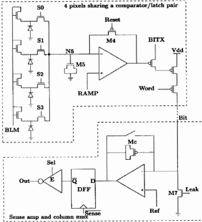
Figure 2.1 Example of CMOS image sensor's pixel block and column sense amplifier circuit
