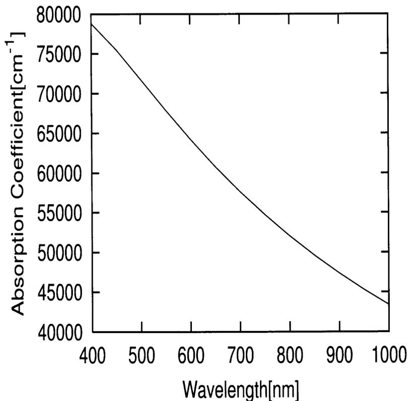
Figure 6.2 Absorption coefficient( $\text{SiO}_2$ )
