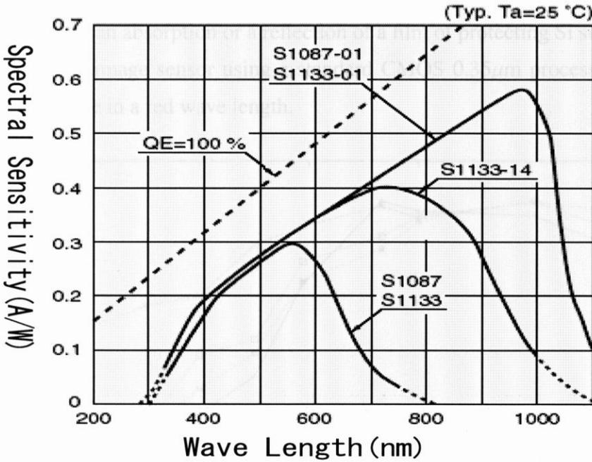
**Figure 4.5** Spectral Sensitivity of photodiode(S1087-01)
