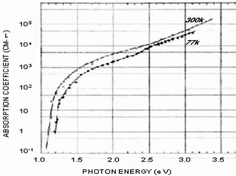
Figure 3.5 Absorption Spectra of single-crystal silicon at 77K and 300K[10]
