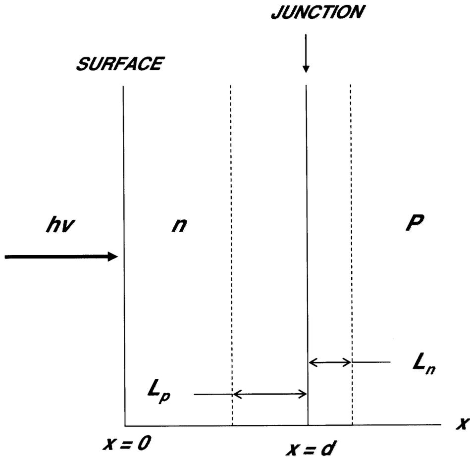
**Figure 5.9** One-dimensional geometry with junction depth  $d$  and minority carrier diffusion lengths  $L_n$  and  $L_p$  for the  $P$  side and  $n$  side [15, 21]
