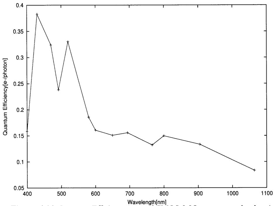
**Figure 4.14** Quantum Efficiency(case of CMOS 0.35 $\mu$  process technology)
