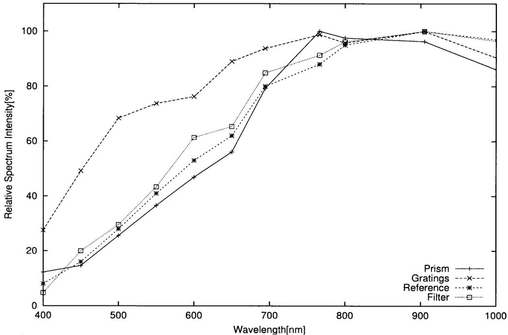
**Figure 4.6** Relative Spectrum Intensity measured by photodiode(Compared lamp's data with results using filter and prism)
