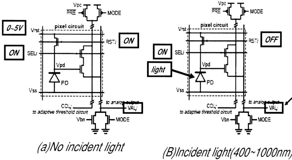
Figure 4.10 Measurement of  $V_{rst}$  and  $V_{val}$
