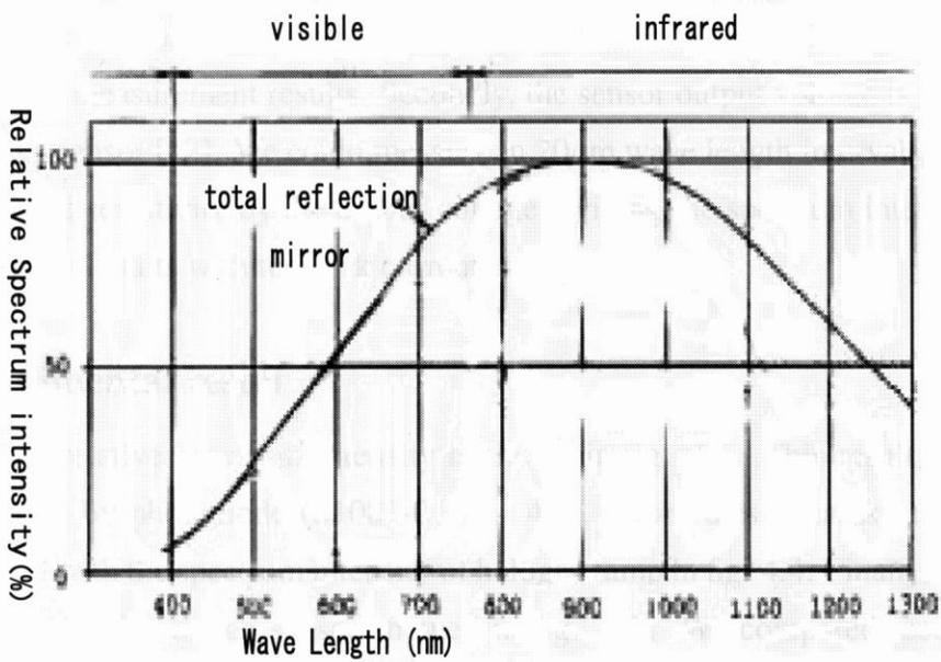
Figure 4.4 Relative Spectrum Intensity of Halogen Lamp JCR15V150WH5
