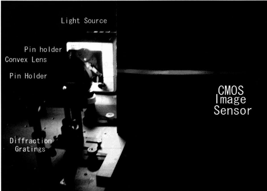
Figure 4.3 Optical system(in the case of a gratings)
