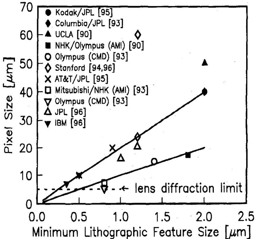
**Figure 2.2** Scaling trend of CMOS imager pixel size. Symbols are experimental data reported in the literature. The line represents linear scaling. The upper solid shows pixel size scaling as  $20L_g$  (typical of 4-transistor photodiode designs), the lower solid line shows pixel size scaling as  $16L_g$  (typical of 3-transistor photodiode designs),  $L_g$  is the minimum lithographic feature size.[16]
