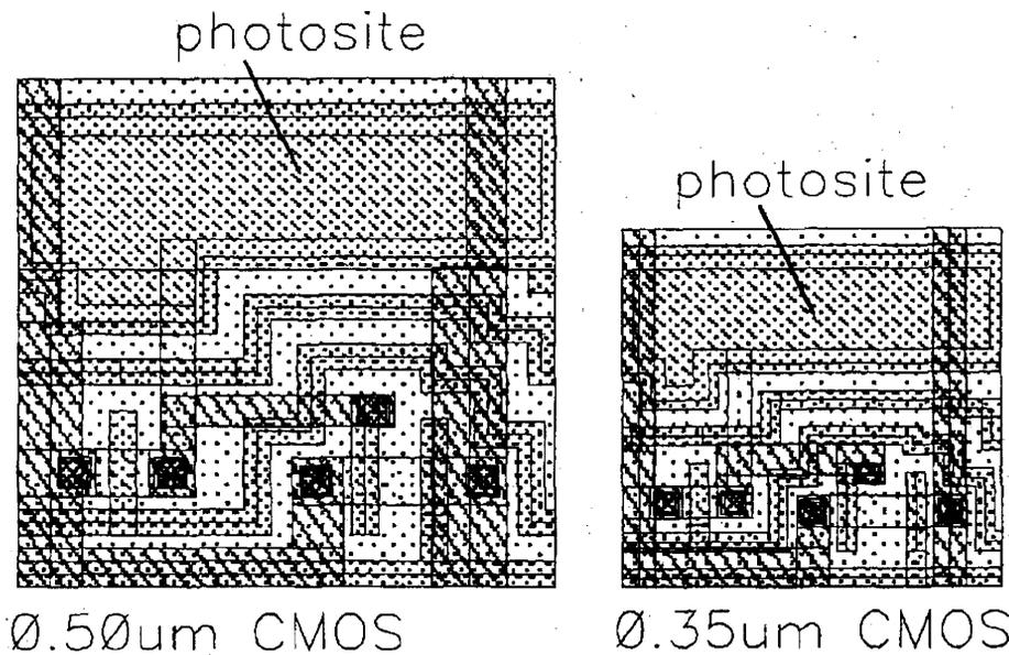
**Figure 2.3** Example layout for a  $0.5\mu\text{m}$  technology ( $10\mu\text{m}$  pixel) and  $0.35\mu\text{m}$  technology ( $7\mu\text{m}$  pixel).
