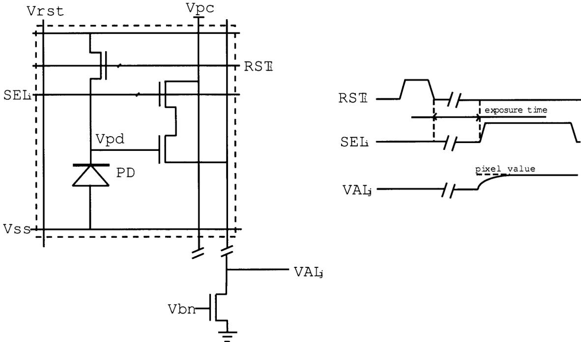
Figure 3.1 Pixel Circuit and Readout operation[12]
