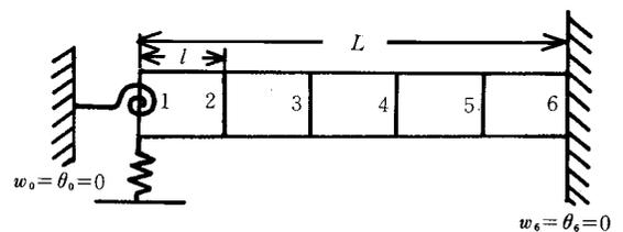
Figure 1 Virtual spring elements and finite element division
