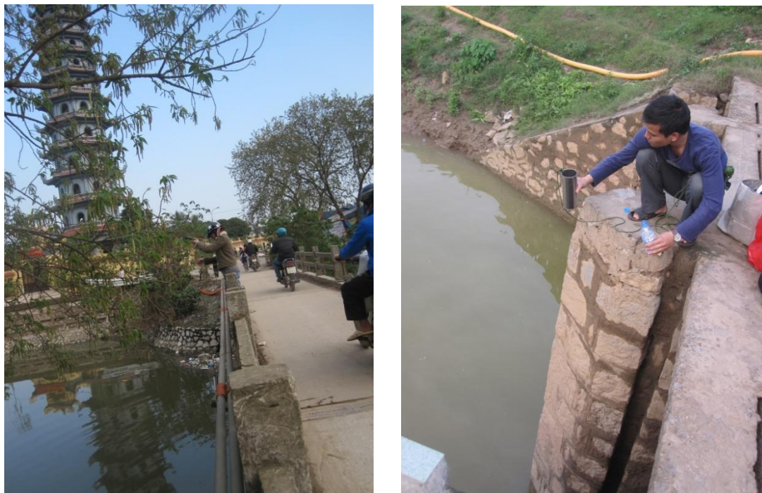
Figure 25. Taking sample with Sampling bucket and rope (Photo taken in March, 2011)
