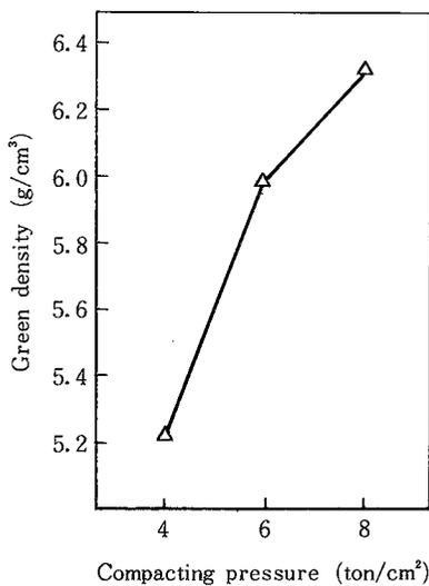
Fig. 3 Relation between compacting pressure and density.
