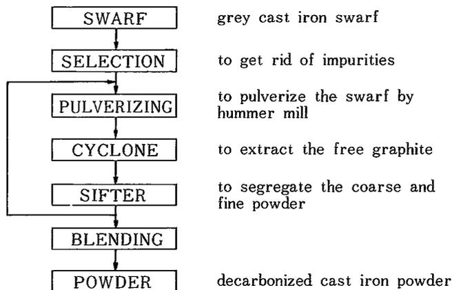
Fig. 1 Manufacturing process of the decarbonized cast iron powder from swarf.
