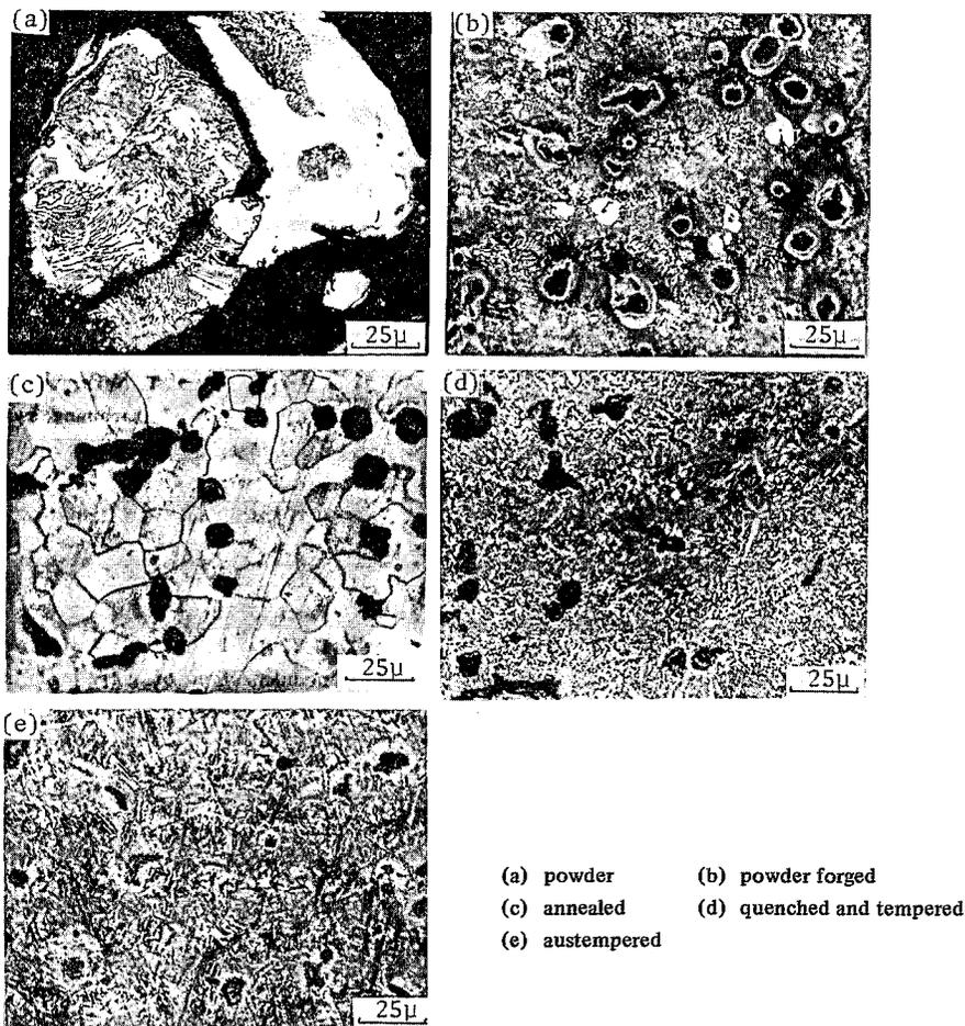
Fig. 7 Micrographs of powder and powder forged decarbonized cast iron.
