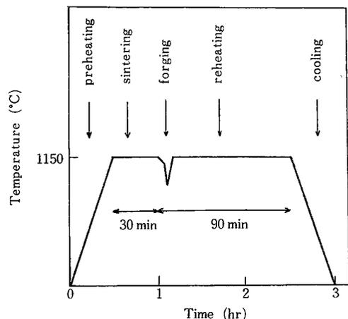
Fig. 6 The forging process of decarbonized cast iron powder.
