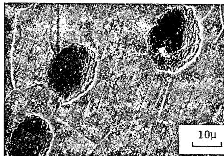
Fig. 9 Scanning electron micrograph of the powder forged product of decarbonized cast iron.
