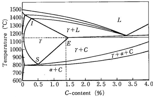
Fig. 10 Sliced phase diagram of Fe-C-Si (3%) alloy.
