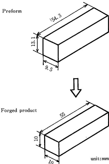
Fig. 5 Dimensions of preform and powder forged product.
