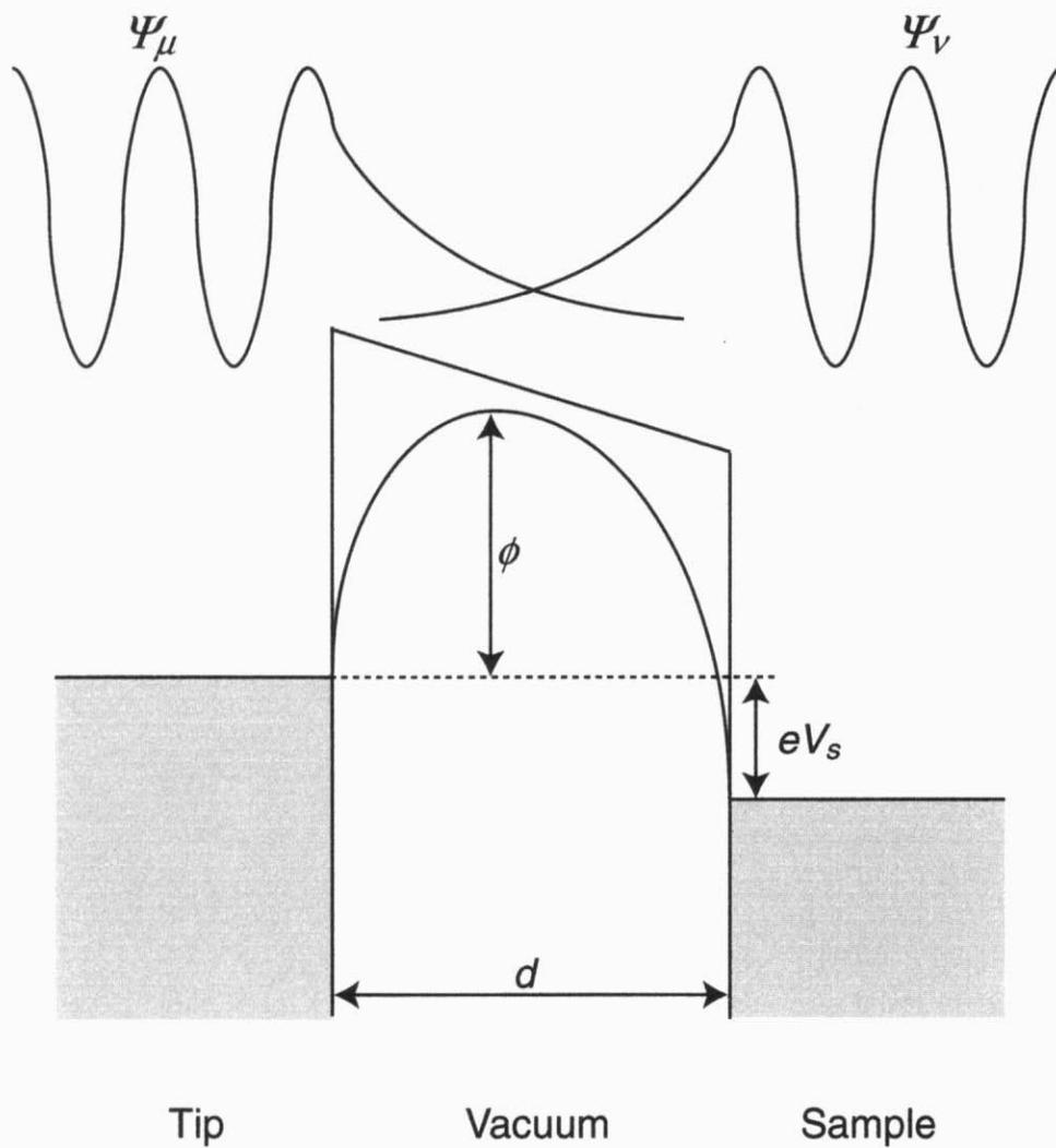
**Figure 2.3** Schematic potential diagram for STM.
