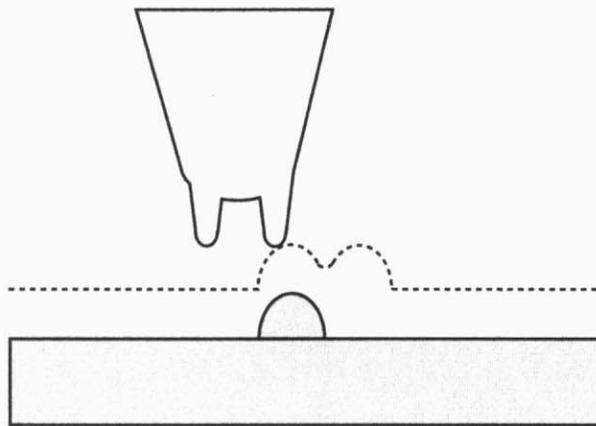
Figure 2.4 Effects of tip shape on measured STM profile.
