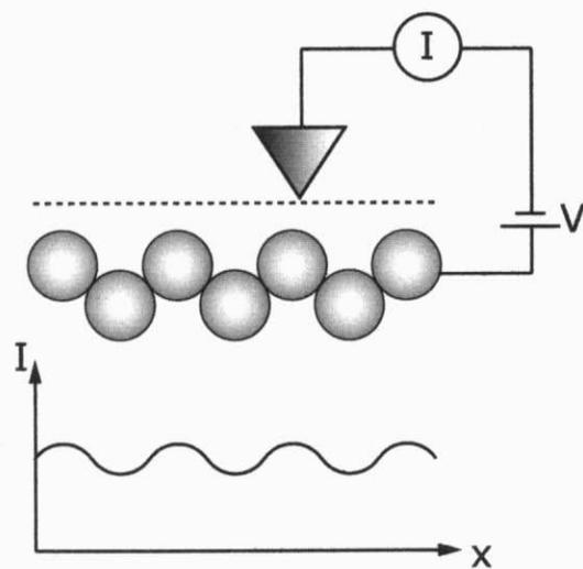
**Figure 2.2** Schematic drawings of imaging mode in STM.
