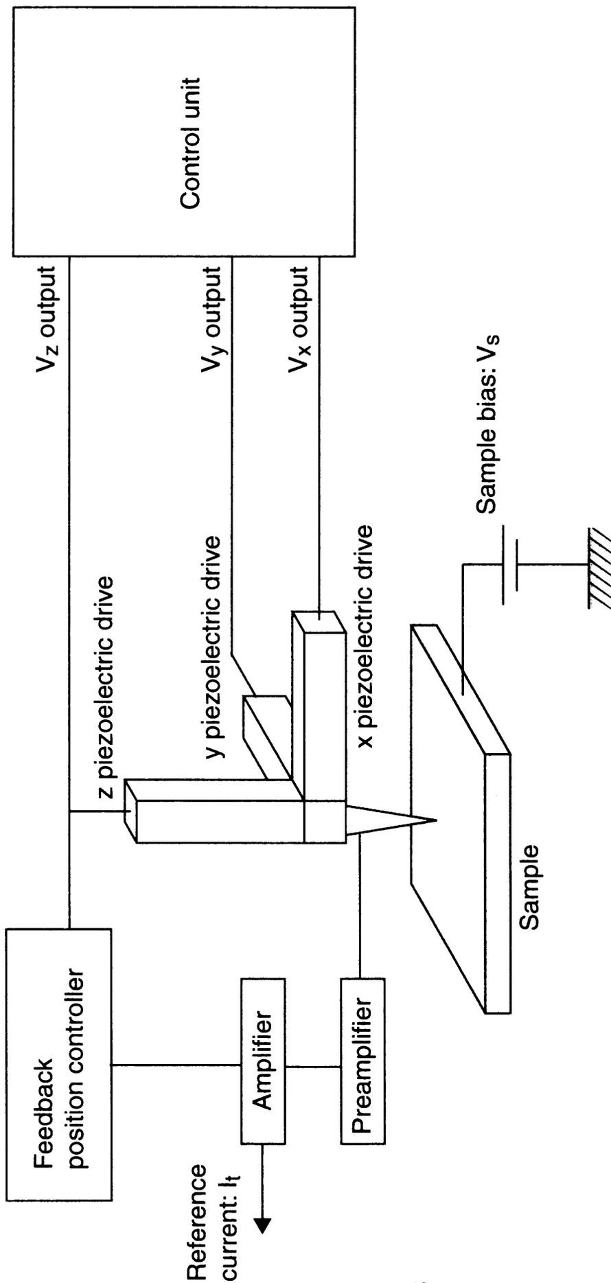
**Figure 2.1** Schematic drawing of an experimental system of STM
