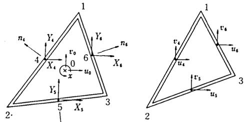
Fig. 3 Two types of Hybrid Displacement Models for In-plane Deformation Problems.
