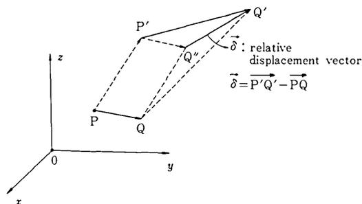
Fig. 1 Relative Displacement Vector  $\vec{\delta}$  in 3D Cartesian Space
