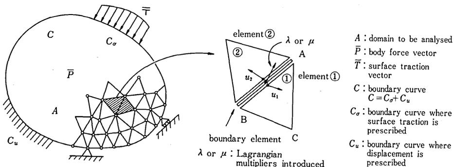
Fig. 2 Finite Element Analysis of Two Dimensional Displacement Field
