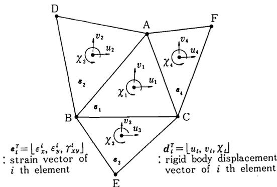
Fig. 4. A set of four CST Elements
