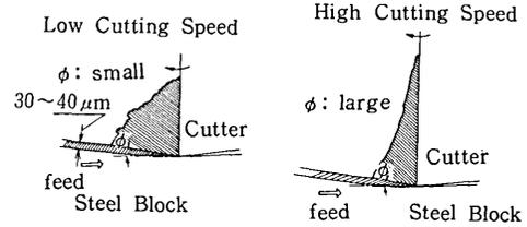
Fig. 4 Effect of the cutting speed on the shear angle  $\phi$  ( $D = \phi 100$  mm,  $\theta = 0^\circ$ )
