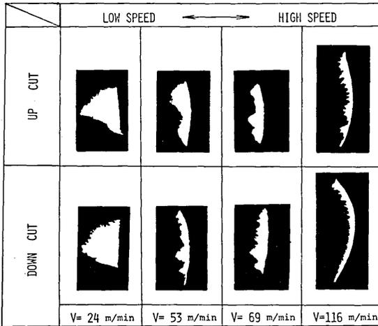
Fig. 2 Effect of the cutting speed on the cross sectional geometry of fibers (18-8 Stainless steel,  $S_z \approx 0.4$  mm,  $t = 0.4$  mm,  $\alpha = 15^\circ$ ,  $\theta = -15^\circ$ ,  $D = \phi 100$  mm)
