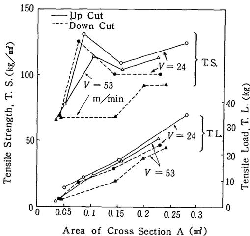
Fig. 10 Effect of the area of cross-section on the strength of fibers
