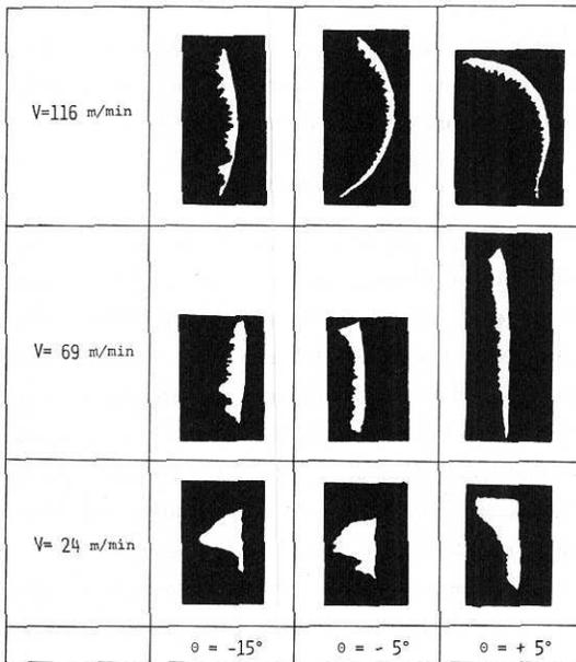
Fig. 5 Effect of the rake angle on the cross-sectional geometry of fibers
