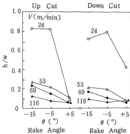
Fig. 6 Effect of the rake angle on the cross sectional geometry of fibers
