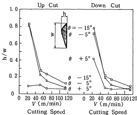
Fig. 3 Effect of the cutting speed on the cross sectional geometry of fibers (18-8 Stainless steel,  $S_z \approx 0.4$  mm,  $t = 0.4$  mm,  $\alpha = 15^\circ$ ,  $D = \phi 100$  mm)
