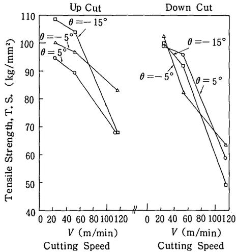
Fig. 9 Effect of the cutting speed on the strength of fibers
