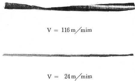
Fig. 7 Effect of the cutting speed on the appearances of the fiber
