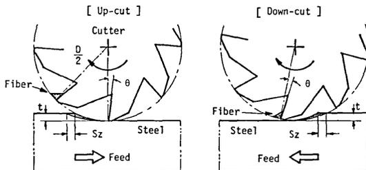
Fig. 1 Schematic principle of production of fibers by a milling machine
