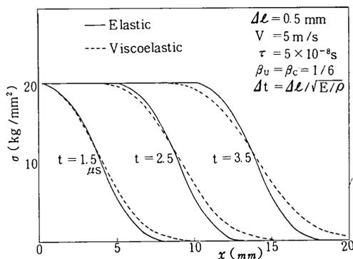
Fig. 2 Wave front decay due to viscous damping in steel compared with elastic stress wave
