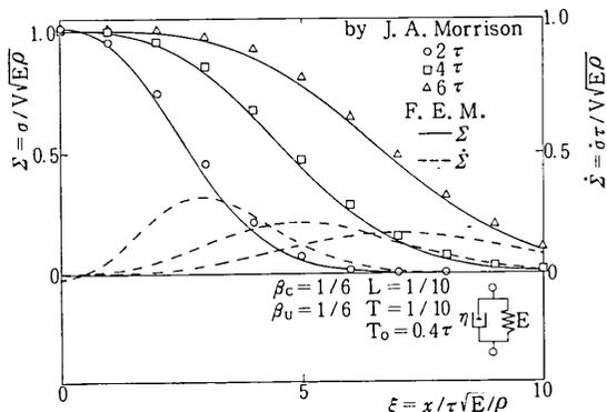
Fig. 1 Stress wave propagation in Voigt solid from impacted end
