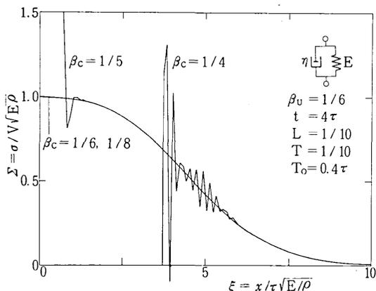
Fig. 3 Instability caused by inadequate choice of parameter  $\beta_c$  and time increment
