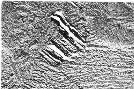
Fig. 7 Electronmicrograph of the cracks on copper strike surface
