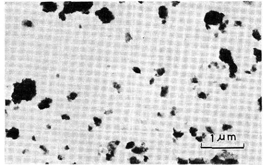
Fig. 1. Electronmicrograph of air ground  $\text{MoS}_2$
