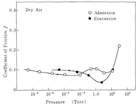
Fig. 2. Variation of coefficient of friction with dry air pressure for oleophilic  $\text{MoS}_2$
