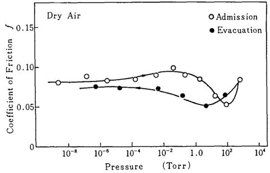
Fig.5. Variation of coefficient of friction with dry air for cleavage plane of  $\text{MoS}_2$  single crystal.
