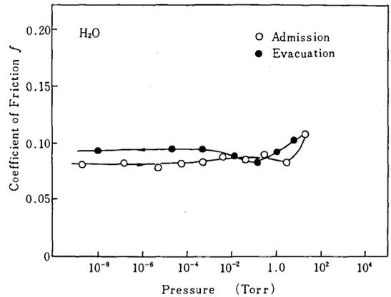
Fig.6. Variation of coefficient of friction with water vapour for cleavage plane of  $\text{MoS}_2$  single crystal.
