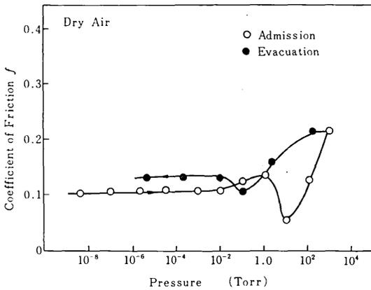
Fig.4. Variation of coefficient of friction with dry air for air ground  $\text{MoS}_2$ .
