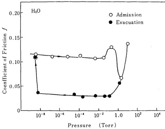
Fig.3. Variation of coefficient of friction with water vapour for air ground  $\text{MoS}_2$ .
