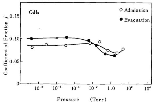
Fig.7. Variation of coefficient of friction with propane for cleavage plane of  $\text{MoS}_2$  single crystal.
