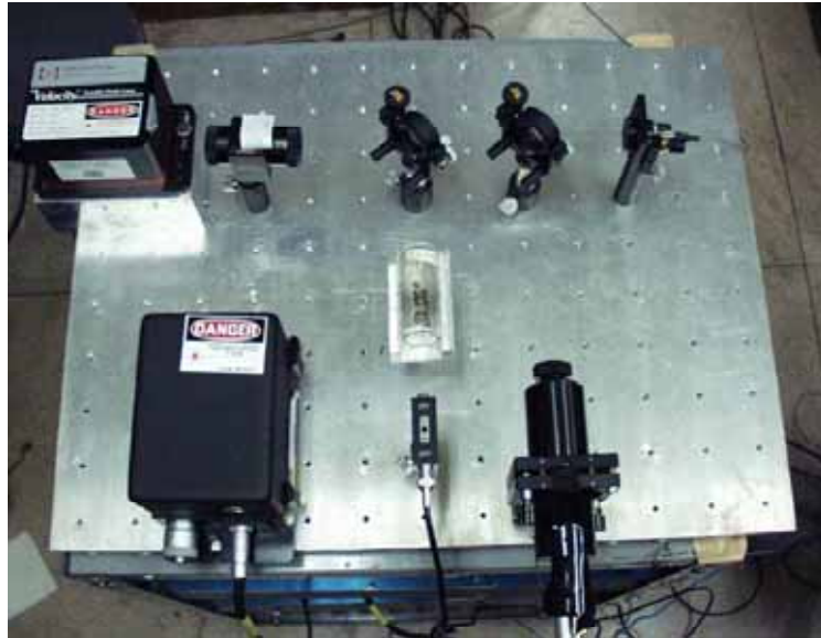
Fig. 2-5 Photograph of measurement system for laser absorption spectroscopy.
