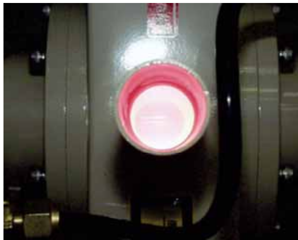
Fig. 3-8 Photo of microwave discharge tube plasma
