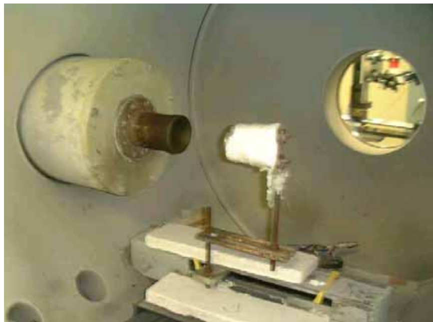
Fig.4-2 Photograph of JUTEM arc-heater.
