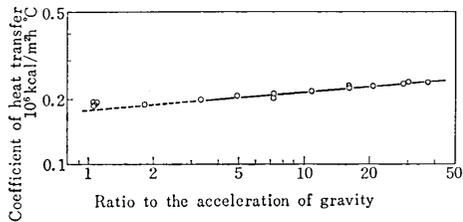
Fig. 3 Heat transfer coefficient vs. acceleration
