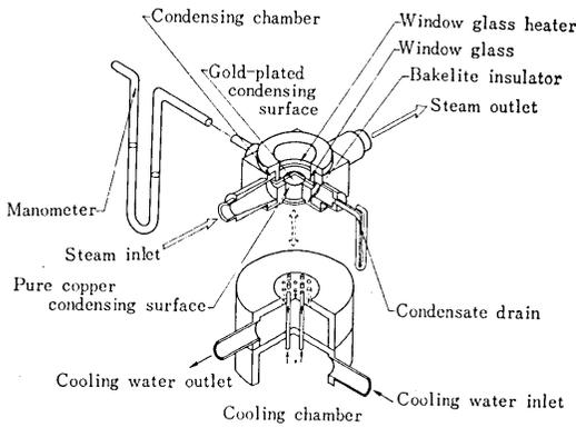
Fig. 2 Condensing chamber and cooling chamber
