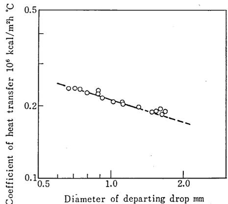
Fig. 5 Heat transfer coefficient vs. critical size
