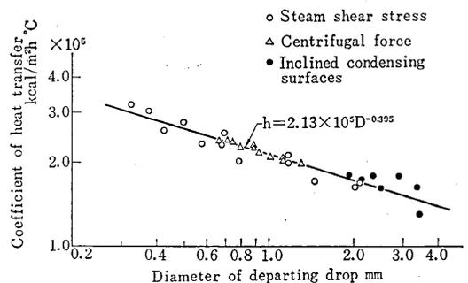
Fig. 6 Heat transfer coefficient vs. critical size
