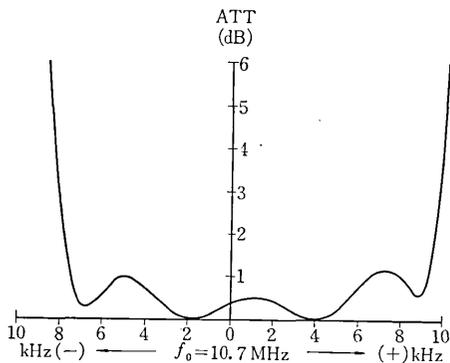
Fig. 3 Schematic of passband characteristics
