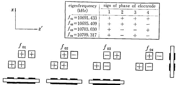
Fig. 5 Polarity of induced charge at eigenfrequencies
