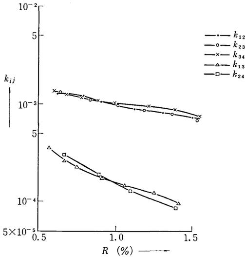
Fig. 2 Coupling factors  $k_{ij}$  as functions of electrode plateback  $R$
