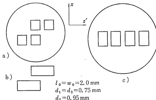
Fig. 1 Electrode configuration
