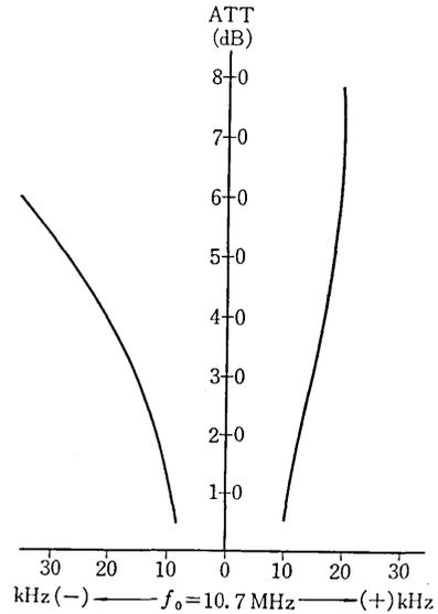
Fig. 4 Filter characteristics
