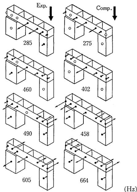
Fig. 2 The natural frequencies and the normal modes by the computation and the experiment for the integrated system.
