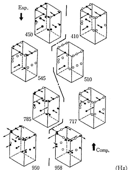
Fig. 1 The natural frequencies and the normal modes by the computation and the experiment for the thick column.
