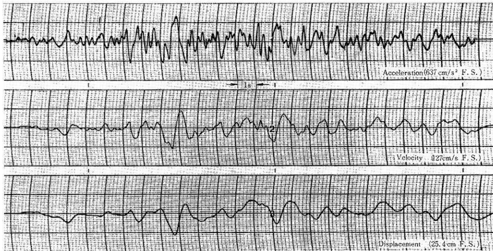
Fig. 4 Earthquake record and its integrated velocity and displacement for Akita Wave ( h=0.10 )
