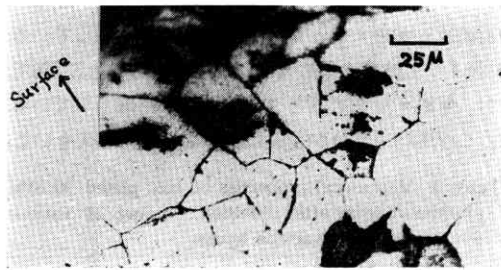
Photo. 1 Photomicrograph of grain boundary diffusion of zinc in aluminium. Sample: 99.85% aluminium wire cold drawn, zinc plated and diffusion heated at 400°C for 50 hr.
