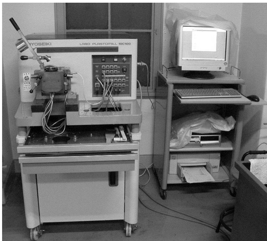
Fig. 6.5 Photograph of mixing machine, "LABO PLAST MILL model 10C100".
