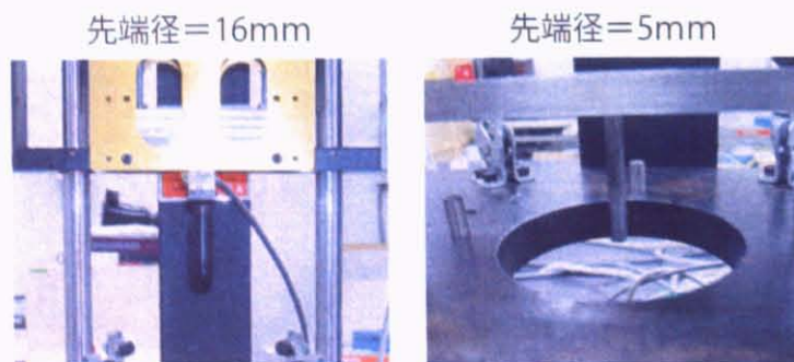
Fig.2.8 Shapes and sizes of the tips of tups used for low velocity impact test.
