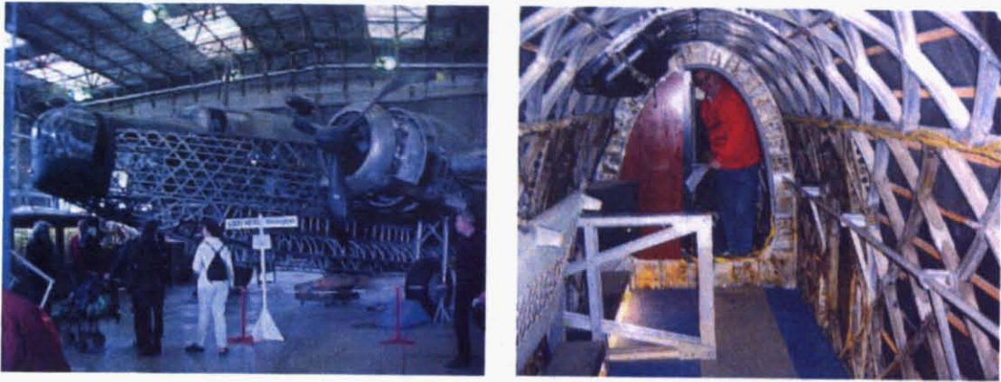
Fig.1.4 The Wellington bomber, an example of grid structures.
