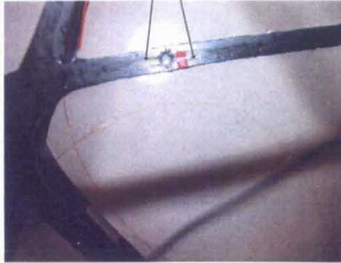
Fig.5.9 Photograph representing splitting on top surface of the rib.
