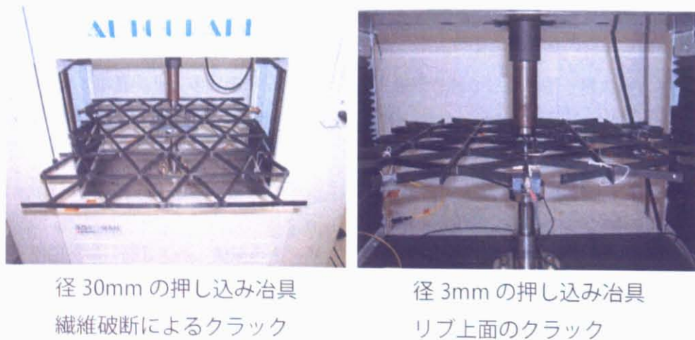
Fig.5.4 Three point bending test configurations for generating a fiber break and a splitting on top surface.
