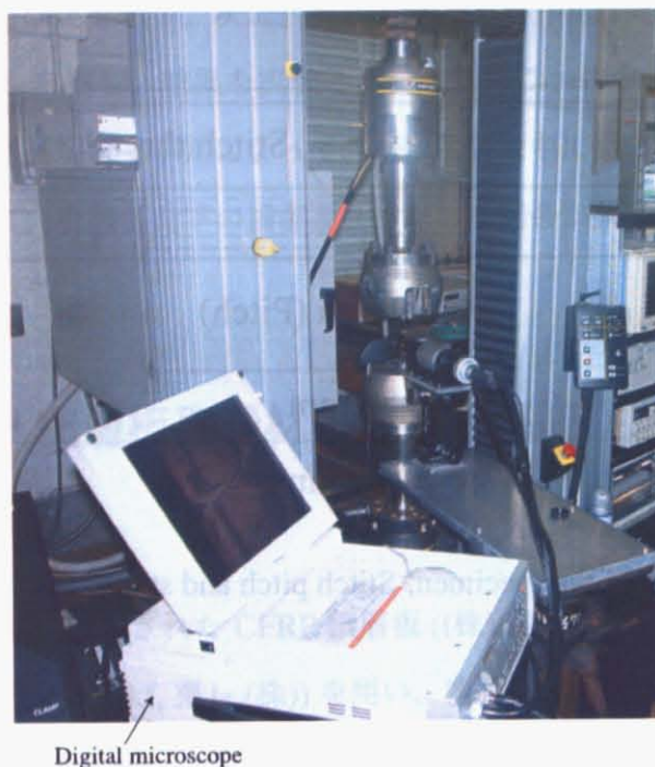
Fig. 3.3: Load-unload test setup
