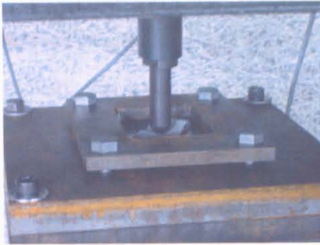
Fig. 5.3: Fixture of the drop weight impact test.
