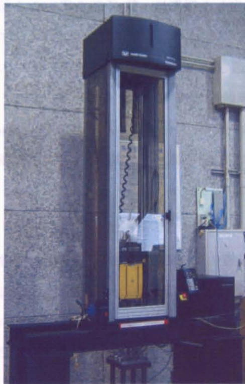
Fig. 5.2: Drop-weight impact test machine.
