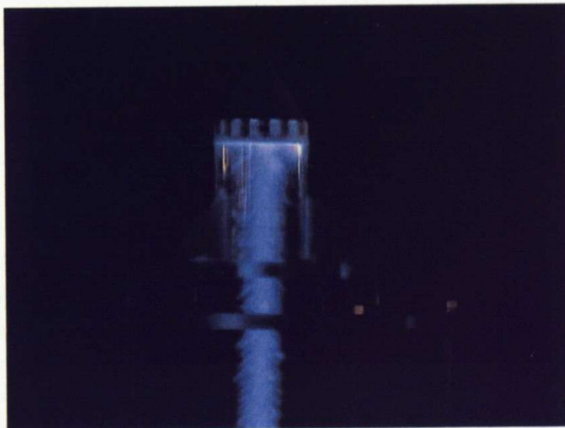
Figure 3.14: Photograph of plasma and cone-cylinder thruster model.
