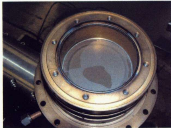
Figure 2.5: Diamond window set to the end of waveguide
