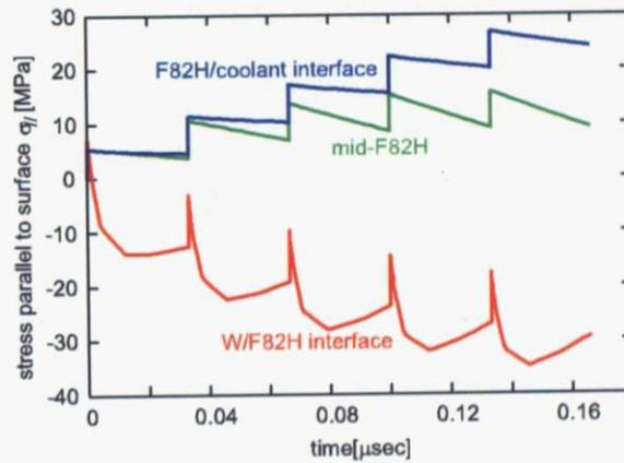
Fig. 5.14: Temporal stress evolution of F82H at the interface to tungsten, the midplane, and the interface to coolant.
