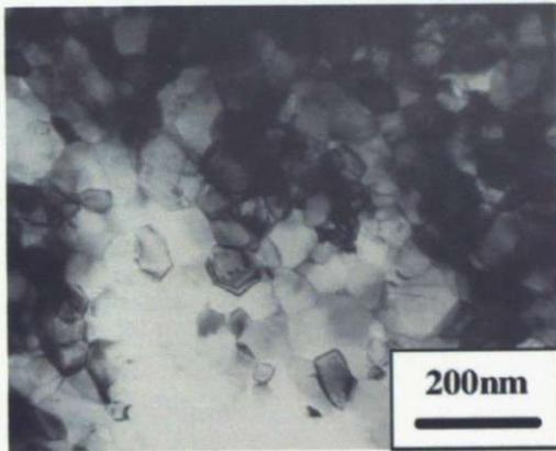
Fig. 5.24: A TEM bright-field image of the grain structure of an ultra fine-grained tungsten sample (a HIPed W-0.7%TiC compact processed with MA in an Ar atmosphere). This figure is derived from Fig. 3 of ref. [69].
