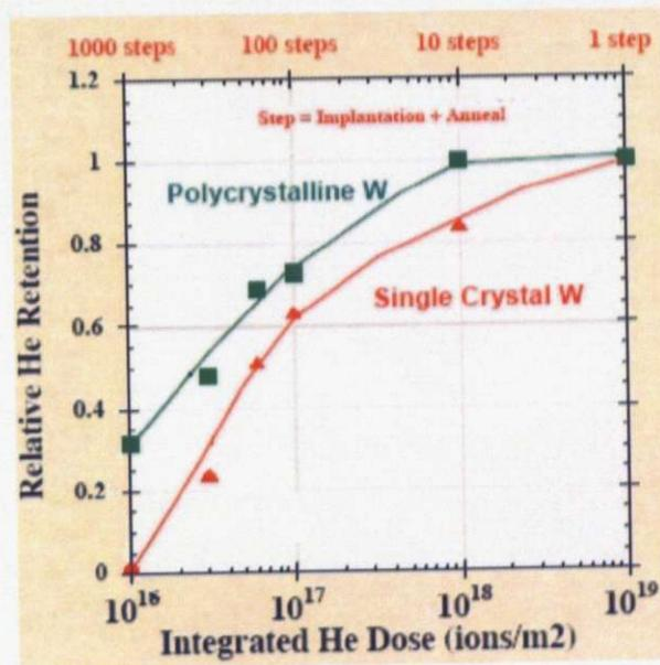
Fig. 5.19: Relative helium retention in polycrystalline and single crystal tungsten samples as a function of helium does per cycle for different number of pulses with temperature anneals (Figure 7 of reference [65].)
