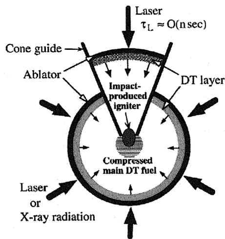
Fig. 7.2: Schematic view of the fuel pellet for the impact ignition (Fig. 1 of reference [85]).
