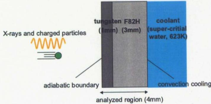
Fig. 5.1: Schematic view of the model used in the 1-D thermal analysis
