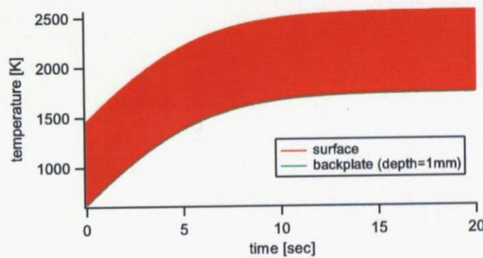
Fig. 5.15: Temporal temperature evolution of the first wall during 10 sec from the first shot in case that the first wall is only radiatively cooled
