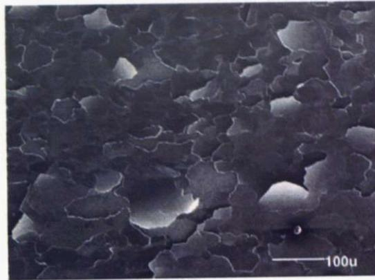
Fig. 5.17: A SEM image of tungsten test sample after irradiation of  $10^{21}\text{He}/\text{m}^2$  in HAPL experiment. Generation of numerous bubbles can be seen. (Fig. 2(b) from reference [61])
