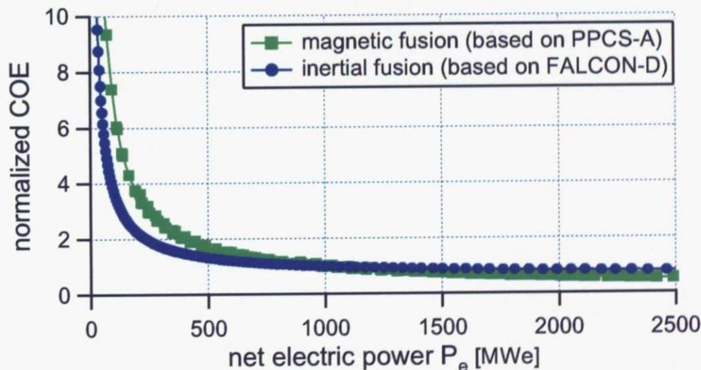
Fig. 7.1: Comparison of COE dependence on electric power output between a magnetic fusion reactor (based on PPCS model-A) and an IFE reactor (based on FALCON-D). COE is normalized by its value at the net electric power of 1 GWe.
