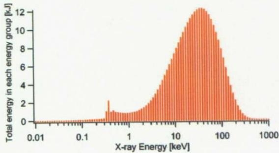
Fig. 5.2: Spectrum of X-ray from the core plasma
