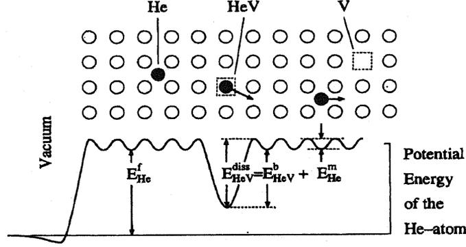
Fig. 5.20: Schematic view of the positions and corresponding energy of a helium in a metal lattice (FIG. 1 of reference [64]).
