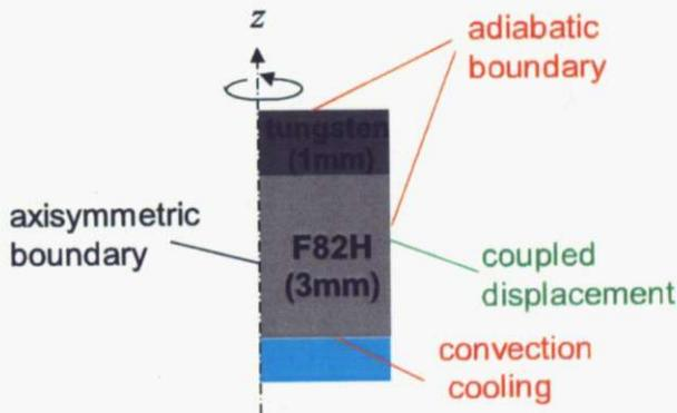
Fig. 5.6: Schematic view of the model used in the thermomechanical analysis
