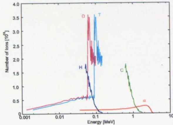
Fig. 5.3: Spectra of charged particles from the core plasma
