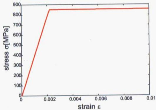
Fig. 5.7: Relation between stress and strain of tungsten used in this calculation
