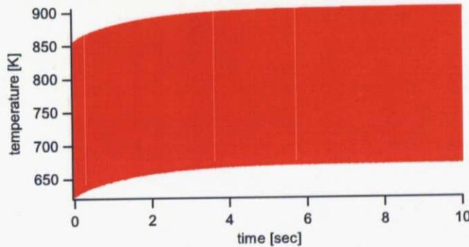
Fig. 5.12: Temporal temperature evolution of the first wall during 10 sec from the first shot in case of the chamber radius of  $R = 9.2$  m
