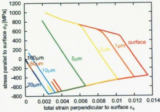
Fig. 5.8: Stress-strain behavior at various depths of the first wall during the first shot
