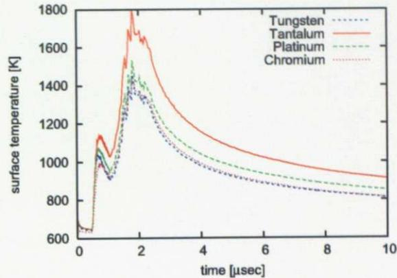
Fig. 5.23: Temporal temperature evolution of the first wall armor during the first shot if alternative materials (Cr, Ta, Pt) are used.
