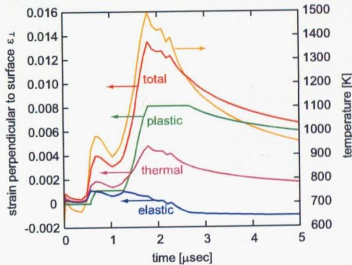
Fig. 5.10: Temporal strain evolution at the first wall surface during the first shot. Temperature evolution is also plotted (right scale).
