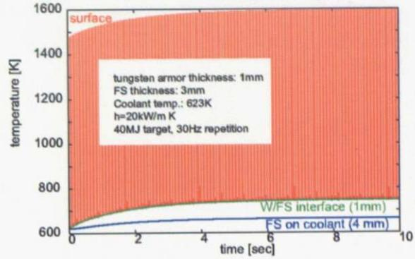
Fig. 5.5: Temporal temperature evolution of the first wall during 10 sec from the first shot
