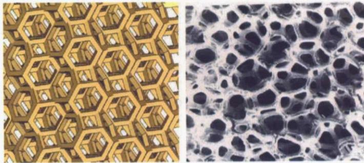
Fig. 5.21: Three dimensional solid model (left) and an optical micrographs (right) of tungsten foam (Fig. 9 from reference [66]).
