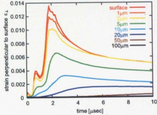
Fig. 5.9: Temporal evolution of total strain at various depths of the first wall during the first shot
