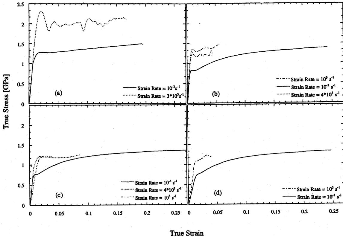
Fig. 5.13: Stress-strain curves for tungsten at different strain rates: (a) as-received; annealed (b) at 2023 K, (c) at 2873 K, and (d) at 3073 K.
