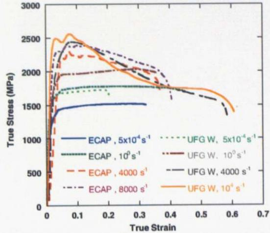
Fig. 5.25: Stress-strain curves of ECAP (Equal Channel Angular Pressing) W (grain size : a few  $\mu\text{m}$ ) and UFG-W with different strain rates (Fig. 3 of reference [72]).
