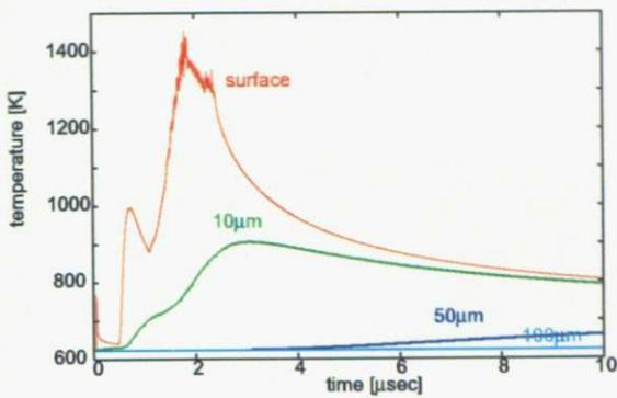
Fig. 5.4: Temporal temperature evolution at various depths of the first wall during the first shot
