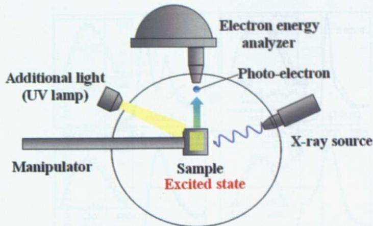
Figure 8.2: Schematic picture of the experimental setup.
