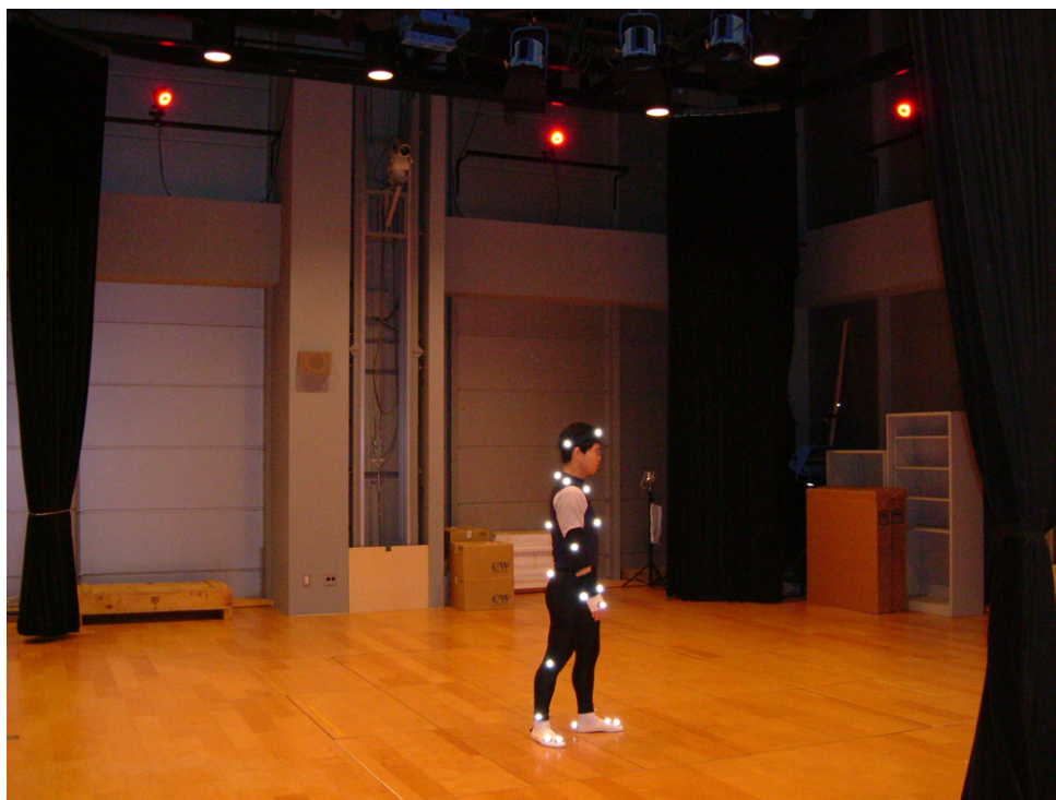
Figure B.1: Optical motion capture system. Red points are infra-red cameras, and white shining points on the human body are the optical markers.
