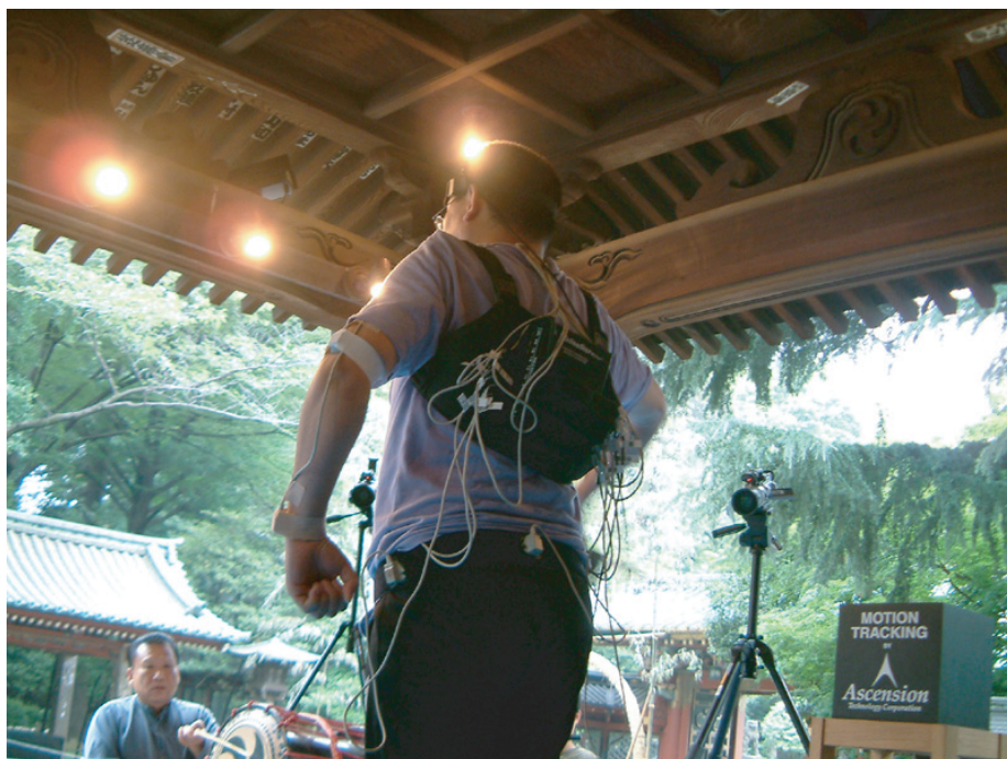
Figure B.3: Magnetic motion capture system. A black box on the right hand side is a transmitter. The performer is carrying a backpack, and magnetic markers are attached to the performer's body and are connected to the backpack.
