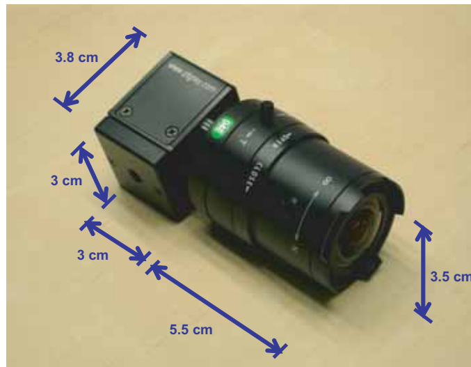
Figure 7.4: Size of the video cameras used for the 3D tracking implementation.
