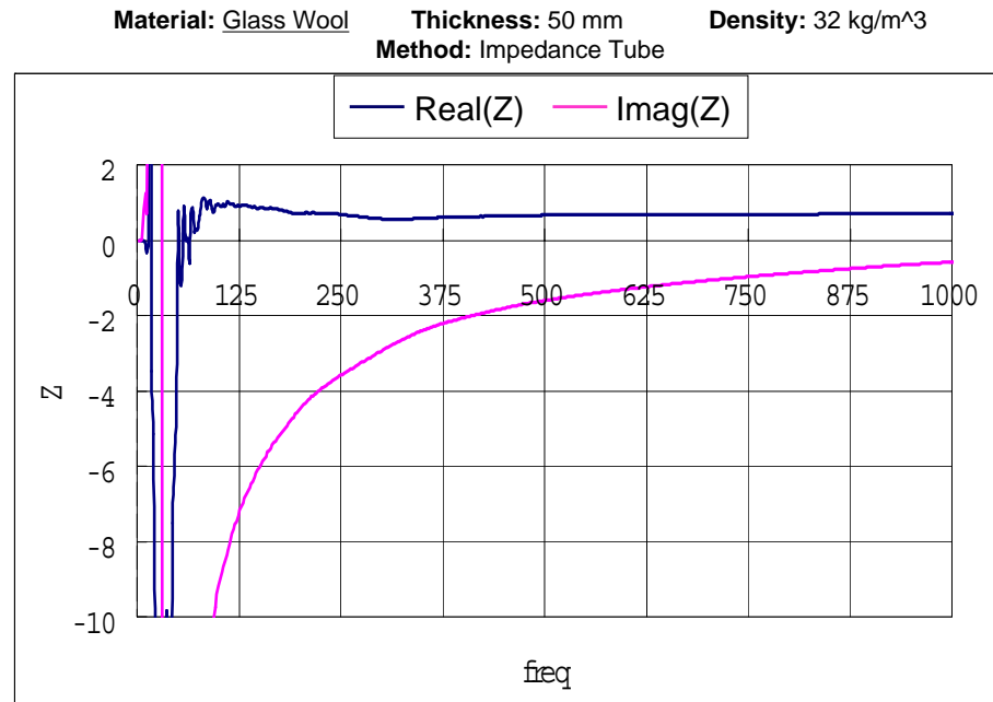
Figure A.2: Normal incidence impedance of the Glass wool measured with the impedance tube method.
