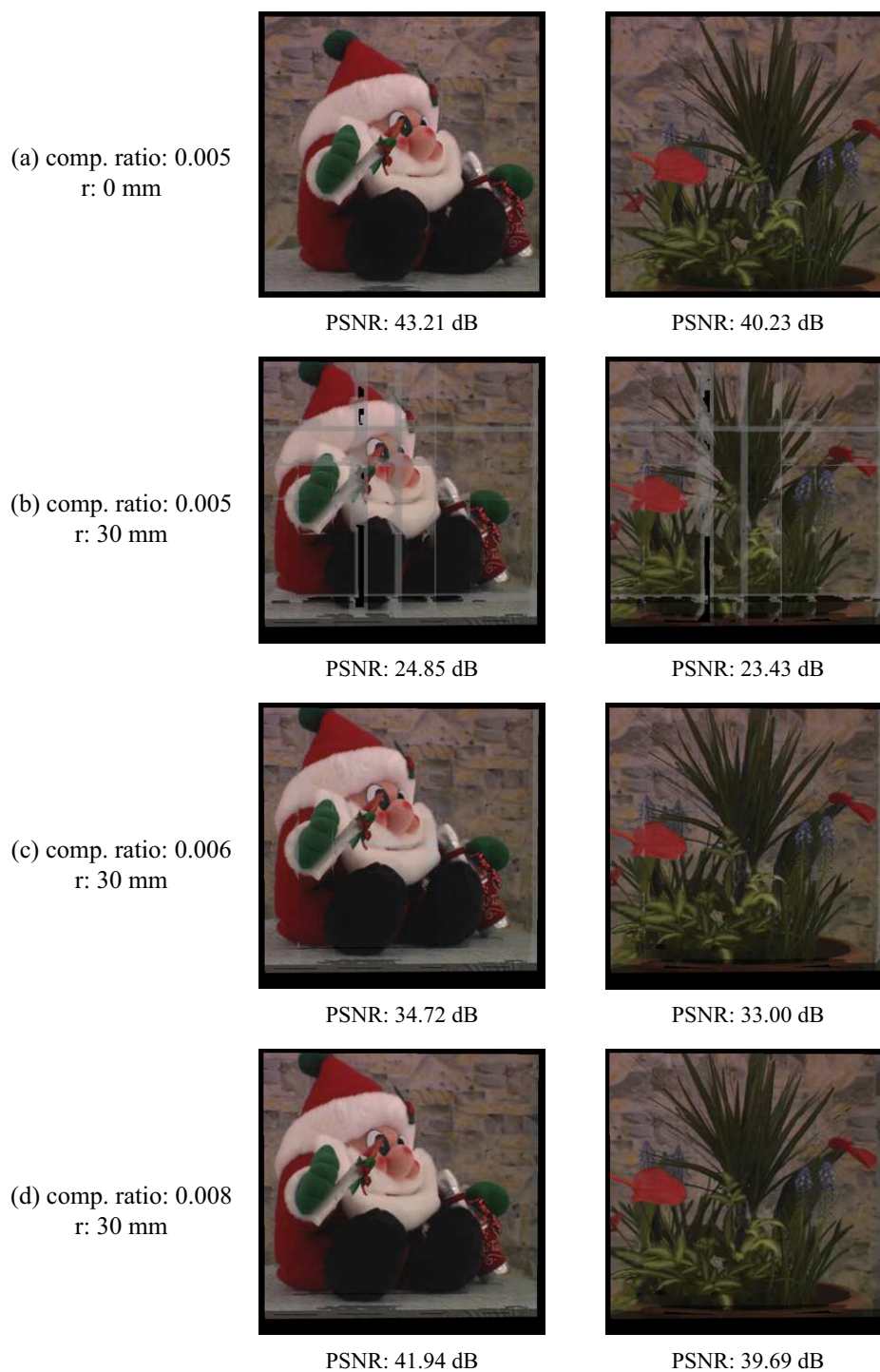
Figure 5.11: Synthesized images obtained using the sloping ROI for the Santa (left) and Plant (right) image sets. The Plant image set has same parameters as the Santa image set.
