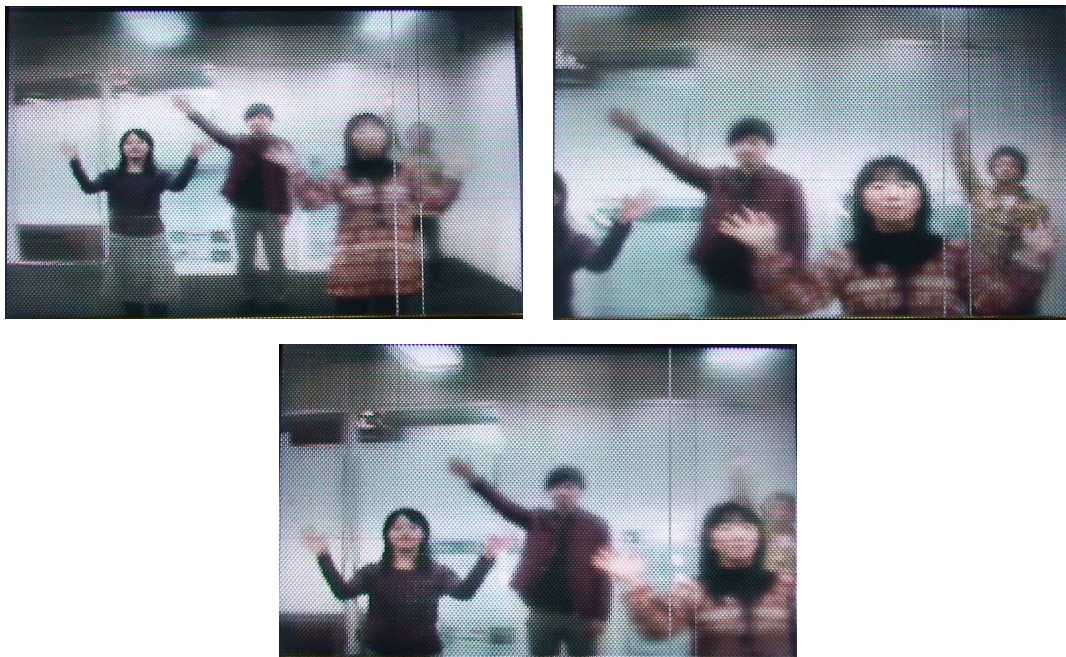
Figure 8.10: Displayed images obtained using different positions and view angles of the rendering cameras. Note that the display presents autostereoscopic 3D images for any target part of the scene.
