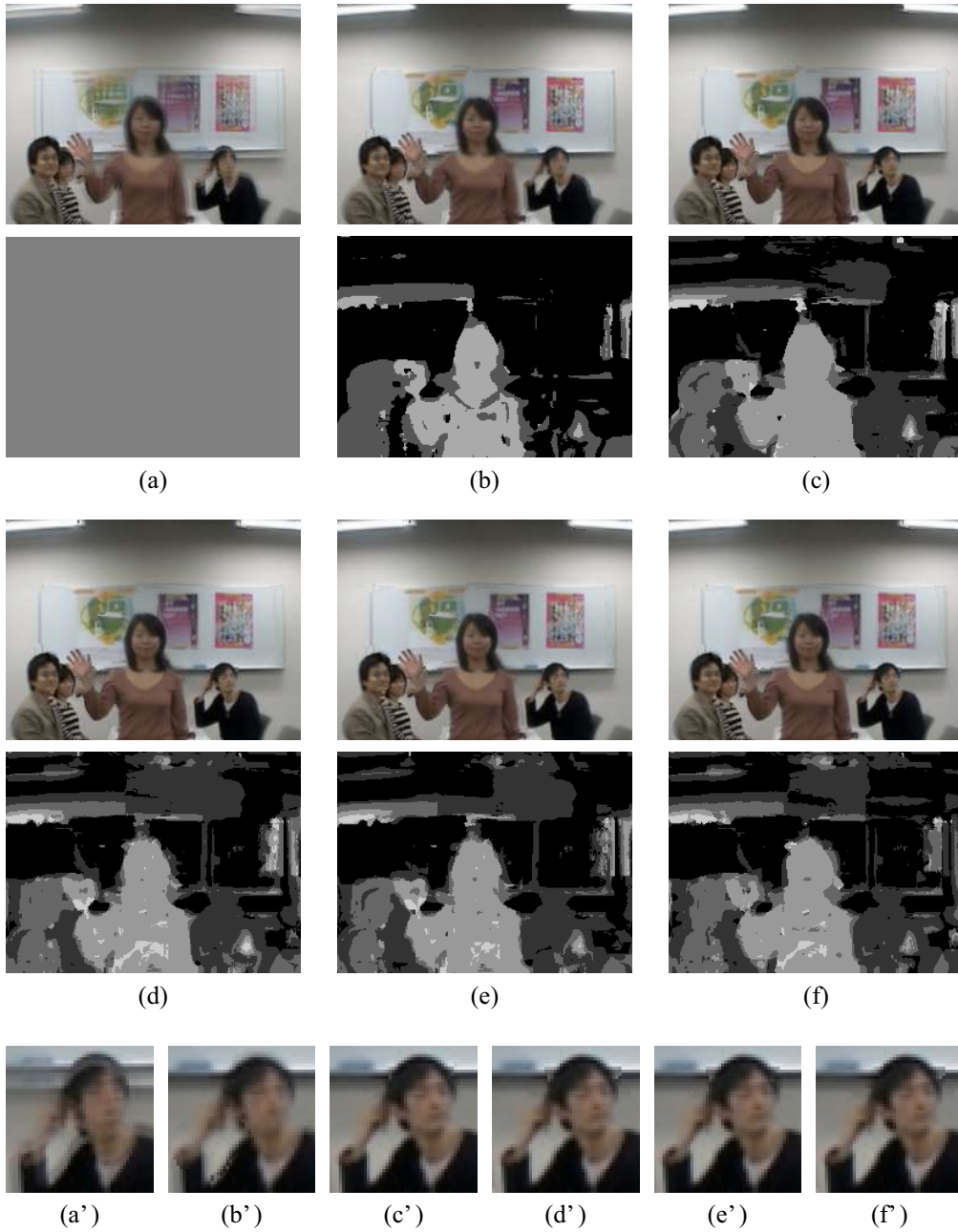
Figure 8.5: (a–f) Synthesized images and depth maps at the 38th viewpoint obtained using different number of depth layers and different rendering methods, and (a’–f’) close-up views of the right person in the corresponding images. (a–c) The depth estimation method at the viewpoint ( M = 1 ) using (a) a single layer, (b) 3 layers, and (c) 5 layers. The rendering quality increases with the increase of the number of depth layers. (d–f) The depth interpolation method with (d) M = 2 , (e) M = 3 , and (f) M = 4 , using 5 depth layers. The interpolated depth maps (d–f) are similar to the one estimated at the viewpoint (c), and the synthesized images are of comparable quality.
