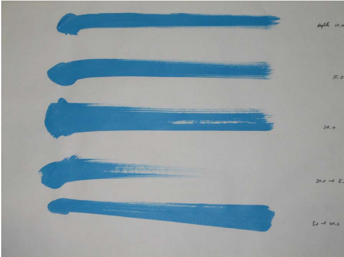
Fig. 6.13 Parameterized paintbrush technique: Changing the depth of vertical axis [mm]; 10, 15, 20, 20 to 5, 5 to 20, respectively.
