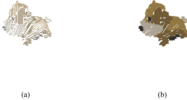
Fig. 4.6 Visual feedback painting with object segmentation using global range information with 1 brush size. (a) Trajectories, (b) Area filling result.
