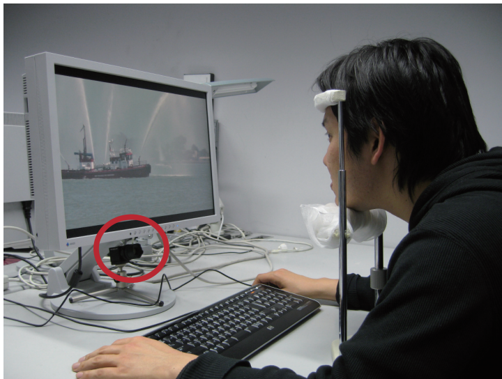
Figure 4.7: Experimental setup. A chin rest is used to fix their head positions, and a 22.0-inches WUXGA ( 473.8 \times 296.1 mm) display was placed 400 mm in front of the subject when video clips were shown. The red circle indicates the position of the camera.
