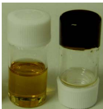
Figure 2.13 Wood solution (left, 1% concentration) and gel (right, 10% concentration, bottle is up side down) prepared from milled wood (2 h) in 6% LiCl/DMSO.
