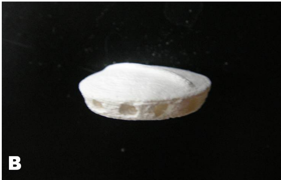
Fig. 3-1 (A) The design of the tailor-made implant. (B) Fabricated tailor-made implant with 6 cylindrical holes
