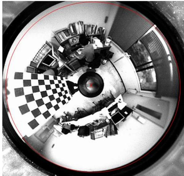
**Fig. 5-7 Extraction of the mirror boundary and estimation of the principle point**
