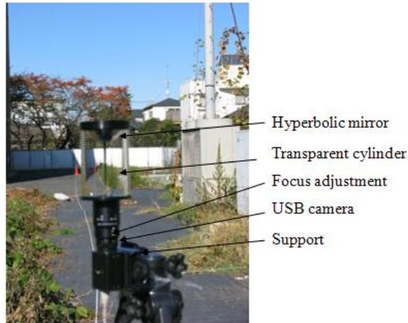
Fig. 3-6 Omnidirectional vision system structure
