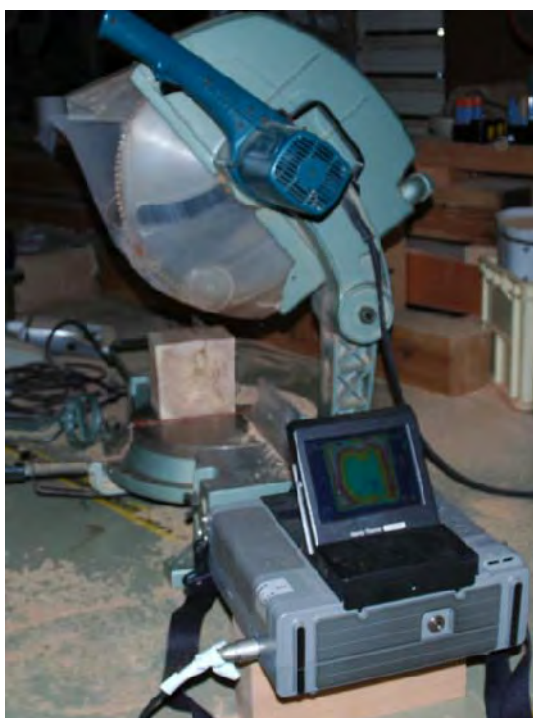
Fig.4-4 Thermal imaging on center surface of cross section after cutting.
