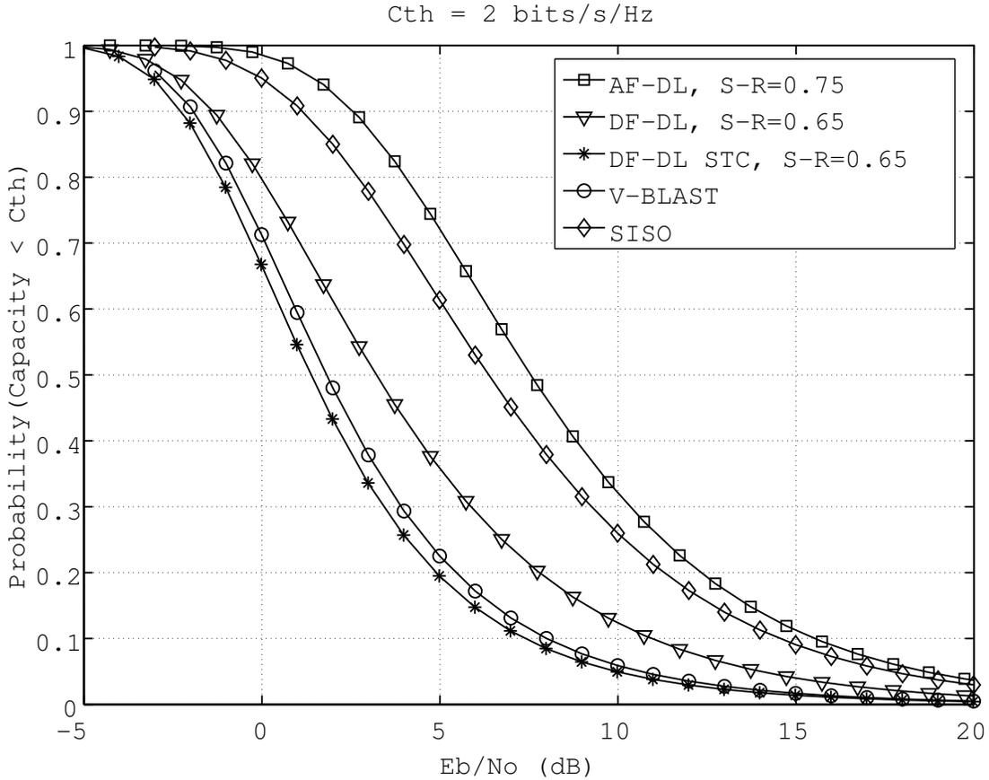
Figure 6.3 Outage capacity of downlink CSM systems,  $c_{th} = 2 \text{ bits/s/Hz}$ .
