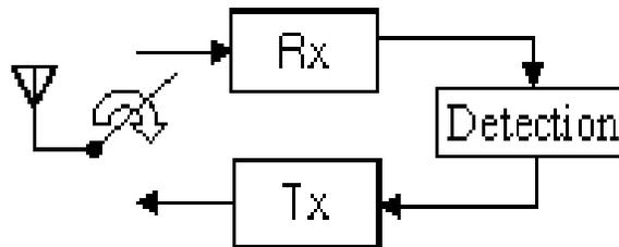
Figure 3.4 Cooperative spatial multiplexing system: relay diagram
