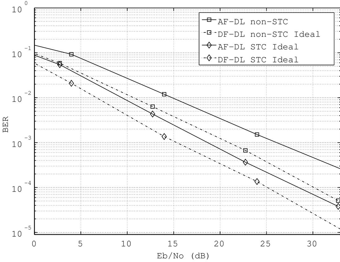
Figure 4.6 BER performance of ideal downlink AF-CSM and DF-CSM systems.
