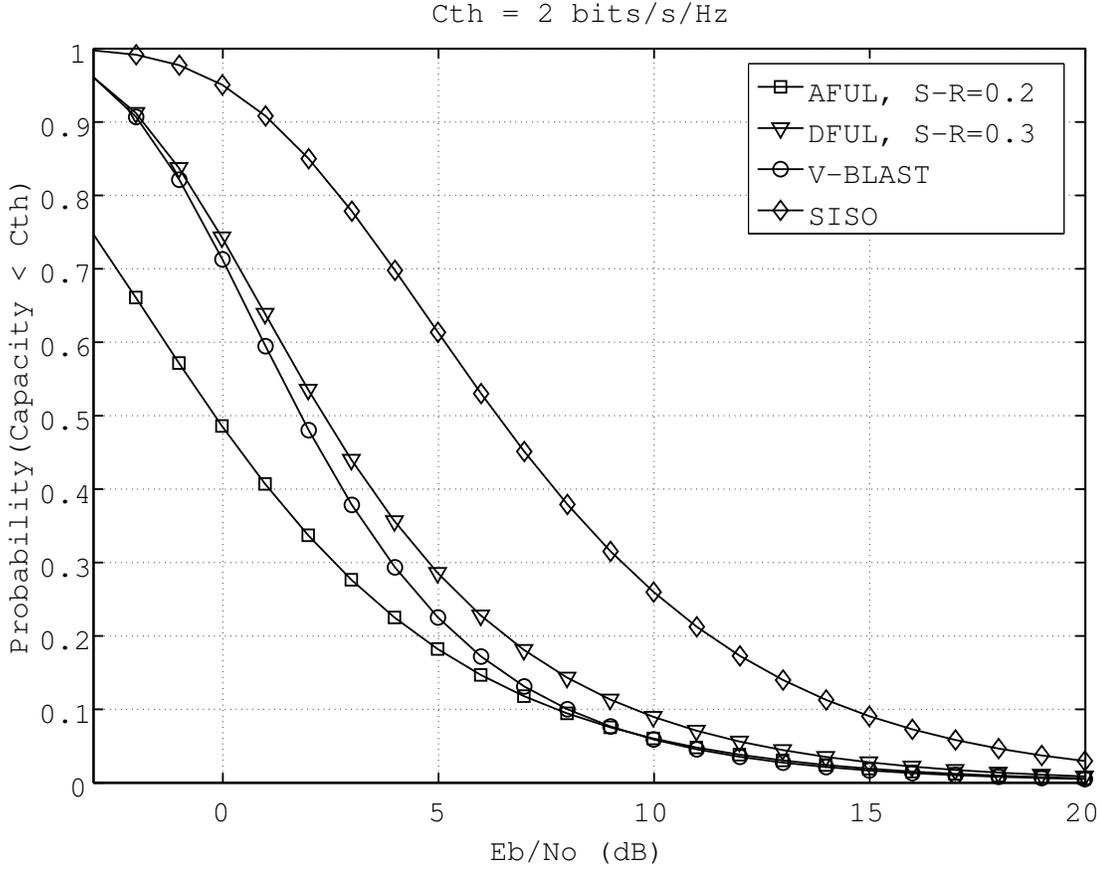
Figure 6.1 Outage capacity of uplink CSM systems,  $c_{th} = 2$  bits/s/Hz.
