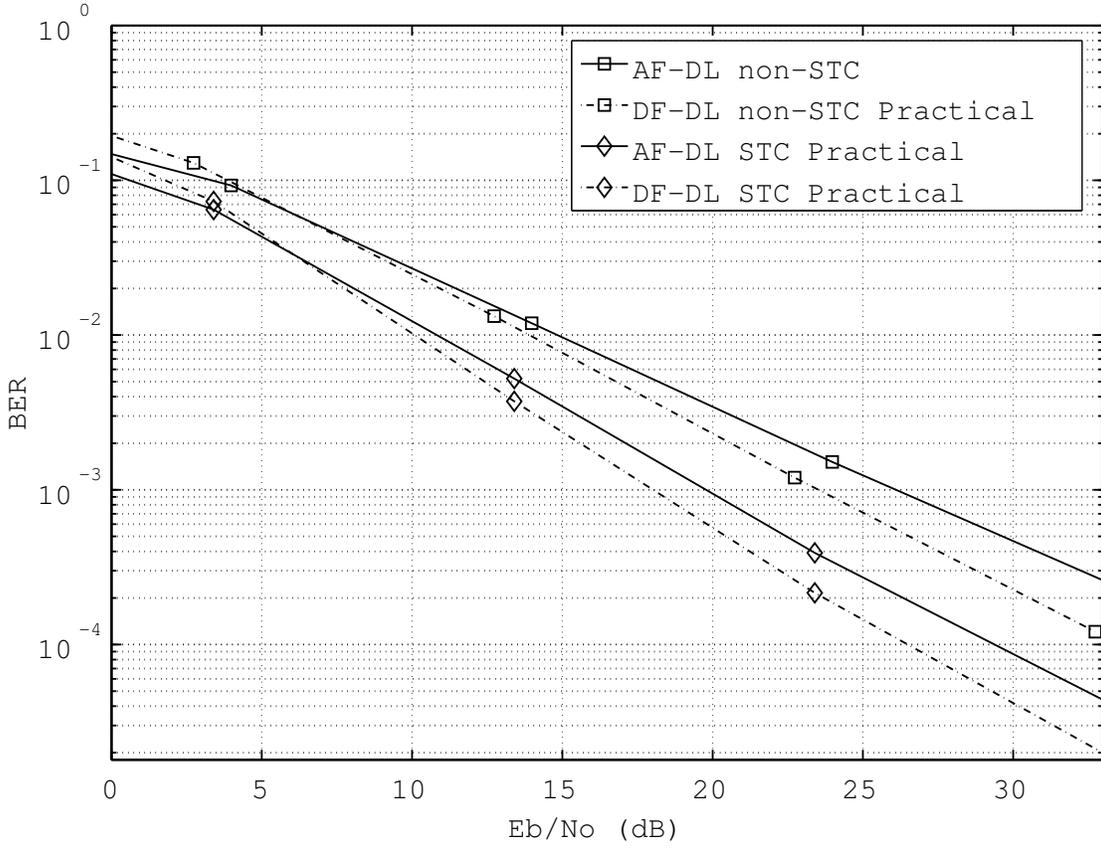
Figure 4.7 BER performance of practical downlink AF-CSM and DF-CSM systems.
