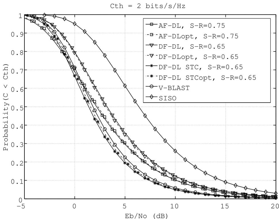
(a) Outage capacity vs.  $E_b/N_0$ ,  $c_{th} = 2 \text{ bits/s/Hz}$
