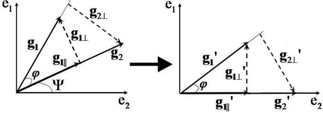
Figure 5.3 Geometrical representation of received vector signal & its rotation for  $M = N = 2$  CSM.
