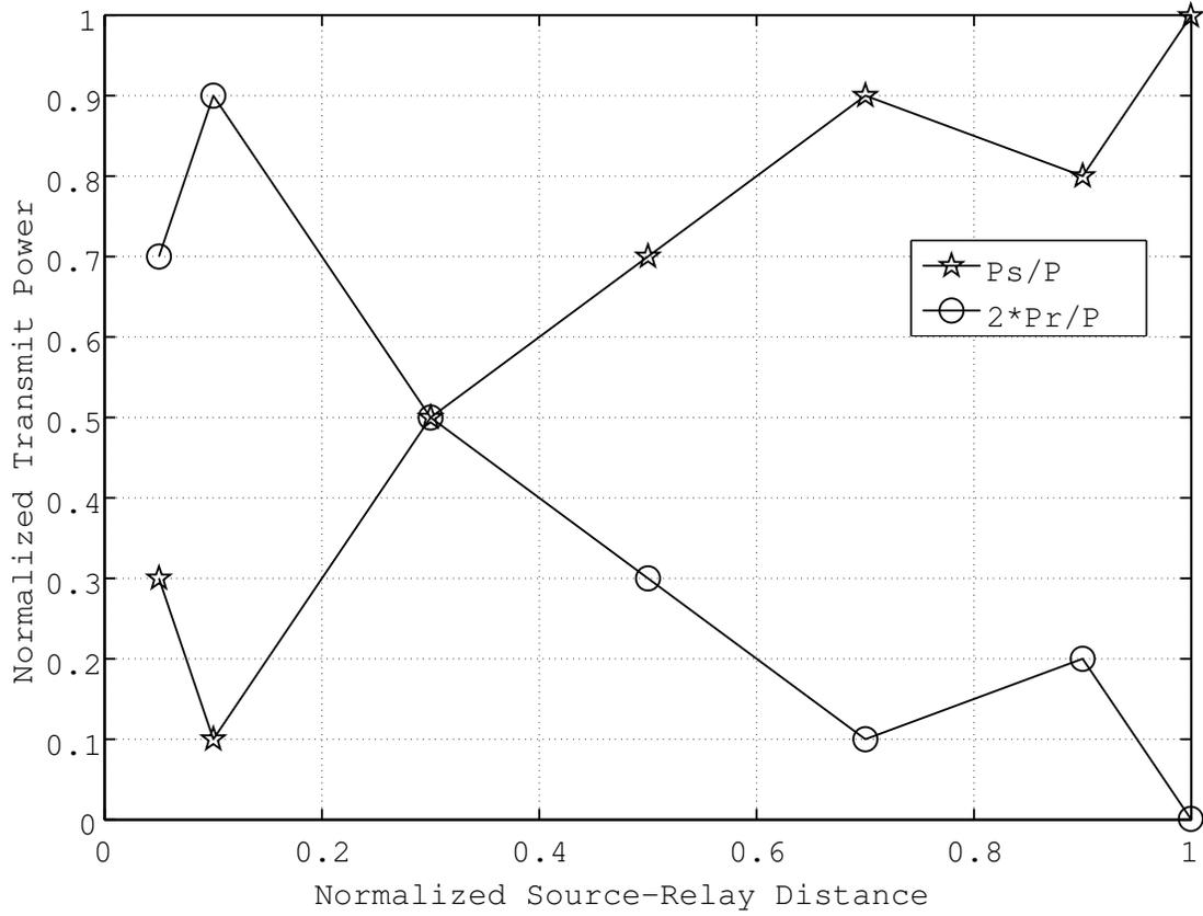
Figure 3.8 Recommended power allocation for AF-CSM, SNR=40 dB.
