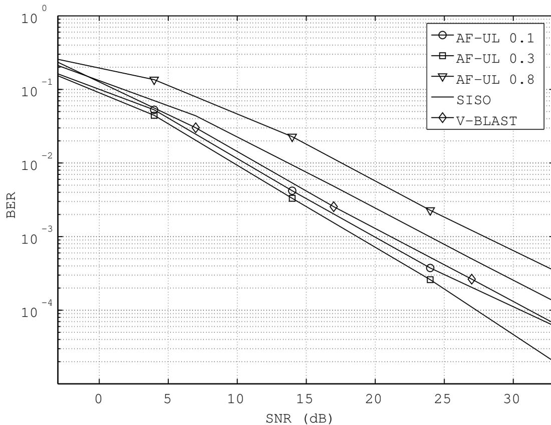
Figure 3.7 BER of AF-CSM with different relay distances & power allocation scheme.
