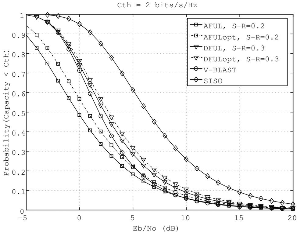
(a) Outage capacity vs.  $E_b/N_0$ ,  $c_{th} = 2 \text{ bits/s/Hz}$
