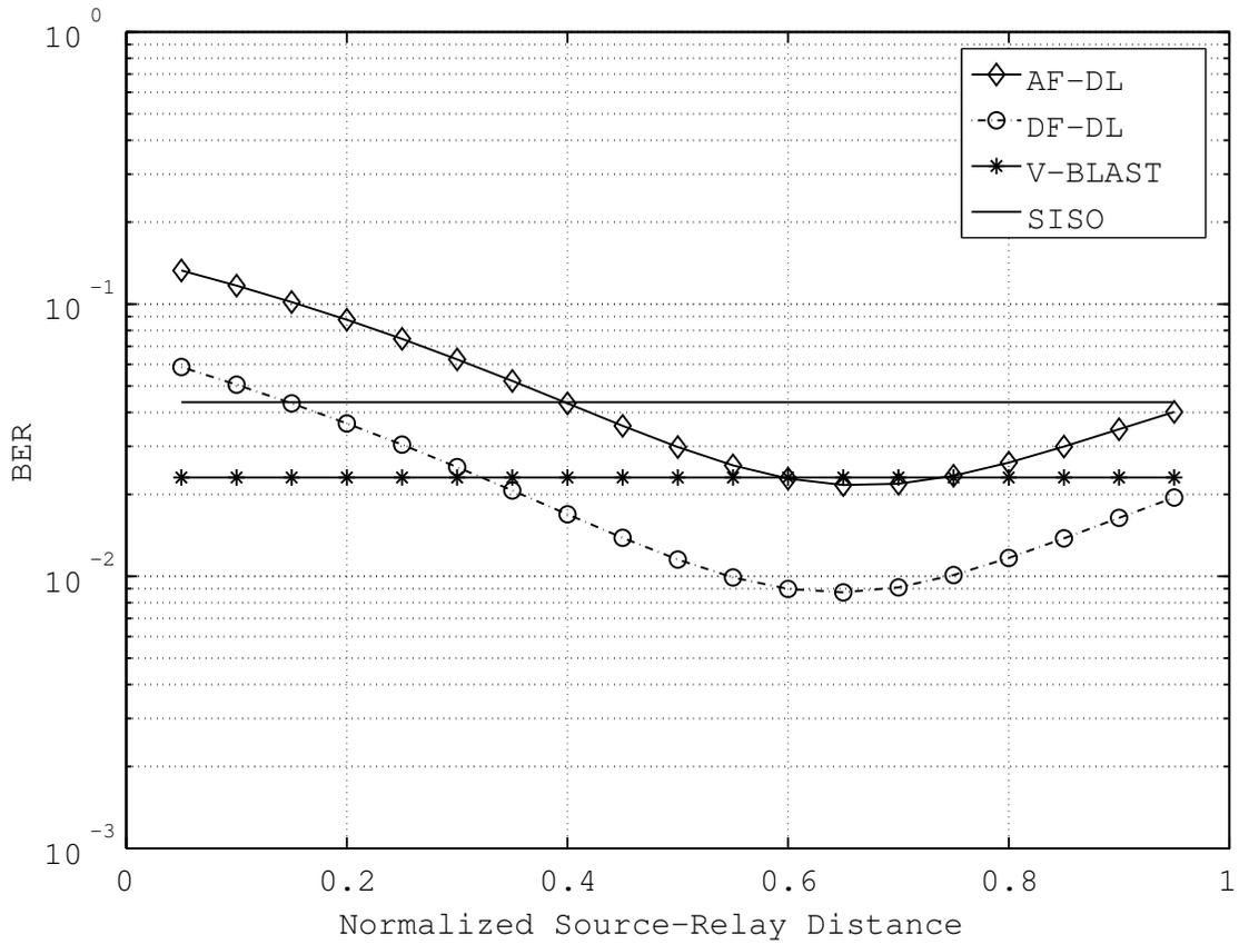
Figure 4.2 BER performance of downlink AF & DF CSM systems for different relay locations,  $E_b/N_0 = 10$  dB.
