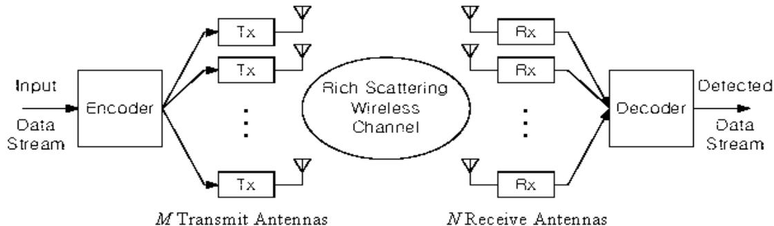
Figure 2.2 V-BLAST system diagram
