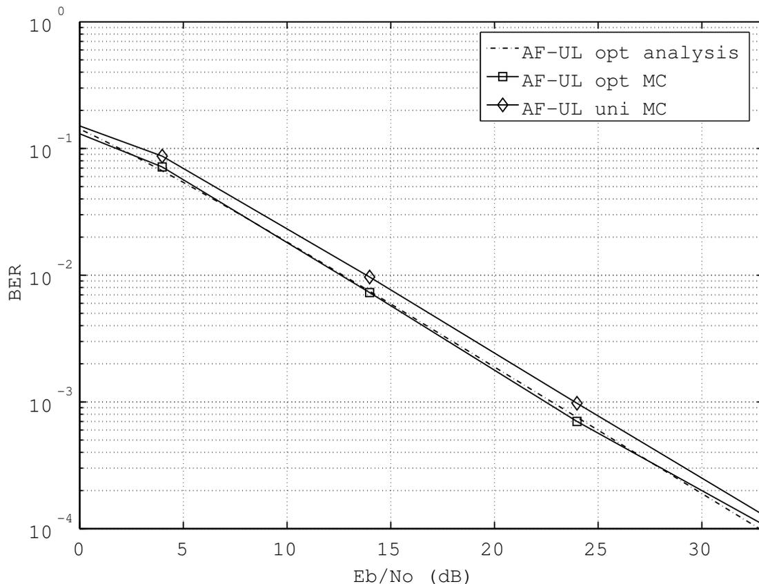
Figure 7.2 BER performance of AF uplink systems with uniform and optimal power allocation schemes.
