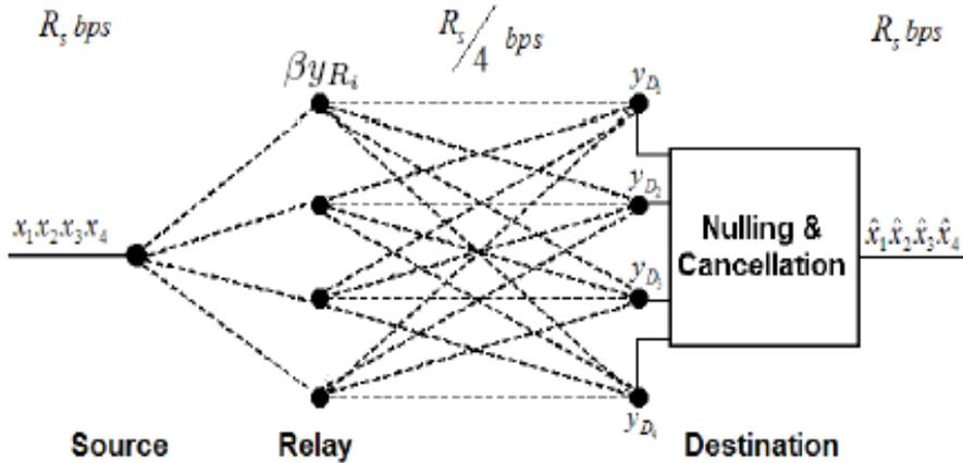
Figure 3.2 Cooperative spatial multiplexing system: Amplify-and-Forward scheme.
