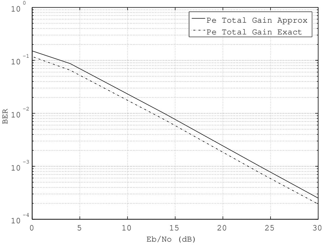
Figure 5.1 Comparison of exact (3.15) and approximate (5.10) relay amplifying factors.
