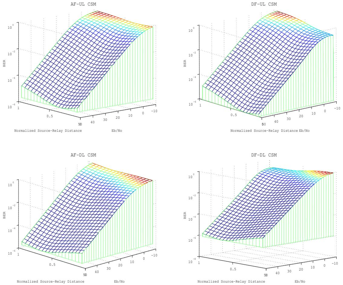
Figure 5.10 Theoretical BER of Downlink AF and DF-CSM, various SNR & source-relay distances.
