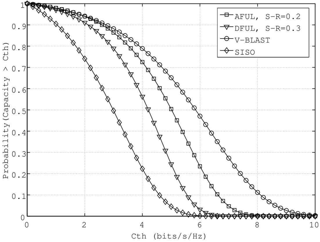
Figure 6.2 Outage capacity of uplink CSM systems,  $E_b/N_0 = 10$  dB.
