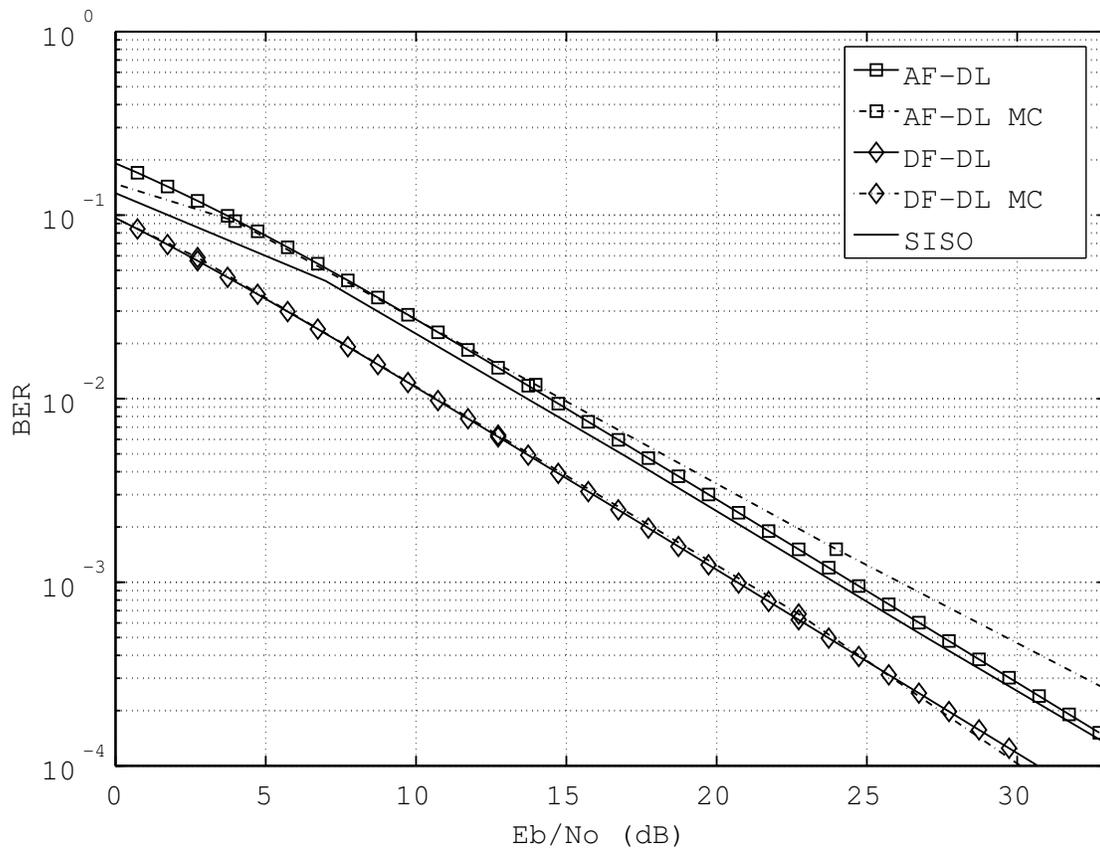
Figure 5.8 Theoretical BER of Downlink AF and DF-CSM.
