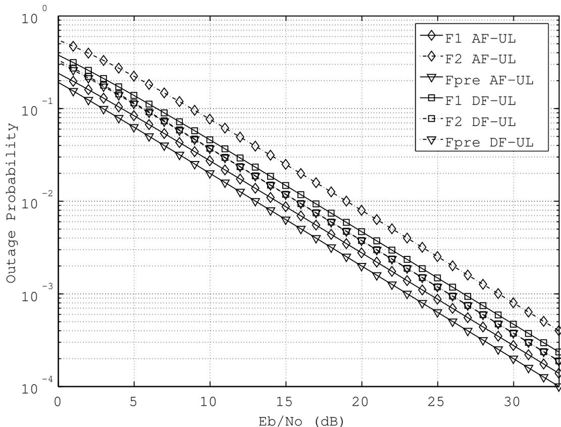
Figure 5.4 Theoretical Outage Probability of Uplink AF and DF-CSM.
