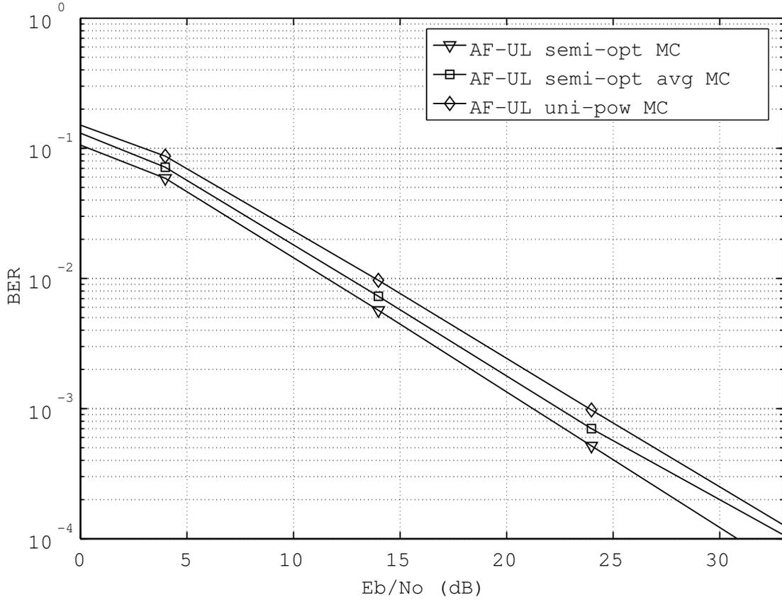
Figure 7.1 BER performance of AF uplink systems with uniform and optimal power allocation schemes.
