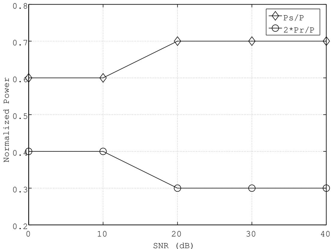
Figure 3.6 Power allocation trend of AF-CSM, source-relay distance = 0.5.
