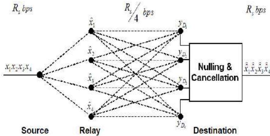
Figure 3.3 Cooperative spatial multiplexing system: Decode-and-Forward scheme.
