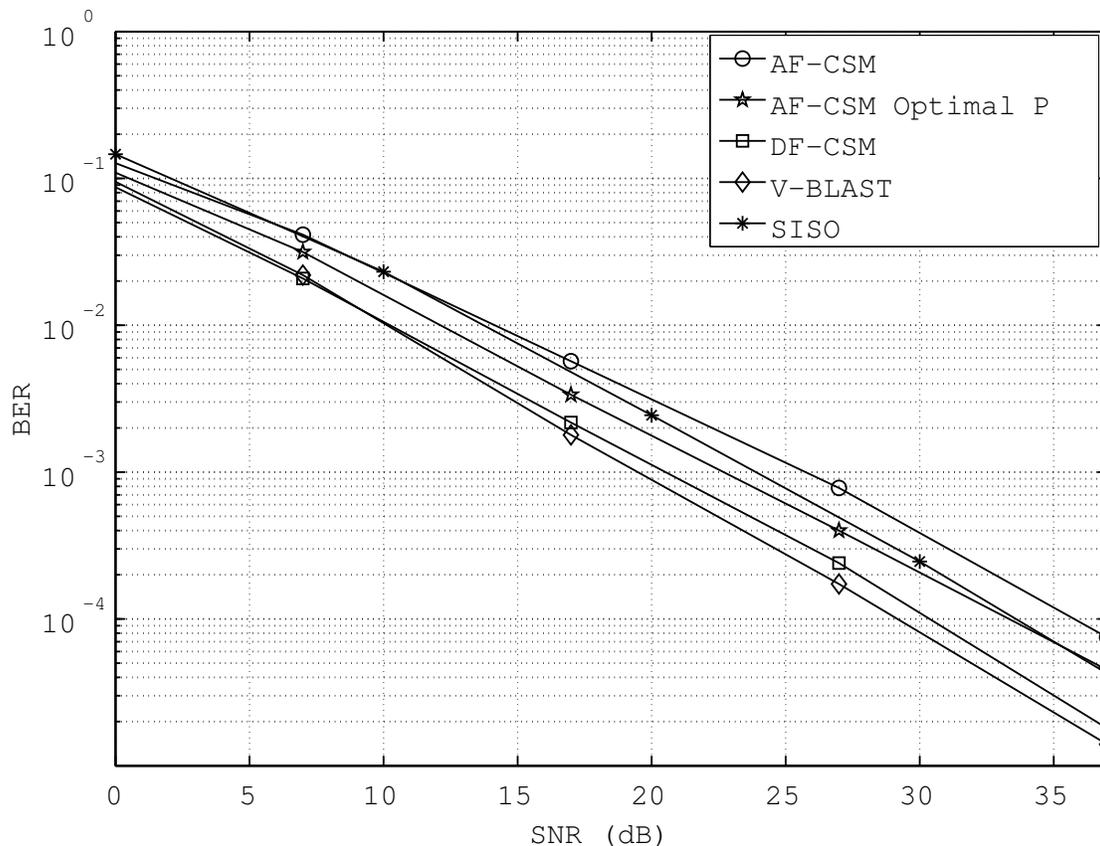
Figure 3.5 BER comparison of AF-CSM system and other systems.
