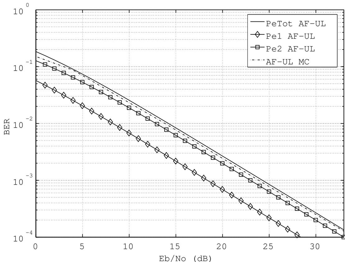
Figure 5.5 Theoretical BER of Uplink AF-CSM.
