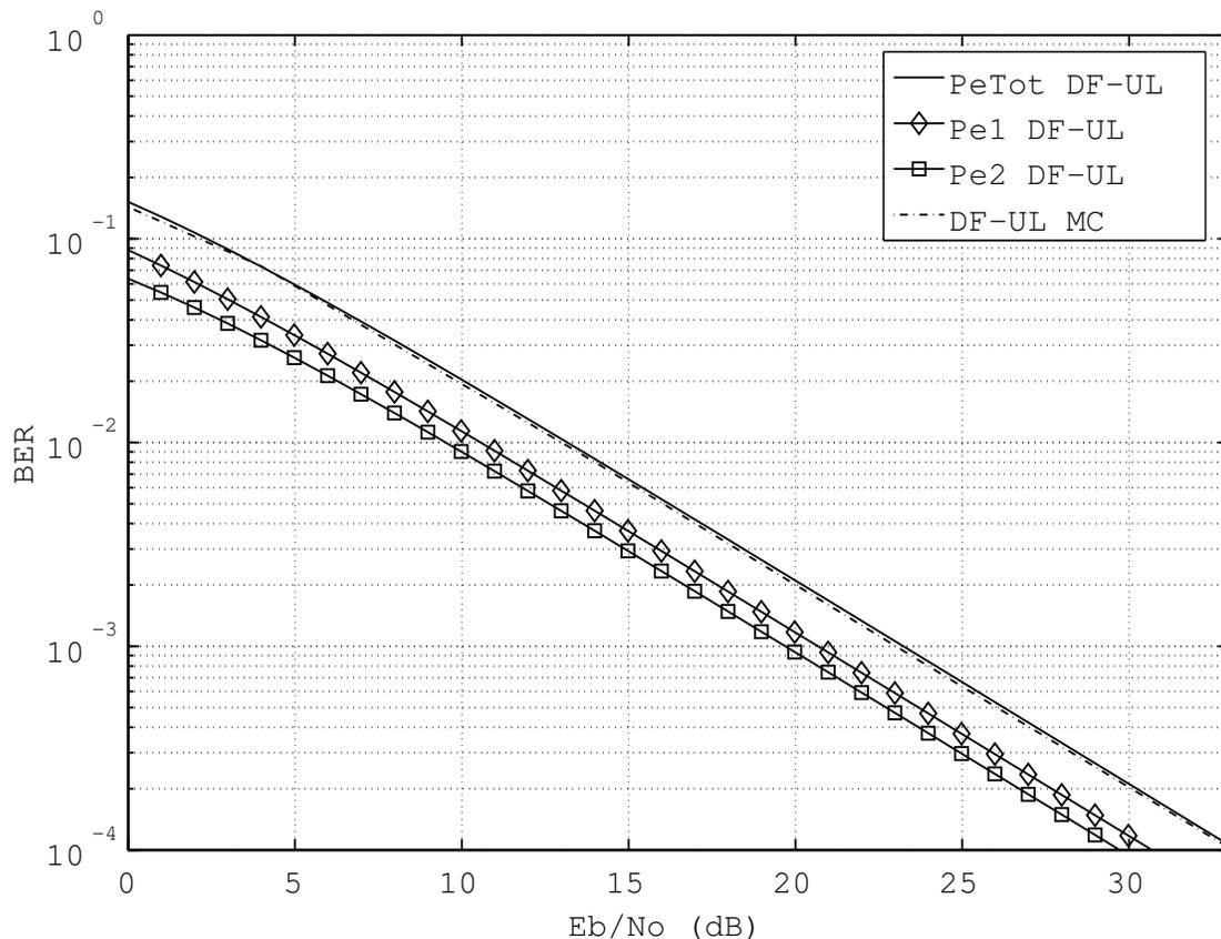
Figure 5.6 Theoretical BER of Uplink DF-CSM.
