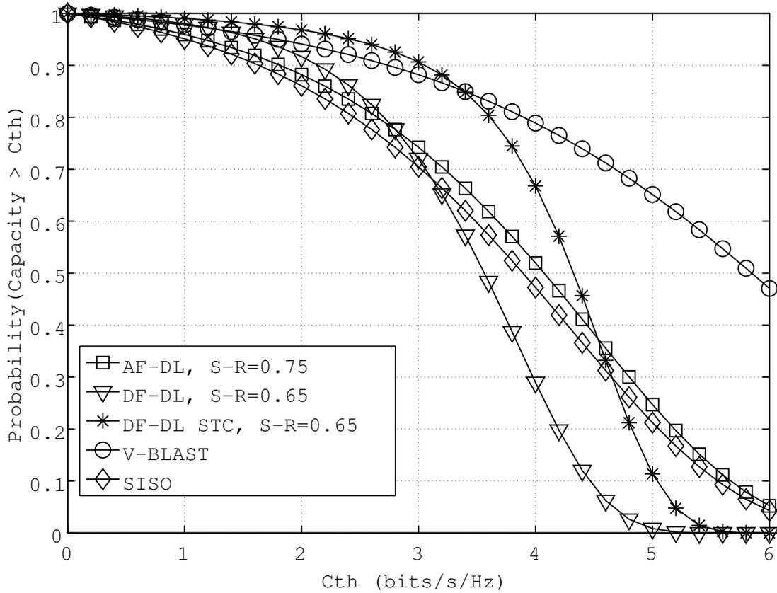
Figure 6.4 Outage capacity of downlink CSM systems,  $E_b/N_0 = 10$  dB.
