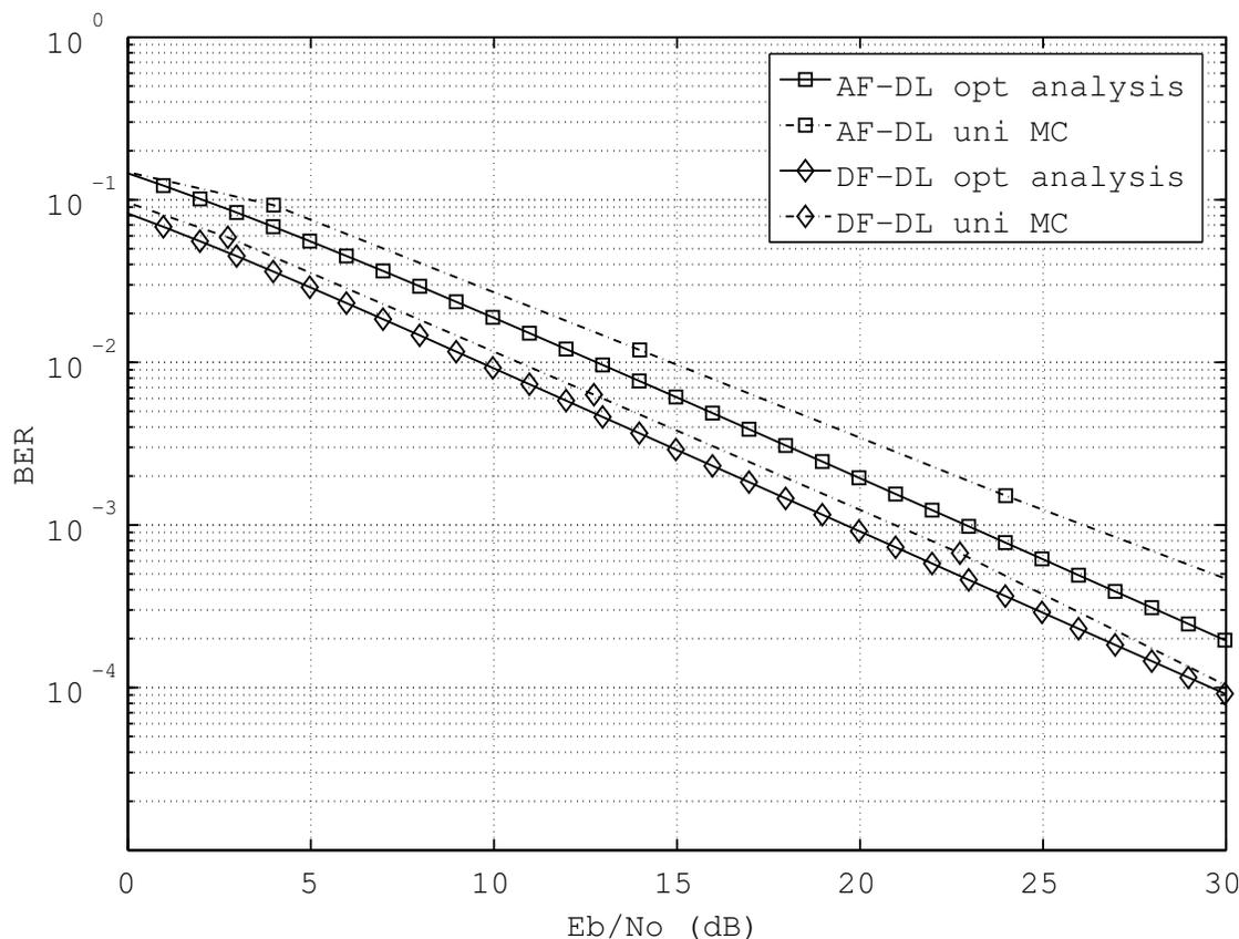
Figure 7.4 BER performance of AF & DF downlink systems with uniform and optimal power allocation schemes.
