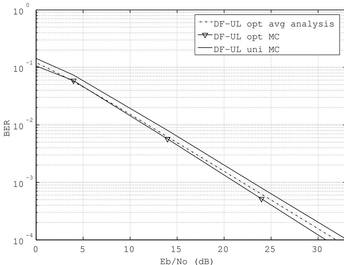
Figure 7.3 BER performance of DF uplink systems with uniform and optimal power allocation schemes.
