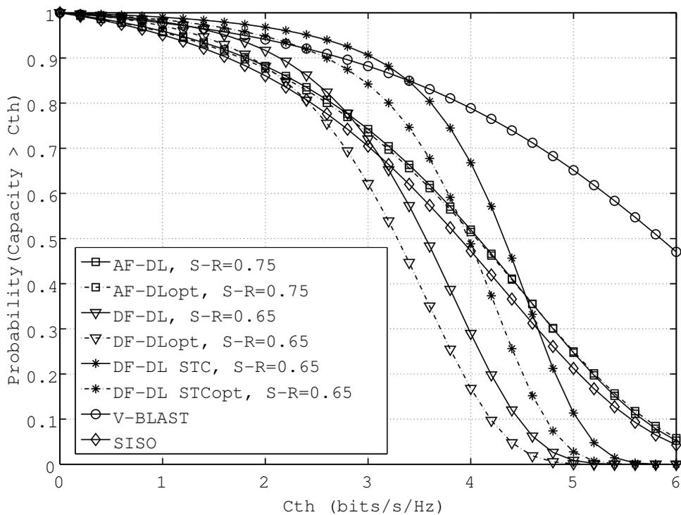
(b) Outage capacity vs.  $c_{th}$ ,  $E_b/N_0 = 10 \text{ dB}$ ,
