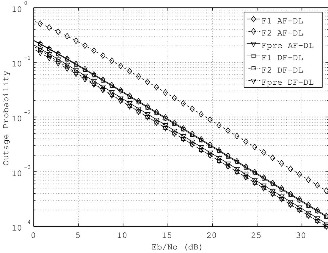
Figure 5.7 Theoretical Outage Probability of Downlink AF and DF-CSM.
