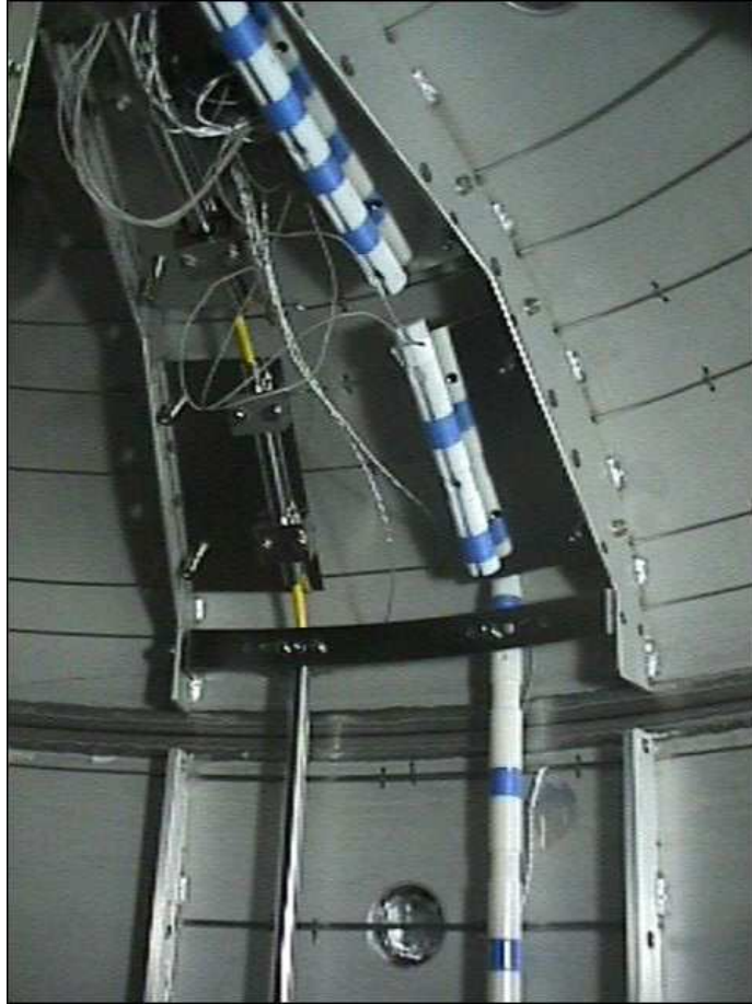
Figure 5.3: A photo of magnetics on the low magnetic field side of the torus (without protection cover). The blue sensors are pickup coils and the yellow ones are I_p rogowski coil. Flux loops covered by the protection stainless steel tubes can also be seen.
