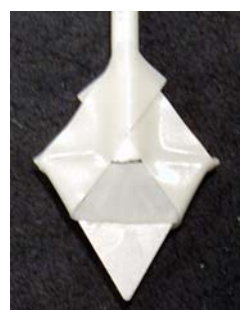
Fig. 5-33 Tool insert masked with tapes
