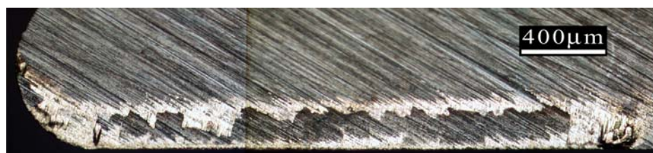
Fig. 5-46 Rake face of non-plated insert after experiment
