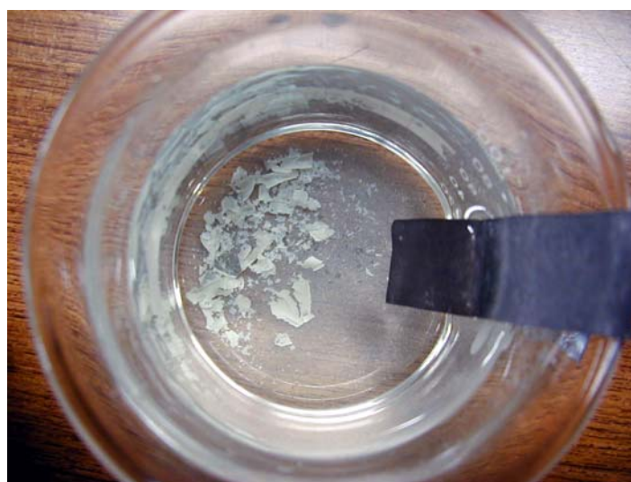
Fig. 5-62 Yellow flakes peeled in 8.8% condition
