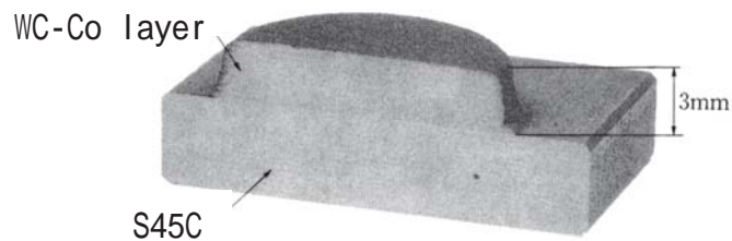
Fig. 5-11 WC-Co layer on S45C steel 5-8)
