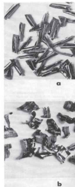
Fig. 4-3 Chips milled by Ti alloy
