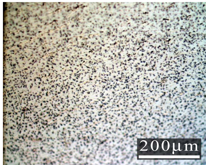
Fig. 5-52 Ni-P-SiC plated surface before the test
