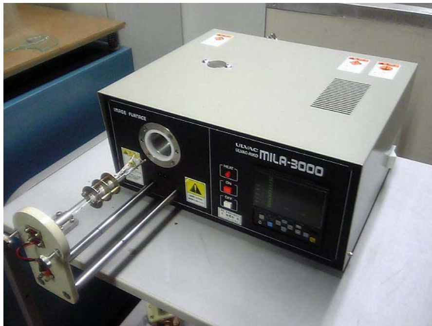
Fig. 6-8 Infrared-type rapid heating furnace (Ulbac MILA-3000)
