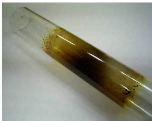
Fig. 6-11 Adhesion of polyimide varnish on inner pipe of furnace
