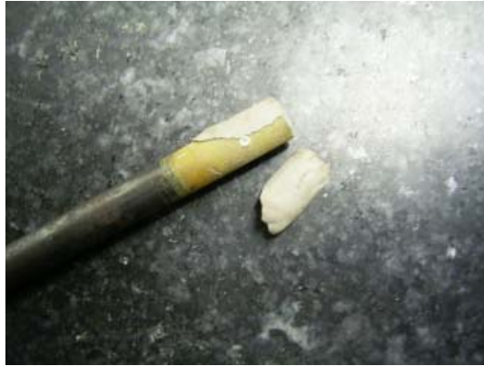
Fig. 6-26 Flaked vitrified abrasive layer in hardness test of layer
