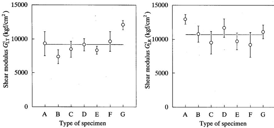
Fig. 2. Shear moduli obtained from the accurate solution,  $G_{LT}^i$  and  $G_{LR}^i$ , corresponding to the type of the specimens.
