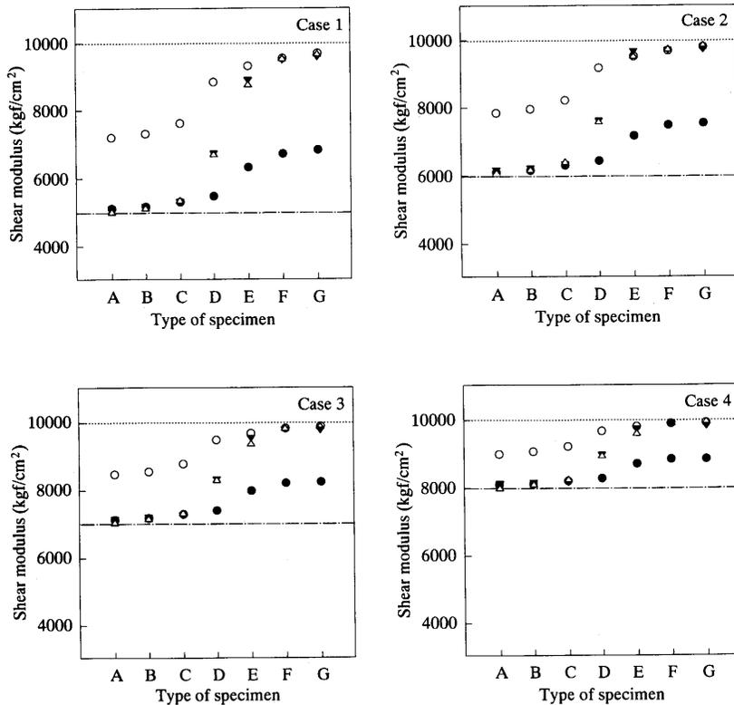
Fig. 4. Shear moduli calculated by the quasi-isotropic solutions.
