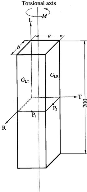
Fig. 1. Diagram of the rectangular bar subjected to the torsional force.
