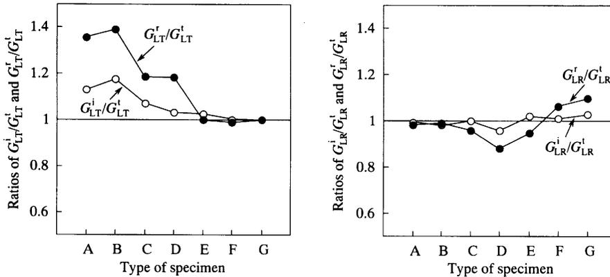
Fig. 3. Ratios of the shear moduli obtained by the approximated methods to those by the accurate solution.
