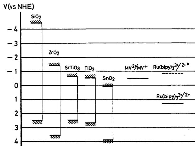
Figure 6. Band energies of oxides at pH 7 and redox potentials of methylviologen and  $\text{Ru}(\text{bpy})_3\text{Cl}_2$ : (—) redox potential for ground state; (---) redox potential for excited state. See text and ref 8-11.
