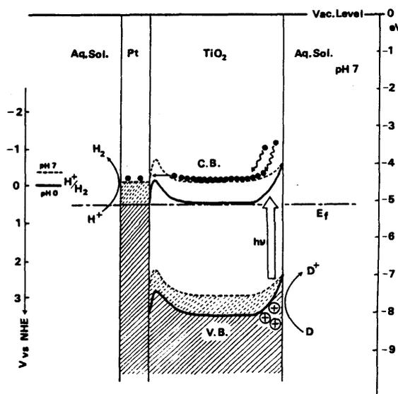
Fig. 1. The energy structure of the photocatalyst,  $\text{TiO}_2/\text{Pt}$ , in an electrolyte solution ( $\text{pH} = 7$ ). The barrier height at the metal-semiconductor interface is modified by the image force of the metal. The solid lines show the energy levels in the dark and the dotted lines those under illumination.
