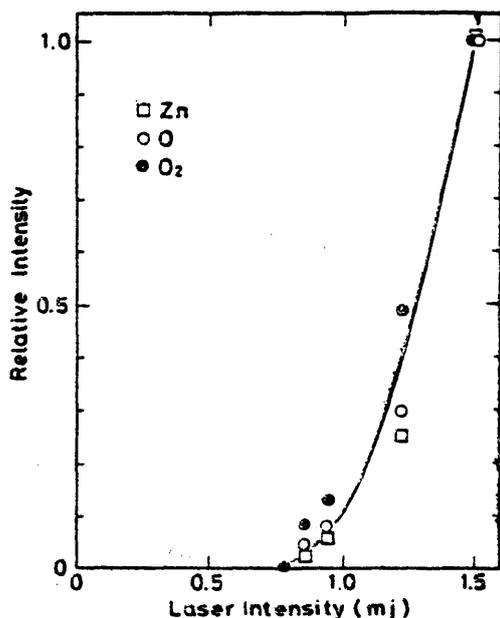
FIGURE 1, Laser intensity dependence of the relative neutral particle emission yield measured at room temperature.
