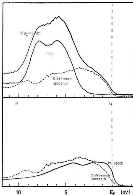
Fig. 3 X-ray photoelectron spectra of  $\text{TiO}_2$  and  $\text{TiO}_2/\text{Pt}$  (5%) in the valence band region
