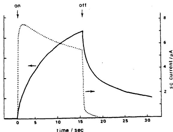
**Figure 6.** — Change of photocurrent vs. time. Light electrode potential: 0.4 V vs SCE. Solid curve:  $\langle \text{ZnO} | \text{eosin-Y}, \text{TEOA} | \text{Pt} \rangle$ ,  $\text{pH} = 12.6$ , 518 nm irradiation. Dotted curve  $\langle \text{ZnO} | \text{rose bengal}, \text{EDTA} | \text{Pt} \rangle$ ,  $\text{pH} = 6.0$ , 620 nm irradiation.
