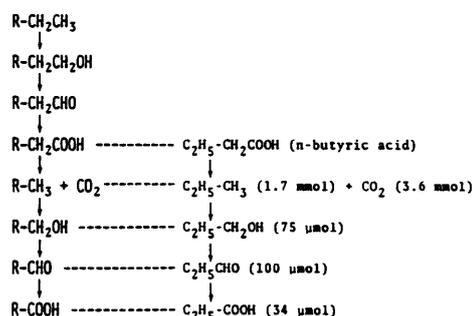
Figure 2. Photocatalytic oxidation process of a linear saturated hydrocarbon and the oxidation products from *n*-butyric acid. Light source: 1-kW Xe lamp. Photocatalyst: TiO<sub>2</sub> in the presence of AgNO<sub>3</sub>. Irradiation time: 19 h.
