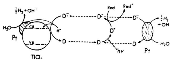
Figure 7. - Schematic illustration of the hydrogen-producing process for halogenated fluorescein derivatives in the presence of a reduction catalyst and a reducing agent.
