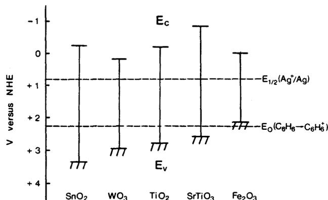
Figure 4. Band edge positions of various semiconductors at pH 7 vs. NHE.<sup>27</sup> Half-wave redox potential of Ag<sup>+</sup>/Ag ( $E_{1/2}$ ) and the potential where the oxidation of benzene occurs ( $E_0$ ) are also illustrated (see the text).
