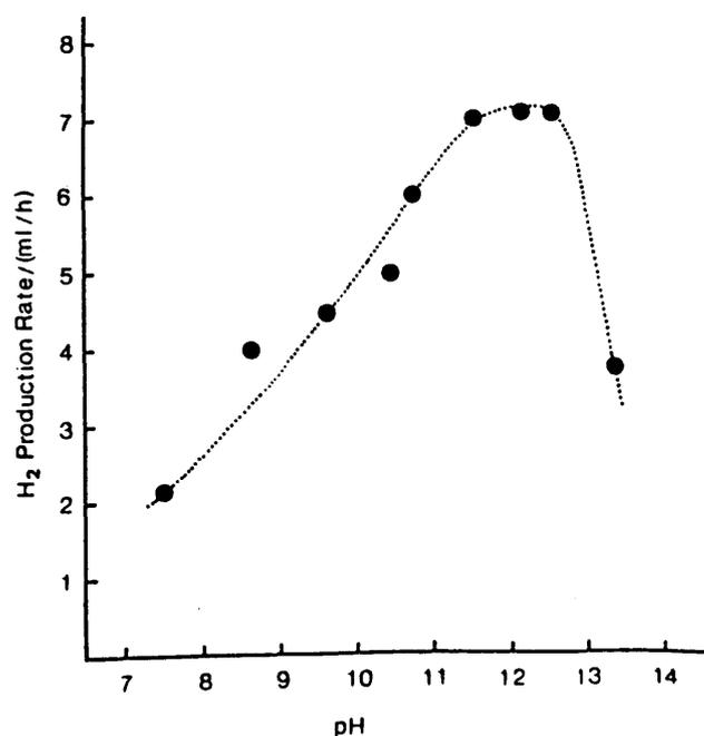
Figure 2. - pH dependence of the initial rate of hydrogen production. FIBr<sub>2</sub>:  $5 \times 10^{-3}$  M, Pt/TiO<sub>2</sub>, TEOA:  $5 \times 10^{-1}$  M.
