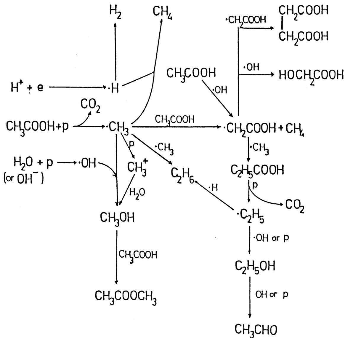
**Figure 2.** Reaction scheme of photocatalytic reactions of acetic acid in aqueous medium with powdered  $TiO_2$  photocatalysts.
