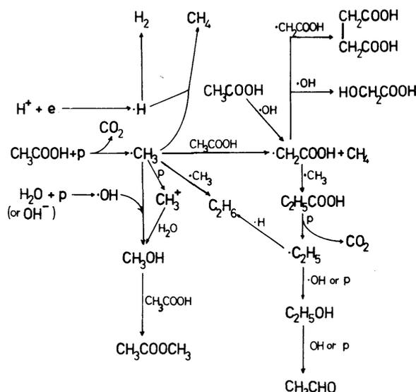
Figure 2. Reaction scheme of photocatalytic reactions of acetic acid in aqueous medium with powdered  $\text{TiO}_2$  photocatalysts.
