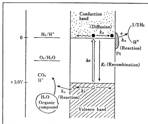
Fig. 6 Energy diagram of  $\text{TiO}_2/\text{Pt}$  particle on which the oxidation of water and organic substance and the hydrogen production proceed
