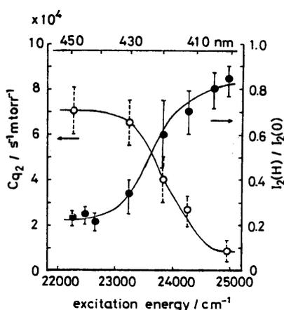
Fig. 2. Plots of  $I_2(H)/I_2(0)$  (●) and the self-quenching constant,  $C_q$  for  $F_2$  (○) versus excitation energy in the presence of a magnetic field of 3.5 kG.
