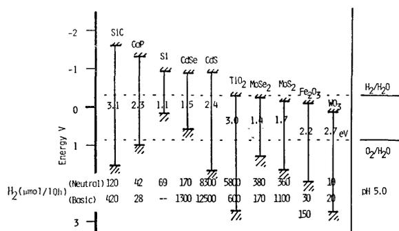
Fig. 1 The rate of  $\text{H}_2$  production from water-ethanol mixture with various platinized semiconductor particles by the irradiation with 500 W Xe lamp
