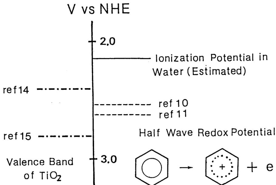
Figure 4. Valence band position of  $\text{TiO}_2$ ,<sup>14 15</sup> half-wave redox potential of benzene in acetonitrile<sup>10 11</sup> and estimated ionization potential of benzene in water. pH = 7.0, vs NHE<sup>26</sup>.
