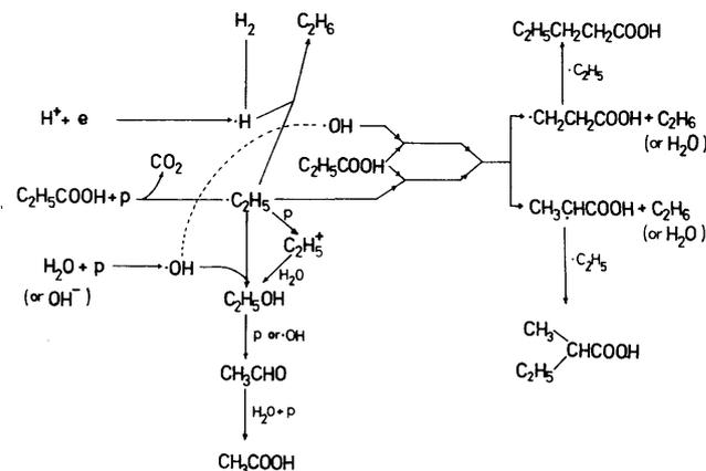
Figure 3. Reaction scheme of photocatalytic reactions of propionic acid in aqueous medium with powdered  $\text{TiO}_2$  photocatalysts.
