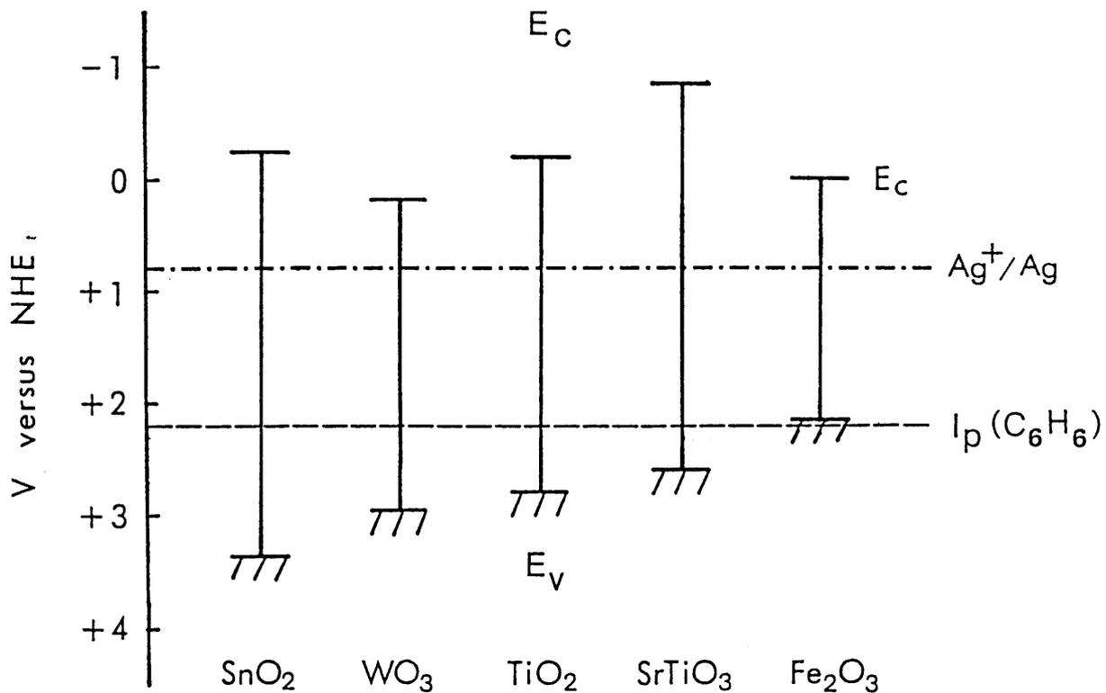
Figure 6. Band edge positions of various semiconductors at pH = 7 vs NHE. Redox potential of  $\text{Ag}^+$  and estimated ionization potential of benzene in water are also illustrated.
