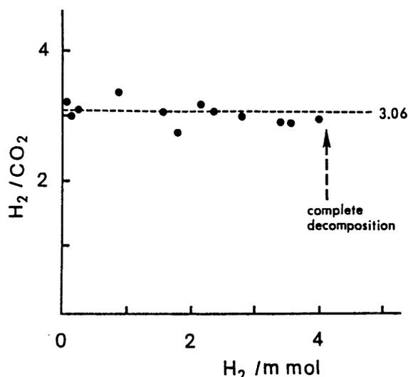
Figure 1. Ratio of hydrogen to carbon dioxide produced during the complete decomposition of *n*-hexadecane (C<sub>16</sub>H<sub>34</sub>). Light source: 1-kW Xe lamp. Photocatalyst: Pt/TiO<sub>2</sub>. Total irradiation time: ~700 h.
