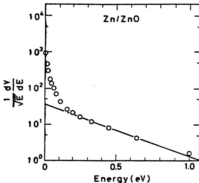
FIGURE 2, The energy spectrum of neutral zinc atoms emitted from ZnO at 210°C. The abscissa is energy  $E$  and the ordinate is the differential emission yield  $dY/dE$ , divided by  $\sqrt{E}$ .
