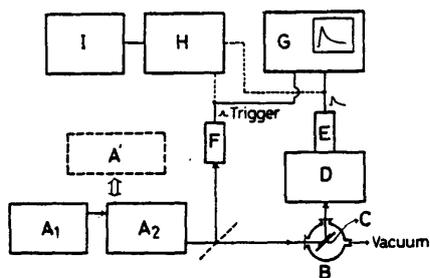
Figure 1. Schematic diagram of experimental apparatus: (A<sub>1</sub>) N<sub>2</sub> laser, (A<sub>2</sub>) dye laser, (A') YAG laser, (B) cryostat, (C) sample, (D) monochromator, (E) photomultiplier, (F) biplanar phototube, (G) oscilloscope, (H) boxcar integrator, (I) recorder.
