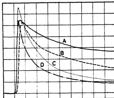
Figure 2. Phosphorescence decay curves of Ru(bpy)<sub>3</sub>Cl<sub>2</sub> adsorbed on various oxide powders. Dye laser excitation, 6 ns, 450 nm. Observed at 620 nm, at 25 °C and under vacuum of 10<sup>-3</sup> mmHg: (A) SiO<sub>2</sub>, (B) ZrO<sub>2</sub>, (C) TiO<sub>2</sub>, (D) SrTiO<sub>3</sub>.
