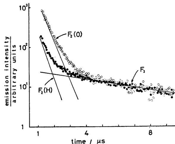
Fig. 1. Semilogarithmic plot of the slow fluorescence intensity (in arbitrary units) of methylglyoxal (22 mTorr) excited at 449.2 nm versus time: o, in the absence of a magnetic field; ●, in the presence of a magnetic field of 1.1 kG.
