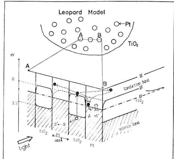
Fig. 4 Schematic model of a  $\text{TiO}_2/\text{Pt}$  particle
