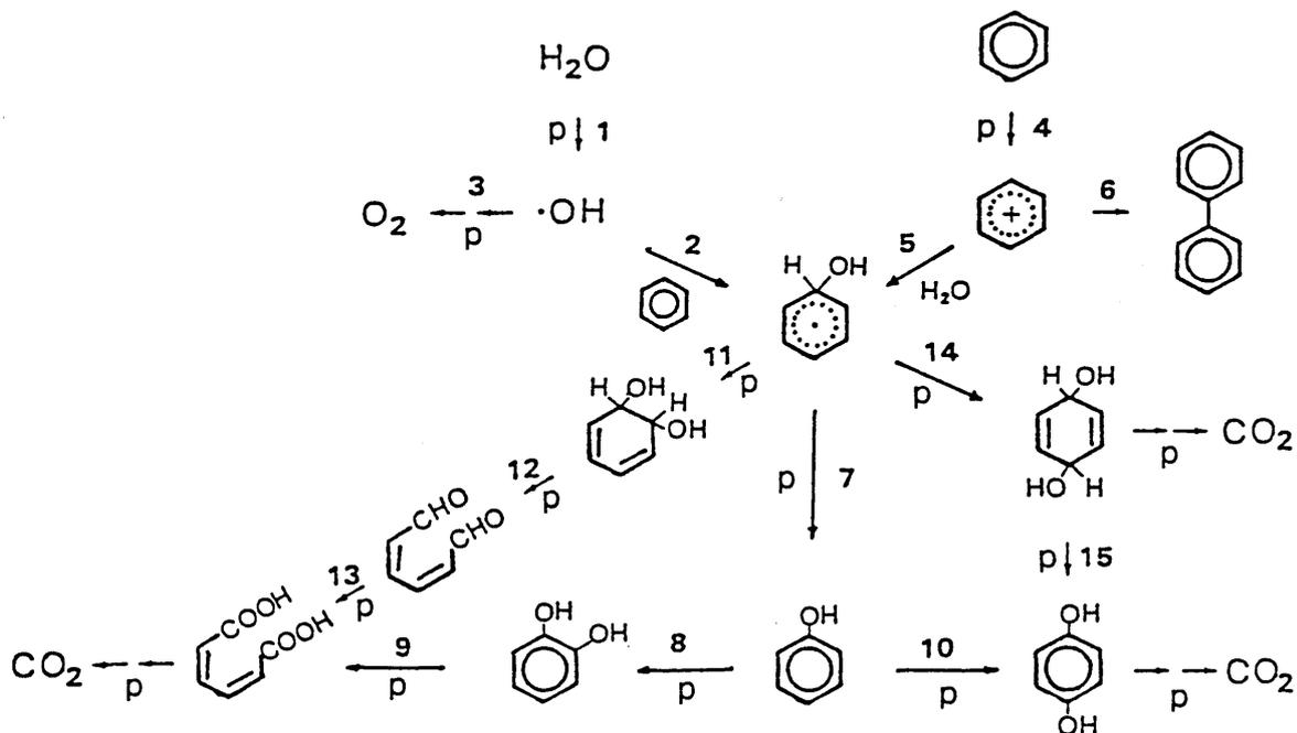
Figure 5. Reaction scheme of photocatalytic oxidation of benzene in water.
