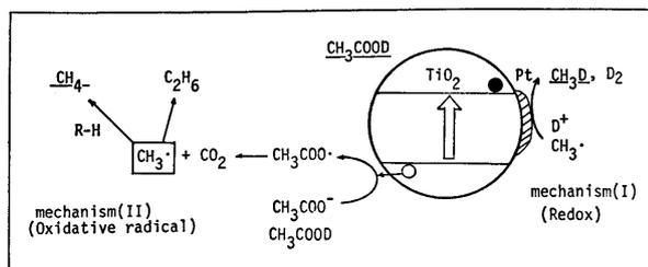
Fig. 5 The two different mechanisms of the decomposition of acetic acid ( $\text{CH}_3\text{COOD}$ ) and the methane formation on a  $\text{TiO}_2/\text{Pt}$  particle
