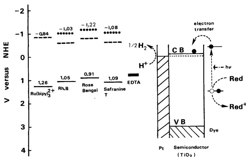
**Figure.** — Schematic mechanism of dye sensitization of semiconductor and the oxidation potentials of the ground state and the first excited state dyes.
