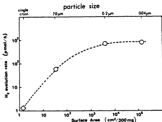
Fig. 3. Dependence of hydrogen evolution on the particle size and surface area of powdered (○) or single-crystalline (◊, 10 mm × 10 mm × 0.8 mm) TiO<sub>2</sub>.
