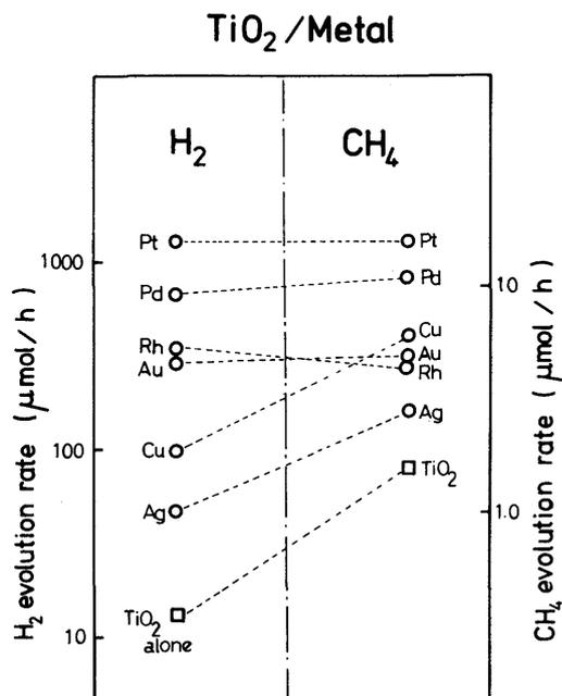
Figure 1. Correlation between hydrogen production rate from an ethanol-water mixture (1:1 in volume) and methane production rate from an acetic acid-water mixture (1:6 in volume) with various  $\text{TiO}_2$  (rutile, doped)/metal photocatalysts; 30 mL of a water-ethanol (or acetic acid) mixture with 300 mg of  $\text{TiO}_2$ /metal photocatalyst was irradiated with a 1-kW Xe lamp (operated at 0.5 kW).
