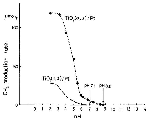
**Figure 4.** Dependence of methane production rate on pH for the photocatalytic decomposition of acetic acid in aqueous medium; 30 mL of a water-acetic acid mixture (6:1 in volume) with 300 mg of  $TiO_2/Pt$  was irradiated with a 500-W Xe lamp. The pH of the mixture, which was controlled by adding NaOH or  $H_2SO_4$ , hardly changed after each experimental run (1-h irradiation).
