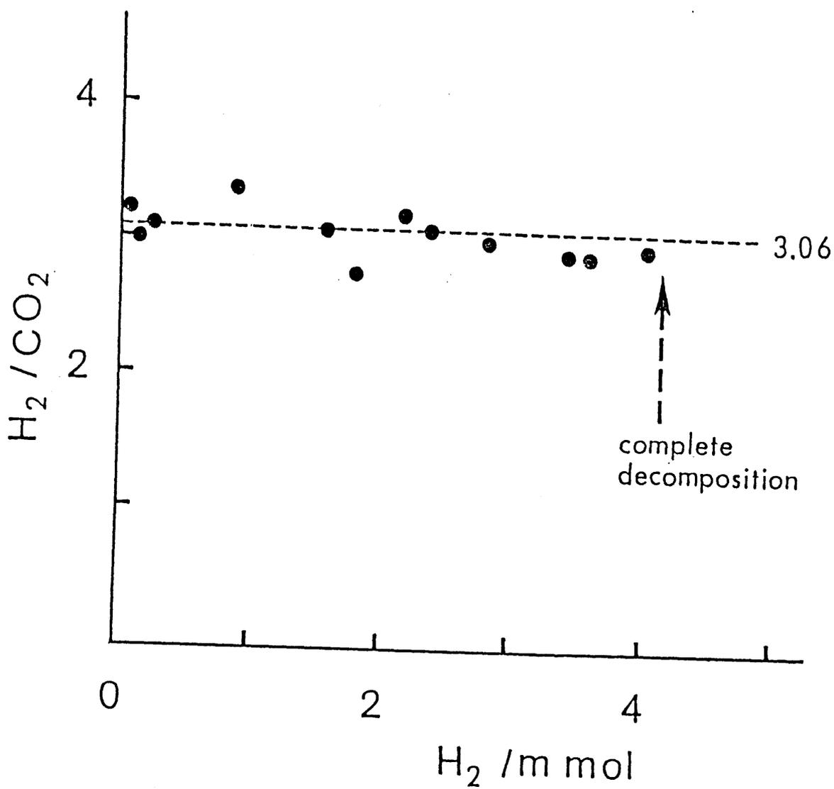
Figure 1. Ratio of hydrogen to carbon dioxide produced during the complete decomposition of n-hexadecane ( $C_{16}H_{34}$ ). Neutral aq. solution, light source: 1 KW Xe lamp, photocatalyst: Pt/TiO<sub>2</sub>, total irradiation time: ~700 hours
