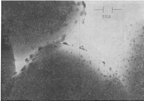
Fig. 2 Electron-micrograph of platinized  $\text{TiO}_2$  (Pt:1 wt%) particle made by photo-electrochemical deposition method
