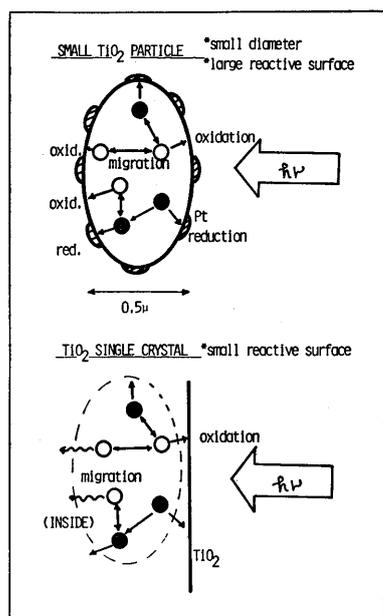
Fig. 7 Schematic representation of small particle of platinized TiO<sub>2</sub> as revealed in this study, and that of bulky TiO<sub>2</sub> single crystal
