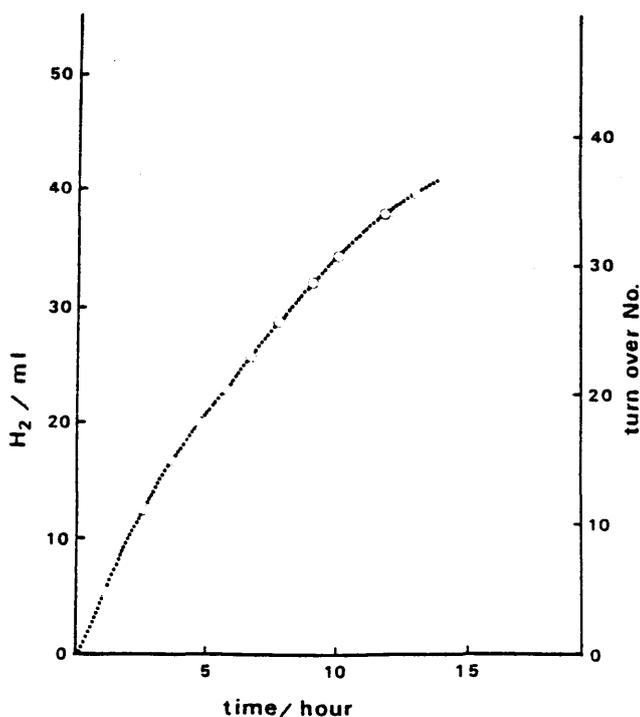
**Figure 3.** — Overall hydrogen production and turn-over number of the dye in Eosin-Y ( $\text{FlBr}_4$ )- $\text{Pt/SiO}_2$ -TEOA system as a function of the visible light illumination time. Light source: 500-W Xe lamp ( $\lambda > 470$  nm).  $\text{FlBr}_4$ :  $5 \times 10^{-3}$  M, TEOA:  $10^{-1}$  M, pH = 12.5 (10 ml aq. soln).
