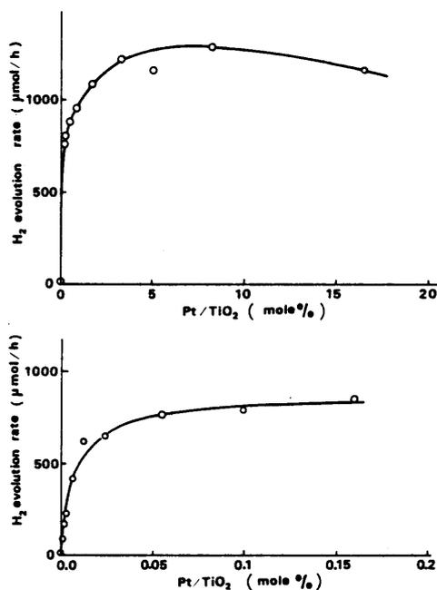
Fig. 2. Dependence of hydrogen evolution rate on the amount of Pt supported photochemically on  $\text{TiO}_2$ . Water: 15 ml, ethanol: 15 ml,  $\text{TiO}_2/\text{Pt}$ : 300 mg, irradiation with a 500 W Xe lamp.
