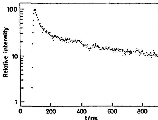
Fig. 3. Decay of Nakarai ZnS. Luminescence at 452 nm (under air at room temp). Light source: Pulsed N<sub>2</sub> laser, 6 ns, 337 nm.
