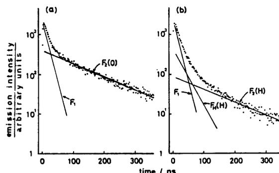
Fig. 3. Semilogarithmic plot of the initial fluorescence intensity (in arbitrary units) of methylglyoxal (100 mTorr) excited at 449.2 nm versus time: (a) in the absence of a magnetic field; (b) in the presence of a magnetic field of 1.1 kG.
