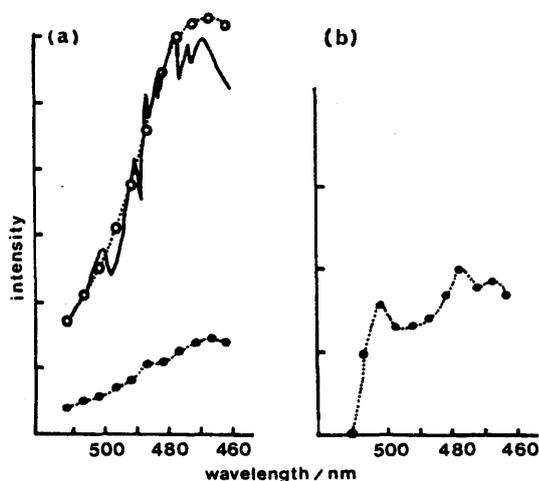
Fig. 4. Emission spectra of methylglyoxal (100 mTorr) excited at 449.2 nm: (a)  $\circ$ , the spectrum of  $F_2$  in the absence of a magnetic field;  $\bullet$ , the spectrum of  $F_2$  in the presence of a magnetic field of 1.1 kG —, the spectrum of  $F_1^h$  in the absence of a magnetic field (from ref. [15]); (b) the spectrum of  $F_3$  (in the absence and in the presence of a magnetic field).
