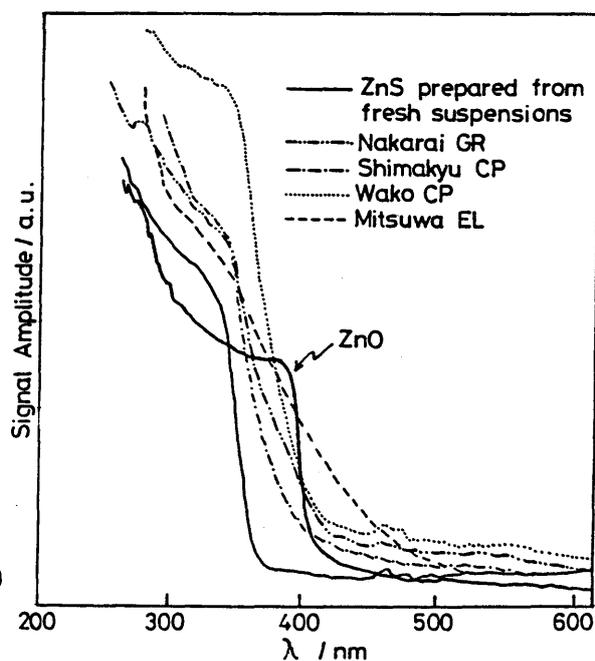
Fig. 2. Photoacoustic spectra of commercial ZnS powders.
