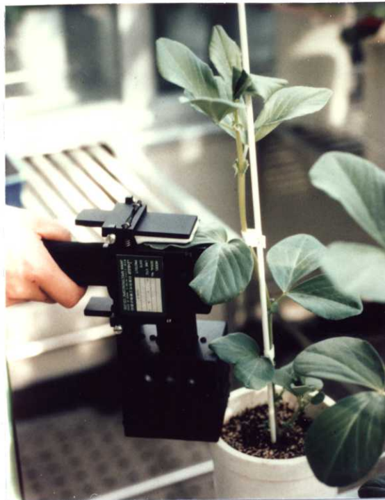
Fig.4.5 Attachment with light source (tungsten halogen lamp) and integrating sphere for measuring reflectance and transmittance of the leaf.
