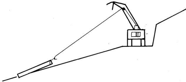
Fig. 3. Ground-skidding system.
