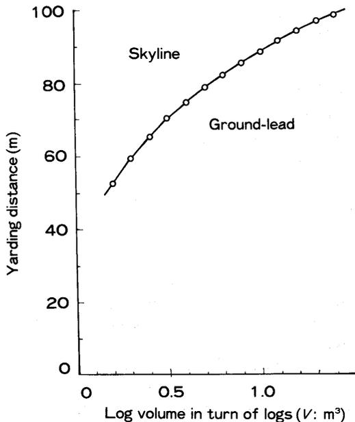
Fig. 9. Break-even points between skyline and ground-lead systems for yarding distance.
