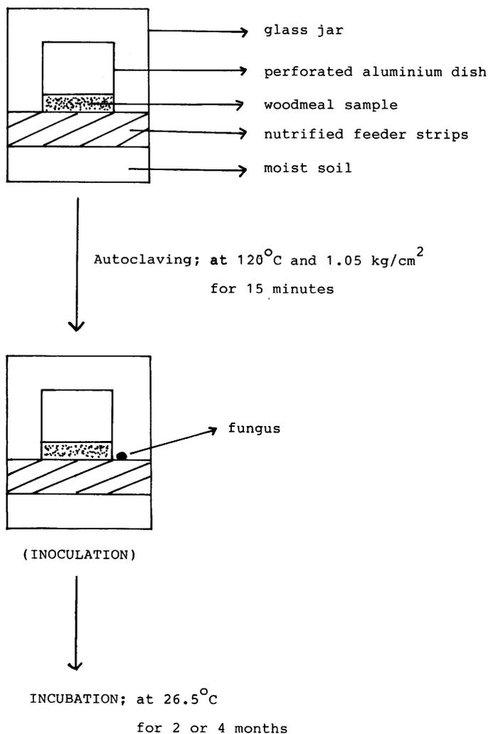
Fig. 1. Chart of wood decay test.
